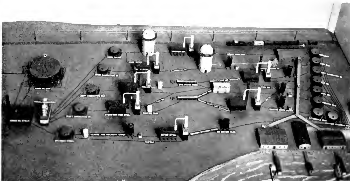
Fig. 4 Model of an Idealized Petroleum Refinery
