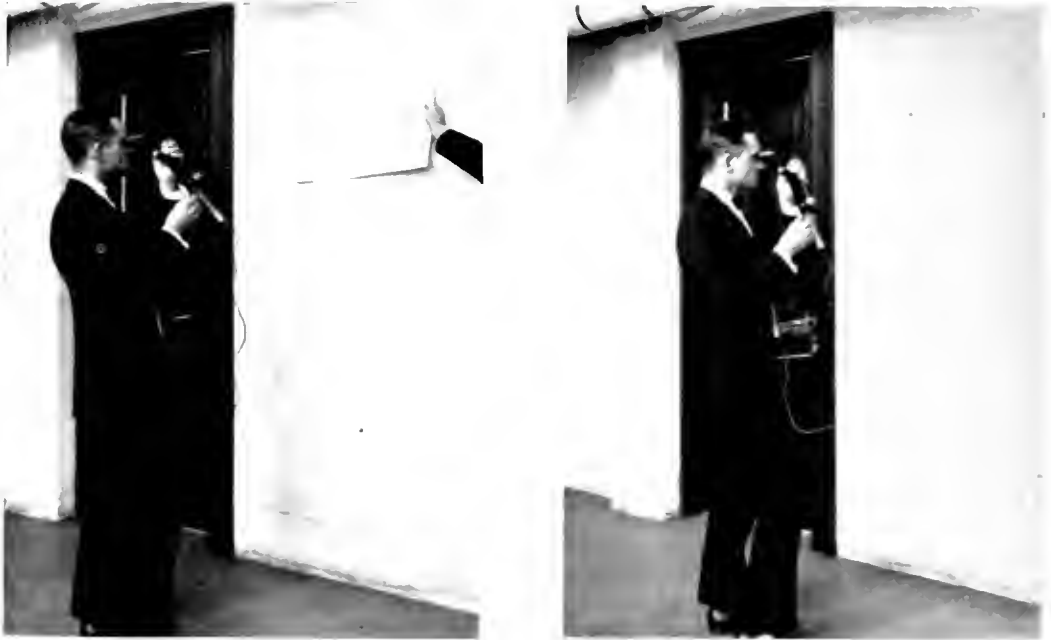
Fig. 1 Determining by Means of Portable Photometer the Reflection Factor of a Wall Surface
