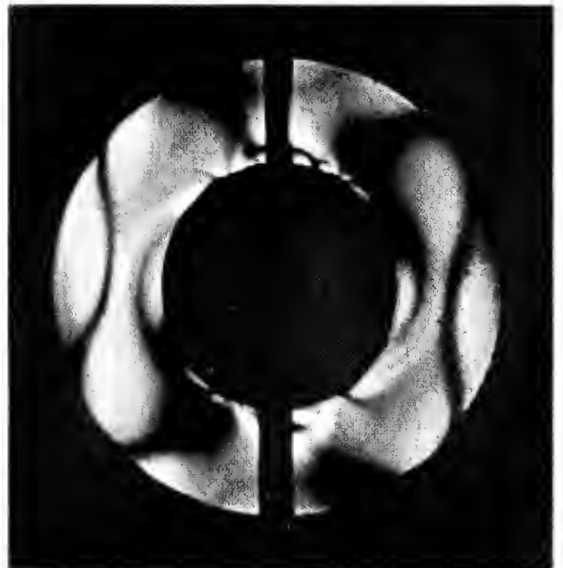
(D) Circular ring in plane polarized light with black band effect.
