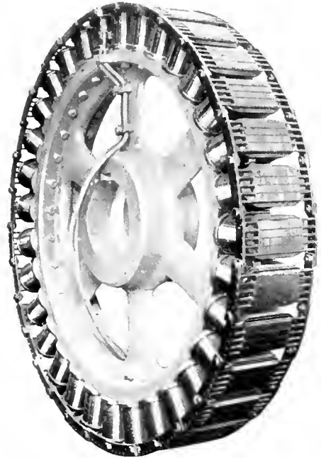
Fig. 7. 32-pole Rotor for Synchronous Motor Showing Construction and Amortisseur Winding
