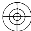
Fig. 17. Direct-current Lamp with Concentric Radiators, the Outer of Which Emits the Light
