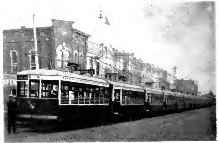
Fig. 19. Light Weight Safety Cars for Eastern Wisconsin Electric Co., equipped with GE-258 motors and K-63 control
