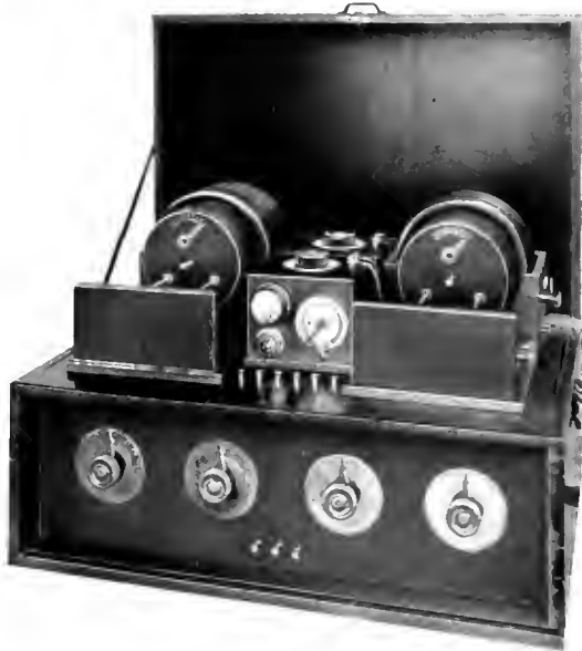
Fig. 29. Radio Receiving Set with Barrage Section
