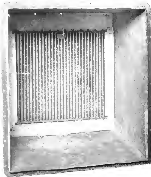
Fig. 2. One of the Radiator Sections in the Air Tunnel Surrounded by Baffles. Baffles at front and sides of section not seen
