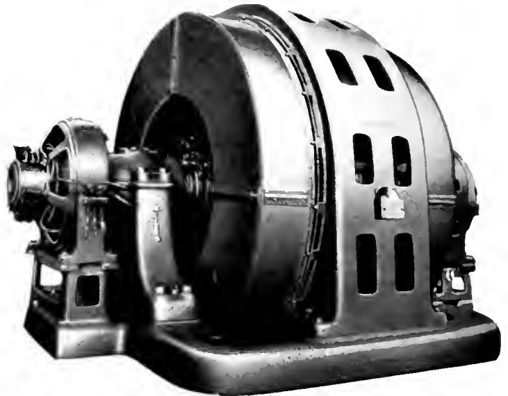
Fig. 12. A 6500 kv-a., 6300-volt, 750 r.p.m. Condenser, having a direct-connected exciter at the near end and a starting induction motor at the far end
