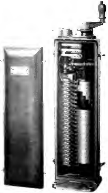
Fig. 10. Type of Master Controller Used in Pilot House and Engine Room
