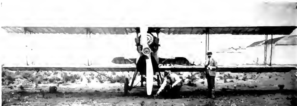
Fig. 15. Biplane Equipped with a G-E Supercharger which can be seen back of the upper blade of the propeller
