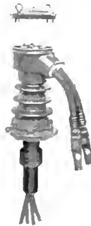
Fig. 54. 25,000-volt Current Transformer Bushing of 400/800 Ampere Capacity with Cover Raised to Show Series-multiple Connection Board
