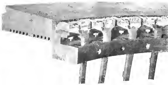
Fig. 4. Detail View of Section of Armature, Alexanderson 200-kw. Radio Frequency Alternator
