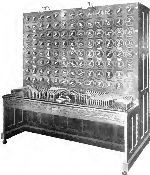
Fig. 1. Short-circuit Calculating Table with Set-up of System Shown in Diagram, Fig. 3
