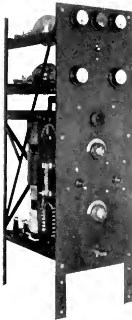
Fig. 7. Plotron Panel for 50,000 Cycles
