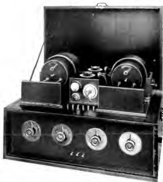
Fig. 9. Barrage Receiving Set Assembled in Carrying Case
