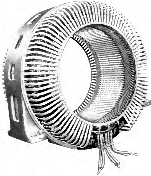
Fig. 5. Stator of a 1400 kv-a. Synchronous Motor Showing the Construction of the Cold Rolled Steel Spot-welded End Shield
