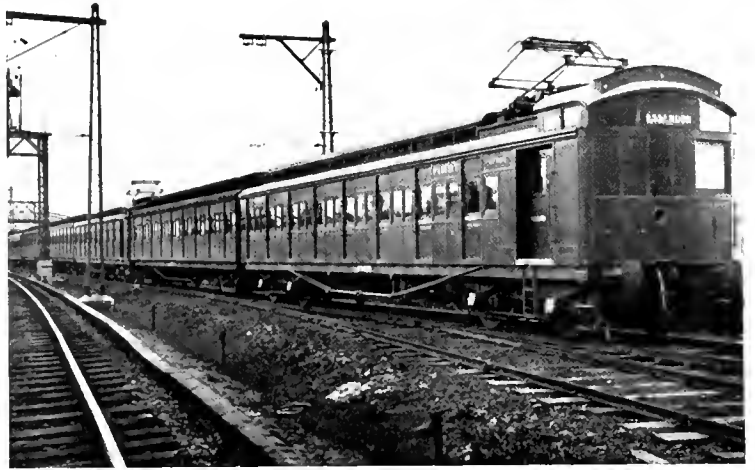
Fig. 17. 1500-volt Direct Current Multiple Unit Train on Victorian Railway, Melbourne, Australia
