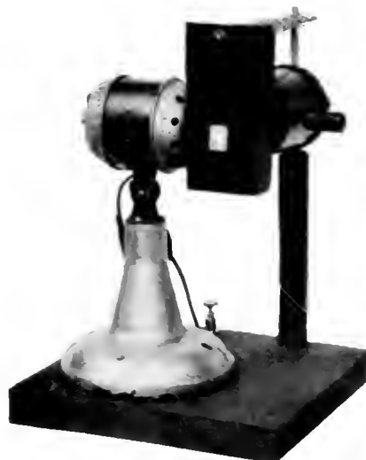
Fig. 2. Front View of Phosphoscope with Shield in Place showing the Observation Window
