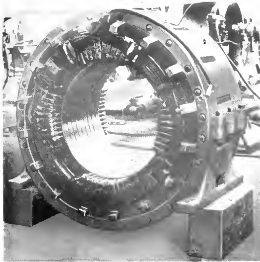
Fig. 21. Armature of 50-cycle, Single-phase, 500-kw., 3000-r.p.m. Turbo-generator Built in 1896
