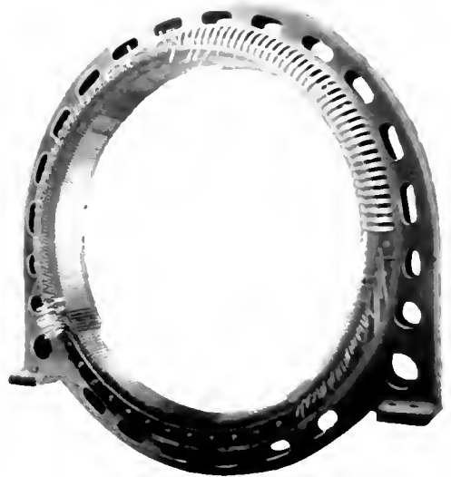
Fig 10 Cored Box Type Stator Frame Used for the Larger Machines
