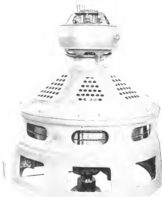
Fig. 1 Vertical Alternating-current Generator with Exciter Arranged for Direct Coupling to a Waterwheel
