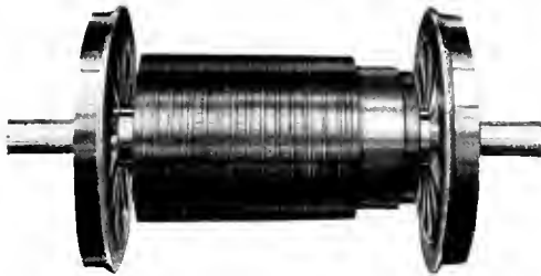
Fig. 7. Armature and Wheels of 3000-volt Direct-current Gearless Locomotive
