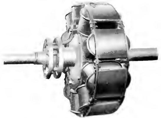
Fig. 6. Synchronous Motor Rotor Having the Amortisseur Winding Before the Laminated Poles Were Riveted
