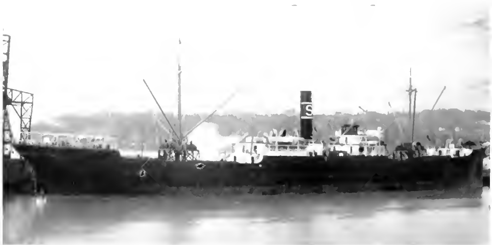
Fig. 1 S.S. Hanna Nielsen Propelled by a 2500 h.p. Two plane Type Marine Geared Turbine. This ship has an active service record of over four years without any repairs or replacements being required for its turbine equipment.
