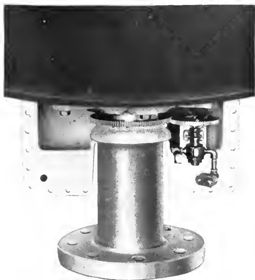
Fig. 9. Pump in Oil Pan of Lower Guide Bearing on Vertical Generators. One-half of pan removed for inspection of pump
