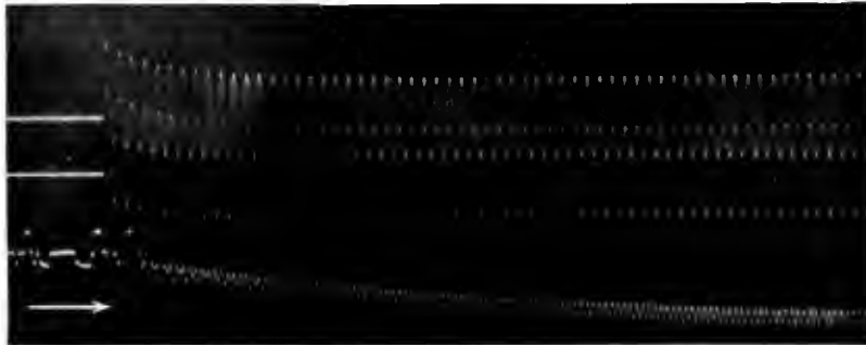
Fig. 8. Single-phase Short Circuit, Alternator Controlled by Automatic Regulator. Lower curve shows the rapidity with which regulator contacts close to increase excitation
