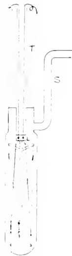
Fig. 48. Hale's Improved Form of Pirani Gauge
