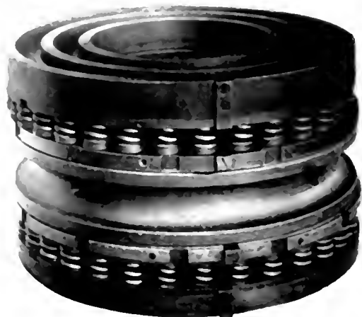
Fig. 12. Spring Thrust Bearing for Marine Propeller Shafts
