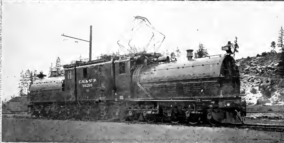
Mallet Type Freight Locomotive Formerly Used on the Mountain Divisions of the C. M. & St. P. R. R. and the New Electric Passenger Locomotive for the Cascade Division of the same Railroad
