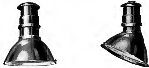
Fig. 3. Accurate Color Matching Units for Industrial Purposes. Light from a Mazda C Lamp is Reflected Downward Through a Glass Color Screen. The unit on the right, of the angle type, produces high illumination on vertical surfaces
