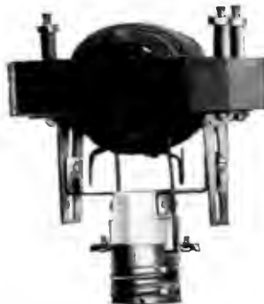
Fig. 13d. Illustrating the Series Auto Transformer and Its Application
