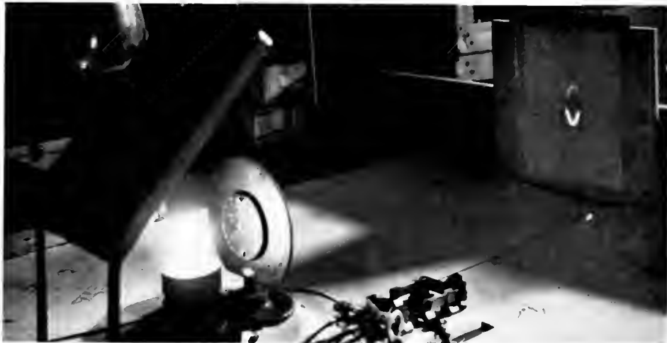
Fig. 16. Optical Device for Testing Light Center Length of Lamps
