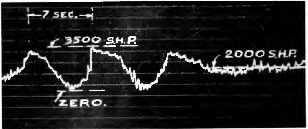
Fig. 7. Record from Torsion Spring Coupling on S.S. Jebsen in Ballast in a Moderately Rough Sea. Average r.p.m. 78. Average shaft horse power about 2000. Part of the smaller fluctuations shown came from an untrue collar in the instrument; otherwise record is correct.
