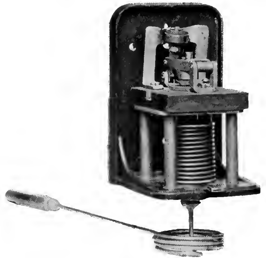
Fig. 24. Temperature Relay, with Cover Removed, used for Protection against Hot Bearings in Automatic Generating Stations
