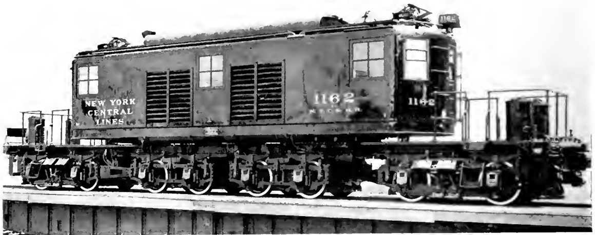
Fig. 9 Latest Type Gearless Passenger Locomotive in Service in the New York Central Electric Zone
