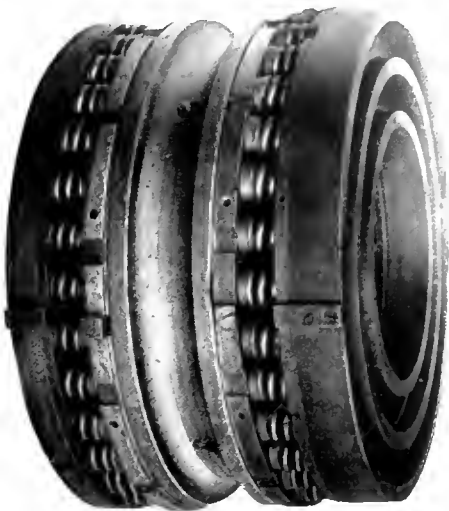
Fig. 12. Spring Thrust Bearing for Propellor Shaft
