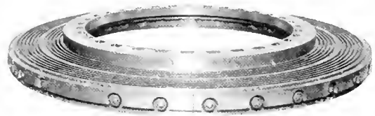
Fig. 6. Completed Armature Ready for Sawing Into Two Sections
