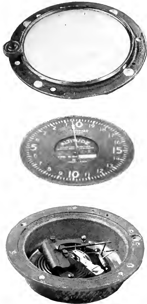
Fig. 8. The Instrument which Indicates to the Aviator the Height at which He is Flying
