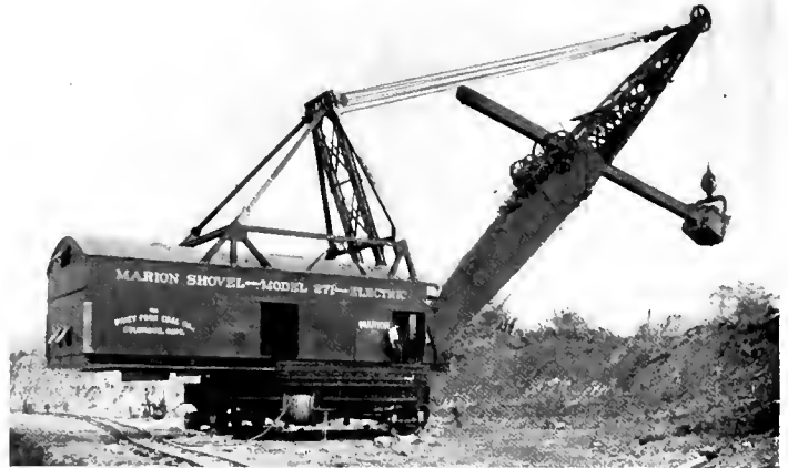
Fig. 38. Electric Stripping Shovel, Piney Fork Coal Company, Smithfield, Ohio
