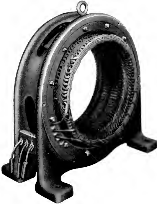
Fig 9 Coreless Box Type Stator Frame Used for the Smaller Machines
