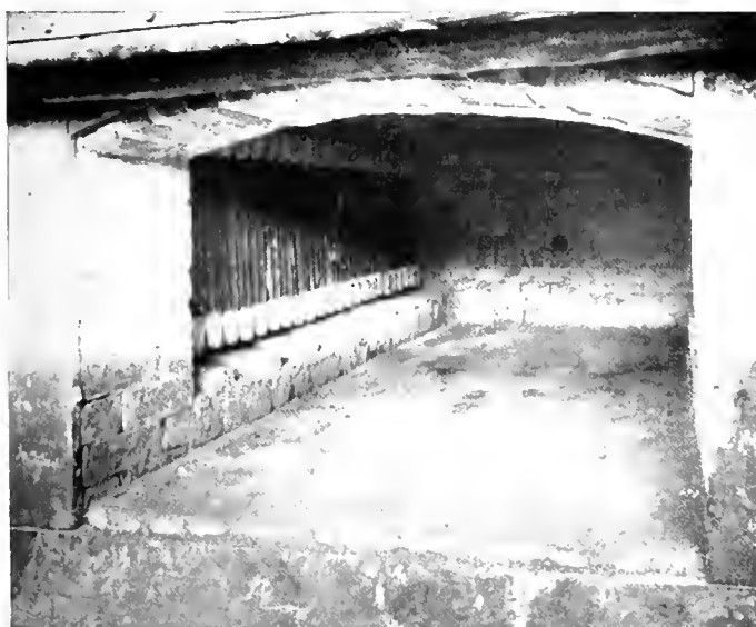
Fig. 5. Interior View of Box Furnace Used for Carbonizing
