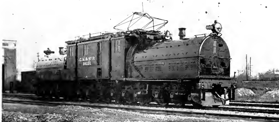
Fig. 6. High Speed Gearless Passenger Locomotive for the C., M. & St. P. Rwy. 3000-volt Direct-current Electrification
