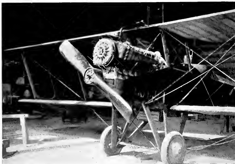
Le Pere Biplane after trial flight at McCook Field, Dayton, Ohio. The General Electric Super-charger is shown mounted on the head end of the Liberty Motor
