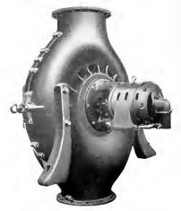
Fig. 1. Single-stage Centrifugal Air Compressor rated 10,000 cu. ft. per min. at 1.25-1b. per sq. in. discharge pressure, driven by a 2-pole, 75-h.p., 3600-r.p.m. induction motor
