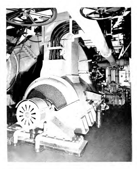
THE ALL ELECTRIC EXPRESS AND PASSENGER SHIP CLBA, SHOWING STARBOARD SIDE OF THE PROPULSION TURBINE GENERATOR
