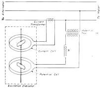
Fig. 2. Diagram of Excitation Indicator
