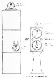
Fig. 2. Selsyn Position Indicator Pedestal Designed for Installation in Switchboard and Generator Rooms of Large Power Statioos
