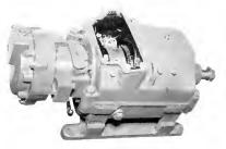
Fig. 2. Direct-current Deck Motor with Disc Type Solenoid Brake, Hand Hole Cover Removed for Inspection
