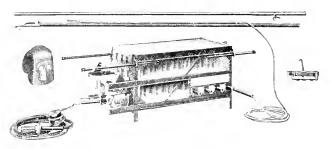
Fig 7. 400 650-volt Resistor Arc Welder
