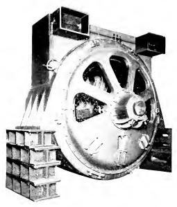
Fig. 1 A Typical Form of Induction Motor for Merchant Marine Propulsion
