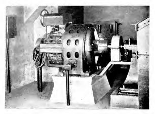
Fig. 1. 150.h.p., 720.r.p.m., 2200 volt, Varying-speed Brush Shifting Motor with Automatic Brush Shifting Mechanism Direct-connected to Forced Draft Fan. The panel mounts the pilot motor, contactors and brush shifting motor overload relays. One push button station and control circuit transfer switch is mounted on the wall
