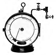
Fig. 2. General Electric Indicating Recording Flow Meter
