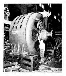
One of the Propeller Motors. The Maryland has four such induction motors each of 7000 h.p. and 170 r.p.m. The motor is 12 ft. in diameter and weighs 62 tons
