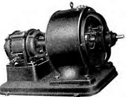
Fig. 5. Motor-Generator Set for Obtaining High-voltage Unidirectional Precipitation Current
