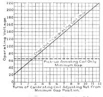
Fig. 2. Range of Calibration of Voltage-drop Relay on 250-volt Circuit
