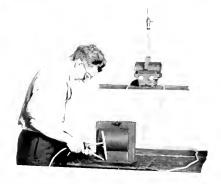
Fig. 8 General Electric Pyrotip Soldering an Alloy Flange to Sheet Iron Tank.
