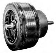
Fig. 5. Completely Wound Rotor of Scherbius Regulating Machine
