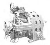
Fig. 1. Type BTS-10-150-720-r.p.m., 2200-volt Motors with Master Switch (cover removed) and Pilot Motor for Automatic Brush-shifting Control Actuated by Air Pressure or Push Button
