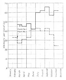
Fig. 2. Monthly Kilowatt-hour Consumption Per Ton of Ice Manufactured in the Plants Referred to in Fig. 1
