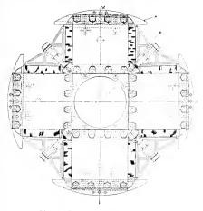
Fig. 24. Rotor Assembly of 7000-kv-a., 750-r.p.m., 14,000-volt Alternator
