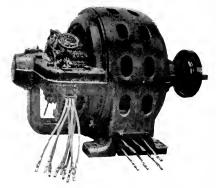
Fig. 3. Type BTS 300-h.p., 750-r.p.m., 550-volt Motor with Worm and Hand Wheel for Shifting the Brushes
