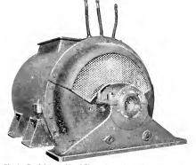
Fig. 1. Partial Assembly of Three-phase Aiternating-current Generator for Electric Propulsion of Cargo Boats
