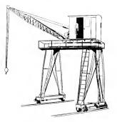
Fig. 30. A Portal Revolving Jib Crane. The jib revolves completely around, the cab moves crossways, and the bridge can move lengthways. Variations of this crane are useful for unloading boats, railroad crs. 1, to a tons for ship's cargo. The speed is about '2; to I trip per minute. Railroad tracks can be bridged, and the rear can be supported on a building instead of on ground level track
