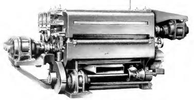
Fig 1 Six-drum Sander with Motors Coupled Directly to Drums, Feed Motor Below
