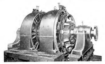
Direct-current Double Armature Motor for Diesel-electric Marine Drive
