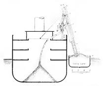
Fig. 44. The Micheuer Portable Bucket Couveyor arranged for filling the bunkers of an ocean liner with coal from a barge at the rate of approximately 125 tons an hour. On large boats several machines are used simultaneously
