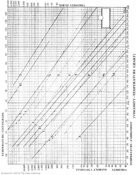
Chart 1. A to I Represent Well Refined Naphthene Base Oils Which Are Practically Free from Paraffine and it Should be Noted That the Viscosity Lines Are Almost Parallel. The other oils are from a different class of crude and while the viscosities are similar the lines have a different slope and not all of them are traight
