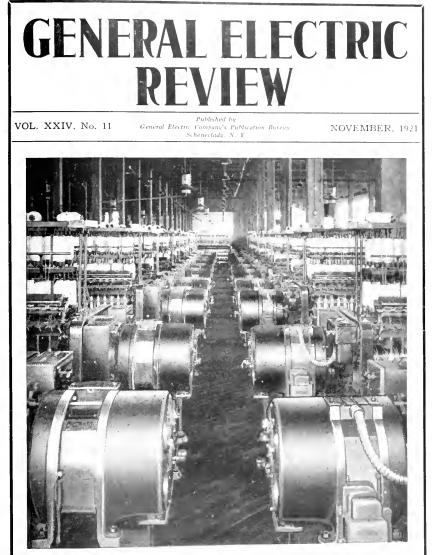
SINGLE-PHASE VARYING SPEED BRUSH-SHIFTING COMMUTATOR MOTORS DRIVING SPINNING FRAMES (See article, page 921)
