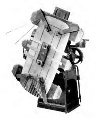
Fig. 5. The Difference in Tension Applied in Winding a Rectangular Coil is Illustrated by the Difference in Lever Arm, i.e., the Difference in the Distances from the Spindle to the Sides. It is impossible to obtain uniform tension in such a coil structure
