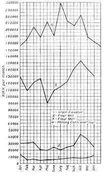
Fig. 2. Curves of Seasonable Distribution of Load in Flour Mills and Grain Elevators
