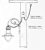
Fig. 17. Installation of Aerial Type Series Transformer
