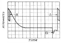
Fig. 1. Elevator Duty Cycle Curve. Shaded Area A represents power saved, and Area B power returned to line, by a 2:1 squirrel-cage motor
