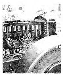
Fig. 2. Contactor Control and Motor Equipment fo. Trackless Trolley
