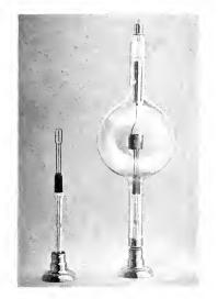
Fig. 11. Construction of the Kenotron Used in Place of the Mechanical Rectifier
