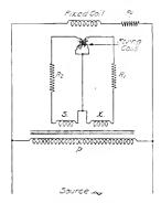
Fig. 6. Connection Diagram of Another Turncounting Device of Greater Precision Than That Shown in Fig. 3
