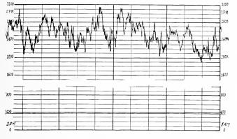
Fig. 1. Sample Kilowatt Time Curves from Power House Supplying Five Mines No Main Hoists Connected
