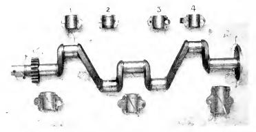
Fig. 3. Crank Pins and Main Pearings of an Automobile After 20,000 Miles Service. Connecting Rod Bearings Equipped with Genelite. The main bearings showed decided wear, while the crank pins were barely polished and the connecting rod bearings had not come to a full seat
