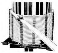
Fig 1 Helical Low-Voltage Coil in Process of Winding on Insulating Cylinder
