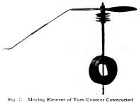
ig. 7. Moving Element of Turn Counter Constructed in Accordance with Fig. 6
