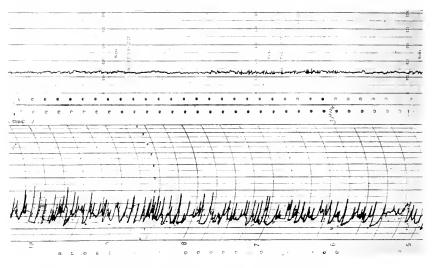
F1g 2. A Comparison Between Automatic and Hand Control of Furnace Electrodes. Upper curve shows kilowatt input with automatic control and lower curve kilowatts input with hand control
