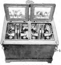
Fig. 2. Rectifier Tank Showing Tube Carriers and Water Cooling Coils
