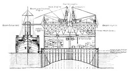
Fig. 3. Straight Line Motion Roof Crane for Use on Narrow Piers Where Space Does Not Permit the Use of Half or Full Arch Gantry Cranes
