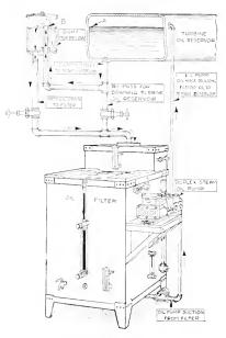
Fig. 5. Part Sectional View of Turbine Oil Reservoir Showing How Oil Level is Maintained
