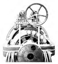
Fig. 9 Another View of Control Equipment for 150-h.p., Brush-shifting Motor
