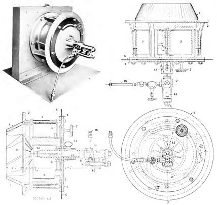
Figs. 3 and 4. Photograph and Drawings of the Babcock & Wilcox Oil Burner
