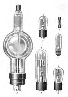
Fig. 4. Vacuum Tubes of Sizes from 5 to 250 Watts Fower Output
