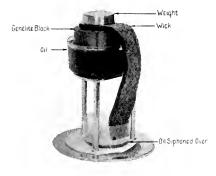
Fig. 2. Test Demonstrating Porosity of Genelite
