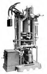
Fig. 1. Mercury Arc Rectifier Outfit for Series Luminous Arc Lighting (Interior View)
