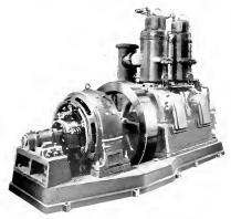
Fig. 3. Oil Engine Generator Set Designed for Service on a Motor-ship
