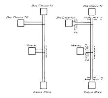
Fig. 1. Connections of Stations for Changing the Voltage of the Southern California Edison Company's 150,000-volt Transmission System to 220,000 Volts. Present connections at the left. Proposed connections at the right, in which each transformer is to have a capacity equal to 100 per cent of its station capacity.
