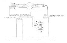
Fig. 2. Diagram Showing Stabilizer in Low-tension Circuit
