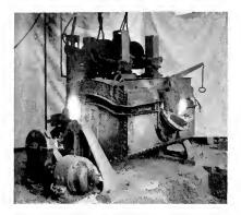
Fig. 6. Two-ton Three-phase Electric Arc Furnace Developed at the Schenectady Plant About 1908. At the time it was the largest capacity electric steel furnace in existence
