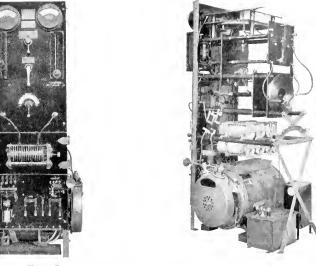
Fig. 2. Front and Eack Views of Two-kilowatt Spark Type Transmitter, Standard for Ships for the Past Eight Years
