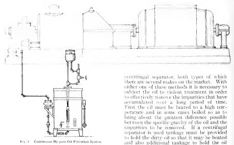
Continuous By-pass Oil Filtration System F12. 4
