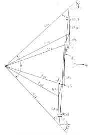
Fig. 3. Vector Diagram of Two Alternators with Constant Nominal Voltage, Paralleled Over a Transmission Line and Pulled Apart by an Angle 0
