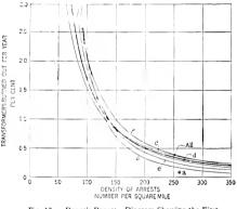
Fig. 17. Roper's Paper) Diagram Showing the First Approximation of the Relation Between the Density of Arresters and the Percentage of Transformers Burned Out by Lightning for the Five-year Period, 1915-1919 Inclusive
