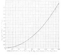
Fig. 11 Speed at Which a Falling Body Strikes Versus Height of Fall in Inches
