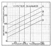
Chart 3. Approximate Variation of Bearing Temperatures with Atmospheric Temperature
