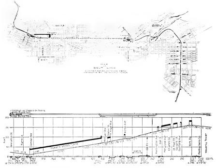
Fig. 2. Map, Track Chart, Profile, and Curvature of the Belt Line, Baltimore, Md.
