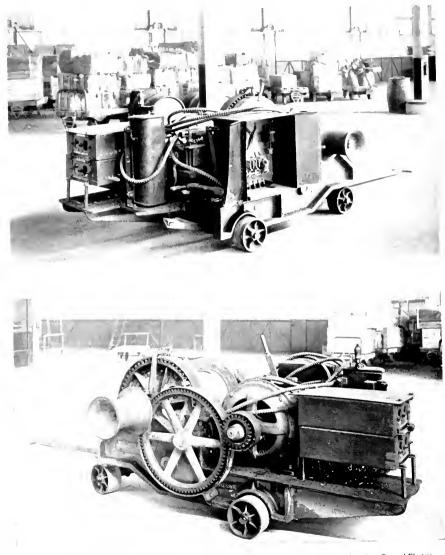
Two Views of a Portable Electric Dock Winch Used at the Brooklyn Army Base. The Winch is Driven by a General Electric Alternating current Motor Current is Supplied Through a Flexible Cable Attached to a Plug Outlet
