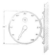
Fig. 17. Geared Selsyn Generator for Miscella neous Purposes
