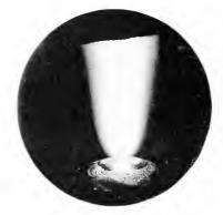
Fig. 1. Are and Tips of the Electrodes of the Luminous Arc Lamp. The arc rises from a molten pool of oxides, spreads out, and furnishes all the light emitted from this type of lamp
