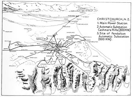
Fig. 1. Layout of Christchurch, N. Z., Tramway Board's Track, Showing Position of Power House and Substation
