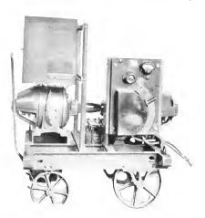
Fig. 5. Portable Single-operator Constant Energy Arc Welding Machine 60 20-volts 200-ampere
