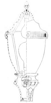
Fig. 9. Part Sectional Drawing of the Duoflux Lighting Unit Used in the Lighting Installation at Saratoga, N. Y.
