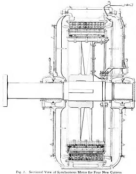
Fig. 2. Sectional View of Synchronous Motor for Four New Cutters for the Coast Guard Service
