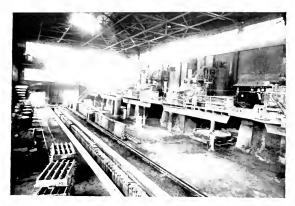
Fig. 6. An Up-to-date Electric Furnace Installation for Producing High-grade Tool Steels. The present equipment consists of four 6-ton furnaces, each taking 1500 kw.
