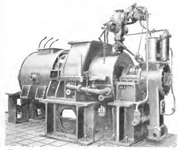
Fig. 5. 3000-h.p., 3000-r.p.m. Marine Turbine Generator Set, Looking Aft
