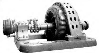
Fig. 14. Main Roll Motor with O. D. Exciter
