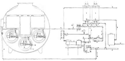
Fig. 2. Arrangement of Dahl Mechanical Fuel Oil Burning System
