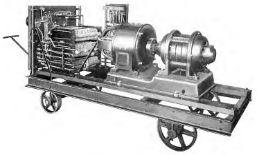
Fig. 6. General Electric Portable Constant Potential Multiple Unit Arc Welding Machine
