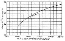
Fig. 1. Efficiency Curve of a Double-reduction Gear
