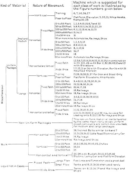
Chart Showing Machine or Machines Best Adapted for Handling Mate ials in Bulk or in Packages Through Horizontal and Vertical Movements
