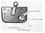
Fig. 21. Top of Electric Braking Controller Showing Control Levers
