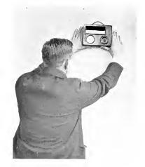
Fig. 21. Reading Illumination on a Vertical Surface with the Foot-candle Meter
