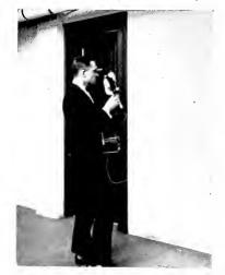
Fig. 20. Measuring Vertical Illumination of Wall Brightness with the Macbeth Photometer
