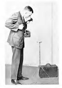
Fig. 18. The Macbeth Photometer as Employed to Measure Illumination in the Horizontal Plane
