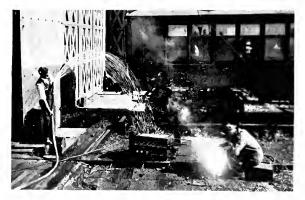
Fig. 45. Testing New Type of Resistor for Arc Welder by Spraying It with Water when It is Operating at Maximum Temperature
