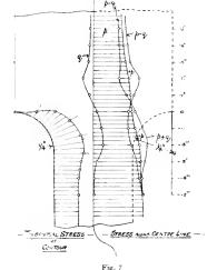
curves of 0.25-in, radius, the isoclinic lines, Fig. 5, define a region of complex stress extending to nearly  $1_2$  in, into the enlarged ends and slightly over 0.4 in, below the shoulders. Above and below these sections approximately uniform stress conditions are obtained as the lines of principal stress, Fig.
