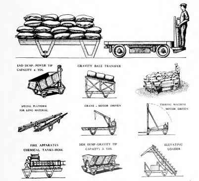
Fig. 16. An Electric Storage Battery Operated Platform-carrying\Truck. It weighs 4500 lbs. and elevates 5000 lbs. on a 48 sq. ft. platform through 9½ in. and carries this load at a maximum speed of 7 miles per hour, into box cars or indoors through 6-ft. aises and on city strets. It is useful for distances between 75 and 5000 ft. for carrying material or machines on any of the platforms shown
