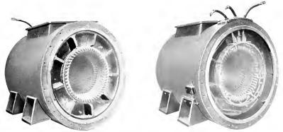
Figs. 4 and 5. End Views of G. nerator of Fig. 1, Showing Form-wound Coils Completely Assembled. Note the method of supporting end windings by steel binding bands
