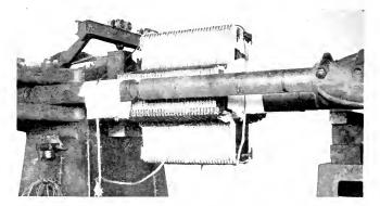
Fig. 5. Rotor Spider of a 4-pole, 7.000-kv-a., 750-t.p.m. Waterwheel Driven Alternator Wound to be Heated Electrically by Induction. Primary winding consists of 32 turns of 430,000 cir. mil bare copper cable
