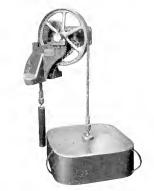
Fig. 10. Water Level Transmitter, Panama Canal Locks
