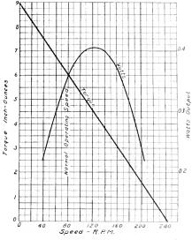
Fig. 1. Speed-torque and Power Curves of the 110-volt 60-cycle Disc Phonograph Motor
