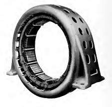
Fig. 4. Partly Wound Stator of Scherbius Regulating Machine
