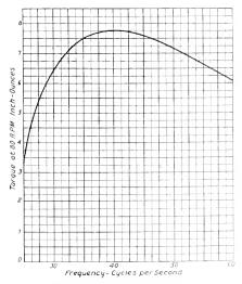
Fig. 2. Torque Curve of the Disc Phonograph Motor at 80 R P M 110 Volts and Frequencies Between 25 and 60 Cycles
