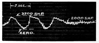
Fig. 2. Record from Torsion Spring Coupling on Jebsen in Ballast in a Moderately Rough Sea. Part of the smaller fluctuations resulted from an untrue collar in the instrument; otherwise the record is correct
