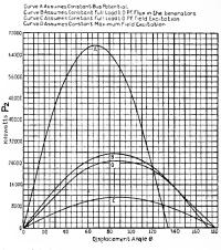
Fig. 5. Calculated Synchronizing Power of Two 12,000-kv-a. 6600-volt Generators Paralleled Through a Transmission Line
