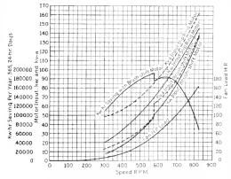
Fig. 12. Comparative Kw. and Kv-a. Input for 150-h p., 720-r.p.m., and 150-h.p., 900 r p m. Slip Ring Motor Under Actual Fan Load
