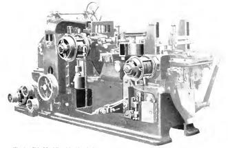
Fig. 2. Side Moulding Machine Driven by Five Squirrel Cage Motors, Two Horizontal and Two Vertical, All Directly Connected to Spindles. Feed Motor is Shown at Left Near the Floor
