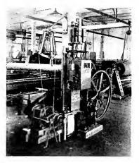
Fig. 18. BTS 7<sup>-1</sup><sub>2</sub>-h.p., 1200-r.p.m., 220-volt Varying Speed Brush-shifting Motor (hand control) Connected by Chain to 50-ft. Woolen Tenter Frame. Hamilton Woolen Company, Southbridge, Mass.
