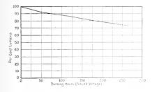
Fig. 1. Typical Performance Data on an Incandescent Lamp
