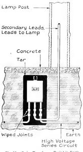
Fig. 18. Series Transformer Buried in Earth
