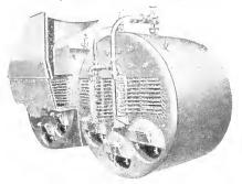
Fig. 2. Scotch Boiler with Fire-tube Type of Live-gas Superheater
