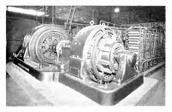
Fig. 9. Main Roll Drive Kraemer System Showing D.c. Motor Mounted on Main Roll Shaft with Induction Motor
