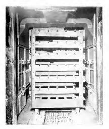
Fig. 5. Electrically Heated Core Baking Oven, Showing Loaded Truck and Electric Heaters. Oven 10 ft. long, 5 ft. wide, 7 ft. high, 72 kw. connected
