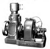
Fig. 1. Steam Engine Generator Set for Lighting Service on Moderate Size Vessels
