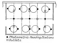
Fig. 1. Diagram Showing Arrangement of Machinery, Position of Outlets and Location of Photometric Reading Stations
