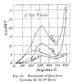
hour treatment at each of the above temperature ranges is sufficient, and makes the interesting observation, which is in accord with that made by Sherwood (see below), that while the gas evolution at temperatures below 500 deg. C. practically ceases at the end of one half hour, the evolution of water vapor at higher temperatures continues indefinitely no matter how long the heating period.
