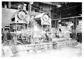
Fig. 3. Alexanderson Alternator Installed in High Power Radio Station
