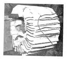
Fig. 2. Rotor Spider Wound to be Heated Electrically by Induction. Primary winding consists of 35 turns of 250,000 cir. mil bare copper cable wound around the rim through the ventilating holes in the web
