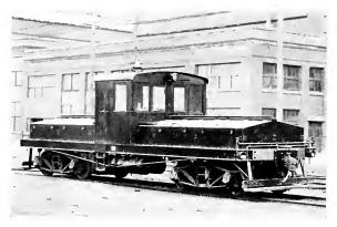
Fig. 22. 40-ton Storage Battery Locomotive
