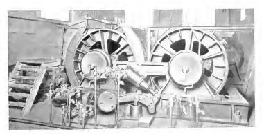
Fig. 13. Hoisting Engine on Cableway Consolidated Gas Electric Light and Power Company, Baltimore, Md.
