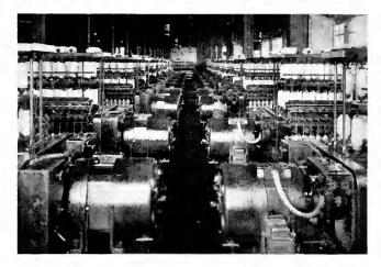
Fig. 38. Single-phase Varying Speed Spinning Frame Motors. Group showing coupling connected with P-10 non-automatic starters. Saratoga Victory Mfg. Co., Victory Mills, N. Y.
