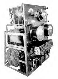
Fig. 3. Spark Transmitter, One-half Kilowatt Navy Type, Used on Small Craft Such as Sub-chasers
