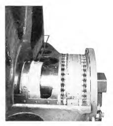
Fig. 5. Spring Thrust Bearing for Propeller Shaft of S.S. Cuba The thrust bearing is at the forward end of the shaft in the bracket of the driving motor
