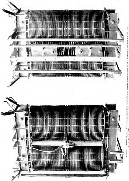
pany by the Pittsfield Works of the General Electric Company. These are the first transformers to be supplied by any manufacturer for regular commercial service at 220-kv. They embody the circular-coil construction, which long service has shown to be superior to any other form of coil and which the General Electric Company has strongly advocated for large highvoltage transformers. These transformers were described in an article by Mr. Clinton Jones in our May issue.
