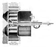
Fig. 6. Bethlehem Furnace Front for Either Forced or Natural Draft Fitted with Dahl Burner
