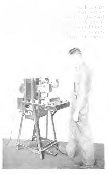
Fug. 7. Electric Rivet Heater, 15 Kw., 220 Volts, 75 Amp., 60 Cycles.
