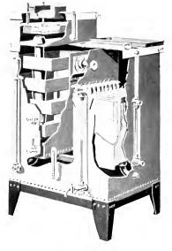
Fig. 6. Sectional View of Oil Filter
