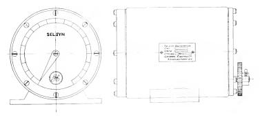
Fig. 16. Selsyn Power Demand Indicator for Generator Room and Boiler Room. These indicators show anticipated power requirements
