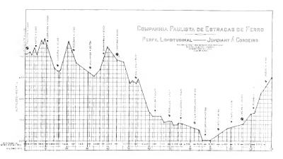
Fig. 2. Profile of the Section of the Paulista Railway Between Jundiahy and Cordeiro
