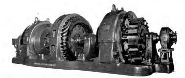
Fig. 5. 1500-kw., 3000-volt, Direct-current Motor-generator Set. Three of these are being installed in the Louveira substation
