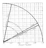
Fig. 5. Phase Angles of Potential and Current Coils at 60 Cycles
