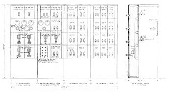
Fig. 2. A Dead-front Switchboard for Control of Two Auxiliary Generators and Balancer Set and for Distribution of Power and Lighting Aboard Ship
