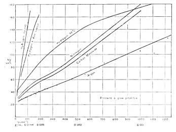
Fig. 70. Relation between Pressure and Glow Potential for Various Gases
