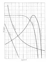
Fig 3. Speed-torque Characteristics of Various Types of Motors
