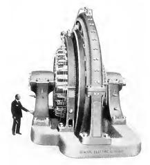
Fig. 5. Enormous Size of a Large Rotary Converter for Electrolytic Work, the output being 13,000 amperes at 525 volts
