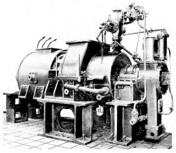
General Electric Marine Turbine-generator Set which, with Induction Motors or Synchronous Motors, is Used for Electric Propulsion. The set is not made reversible as astern movement is obtained by reversing the motors
