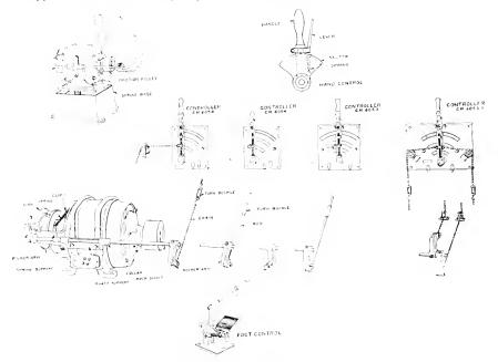
Fig. 32 Various Control Devices Used with BSS Motors
