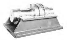
Fig. 2. Spring Thrust Bearing Showing Method of Attaching ] Rotating Ring of Bearing to the Shaft
