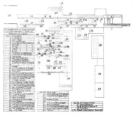
Fig. 5. Plan of the Sawing Floor
