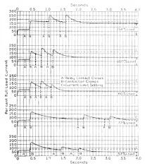
Fig. 6. Accelerating Curves of Series Motor with Acceleration Control by Voltage-drop Relays
