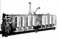
Fig. 5. Arrangement of Main Control Contactors (front view), Showing Arc Chutes and Flush Barriers
