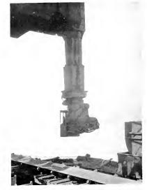
Fig. 2. Coal Trimmer at Bottom of Telescope Chute. Collecto Rings (with Cover Removed) Just Above the Operator's Cab
