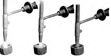
Figs. 8, 9 and 10. Showing Three Stages in the Application of the Pyrotip to Lead Burning for Storage Battery Work
