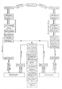
Fig. 1. Flow Chart Showing the Processes and Machines Employed in Paper Manufacture
