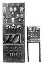
Fig. 42. Electrode Control Panels for Arc Furnace
