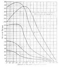
Fig. 4. Typical Speed-torque Curves of the Brush-shifting Motor for Various Positions of the Brushes
