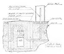
Fig. 20. Series Transformer Installed in Manhole
