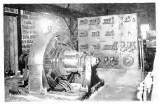
Fig. 8. Synchronous Converter Kraemer System
