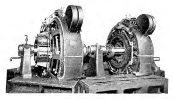
Two Direct-current Generators for Diesel electric Marine Drive on Testing Stand
