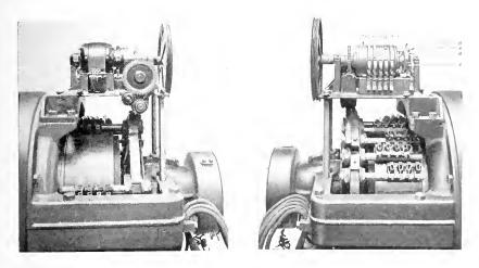
Figs. 7 and 8. Two Views of Pilot Motor Gear Train, Rope Wheel, and Drum Control Switches for Automatically Controlling a 150-h.p., 2200-volt Brush-shifting Motor from Push Buttons or Pressure Regulator. Cover Removed.
