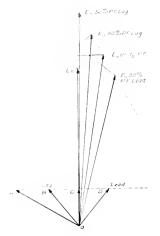
Fig. 2. Influence of the Power-factor of the Load on the Voltage Drop in a Transmission Line
