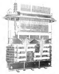
Fig. 7. Large Electric Furnace Transformers are the product of long experience and high skill, and the making use of the best materials available. This transformer takes power at 44,000 volts and delivers to each of three electrodes 26,600 amperes at 85 volts.
