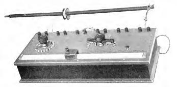
Fig. 5. Special Potentiometer, Based on Fig. 4, for Counting the Number of Turns in Instrument Coils
