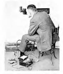
Fig. 17. Reading Illumination on a Horizontal Plane with the Sharp-Millar Photometer
