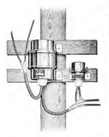
Fig. 15. Series Transformer (Large Capacity) and Protective Device
