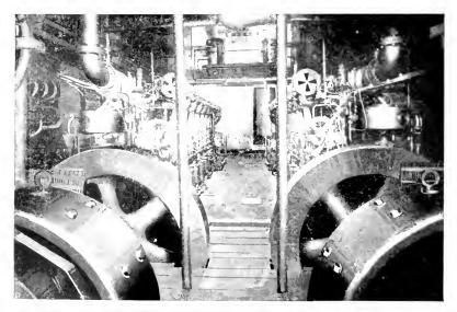
$=_6$  - Engine Receive looking aft , Showing Main Generators with the Engine Flywheels Carried on the Generator Shaft Bearings
