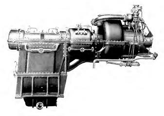
Fig. 7. Two-plane Type Marine Geared Turbine-Starboard or Operating Side
