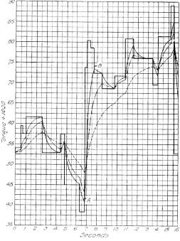
Fig. 11. Typical Rolling Mill Load Cycle
