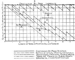
Fig. 3. Curve Showing Results Obtained from Various Methods of Purifying Steam Turbine Oil
