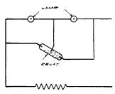
Fig. 11. Wiring Diagram of the Duoflux Unit Shown in Fig. 9
