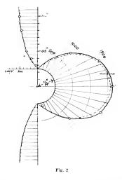
case of a uniform strip having two semicircular notches in it symmetrically disposed with reference to the axial line. Indeed such a form has occasionally been used for tension experiments, although, as Fig. 1A shows, there is no uniform stress distribution at or
