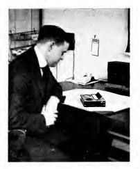
Fig. 19. Determination of the Illumination on a Desk Surface with the Foot-candle Meter
