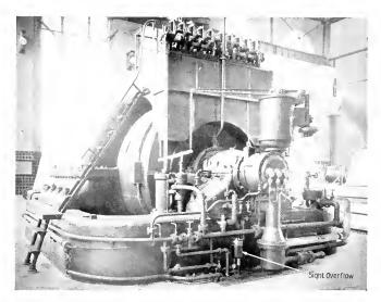
Fig. 7. 15,000-kw. General Electric Turbine Equipped with Continuous By-pass Filtration System
