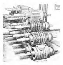
Worn Armature Shafts Built up by General Electric Constant Energy Welding Machine, Showing One Armature Shaft Machined
