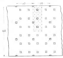
Fig. 16. Location of Test Stations in a Large Area
