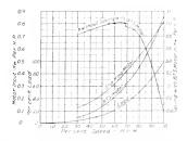
Fig. 9. Comparative Kilowatt Input Per Horsepower for BTS Motors and Slip Ring Motors Driving a Fan Load
