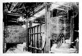
Fig. 44. Compensating Type Electric Furnace for Annealing Steel Wire
