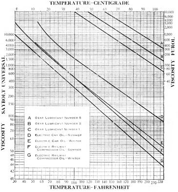
Chart 4 The Viscosities of Various Lubricants Recommended for Electric Street Railways at Different Temperatures
