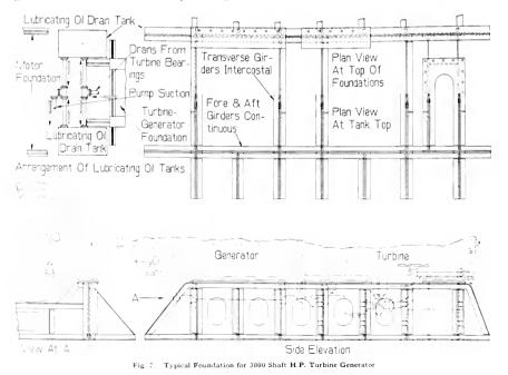
A typical foundation for a 3000-s.h.p. motor consists of two fore-and-aft deep girders, one under each foot of the motor. The girders are well gusseted to the tank top and are tied together on the forward and after sides by means of plate
