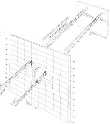
Fig. 8. Light Rays Passing Through Stressed Specimen
