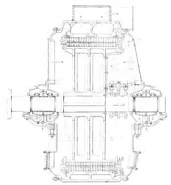
Fig. 2. Sectional View of Typical Induction Motor for Merchant Marine Propulsion
