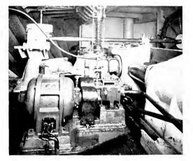
Fig. 3. Alternating-current Motor Operating Hydraulic Steering Gear
