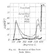
Apparently the glass actually suffers a chemi cal decomposition at higher temperatures.
