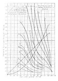
Fig. 6. Brush-shifting Motor Speed-torque Curves for Various Brush Positions with Both Delta and Y-connected Stator
