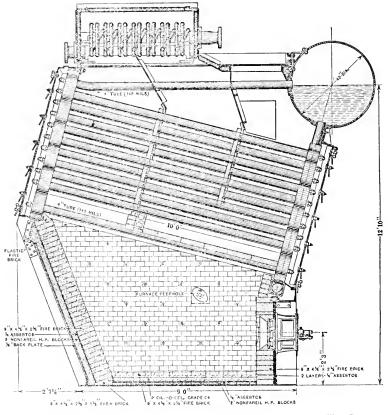
Fig. 1. Sectional Side Elevation of Water Tube Marine Boiler, Showing Tubes, Steam and Hot Water Drum, Superheater, and One Oil Burner
