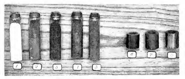
Fig. 1. Some of the Stages in Manufacturing Genetite Nos. 1, 2, and 3, Raw Materials; 4, Graphite; 5, Mixture Ready for Pressing; 6, Bushing Pressed from the Powder; 7, Bushing after Final Bake; 8, Finished Piece
