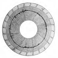
Fig. 4. A 24-hour Chart from a 1500-kw. Ferro-alloy Furnace, Controlled by General Electric Automatic Electrode Pegulator. On account of the nature of the alloy, the load fluctuated somewhat but the load-factor was 96.2 per cent
