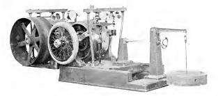
Fig. 41. Testing Automobile Tires by Means of Dynamometer Equipment in United States Bureau of Standards, Washington, D. C.
