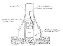
Fig. 19. Series Transformer Installed in Base of Post
