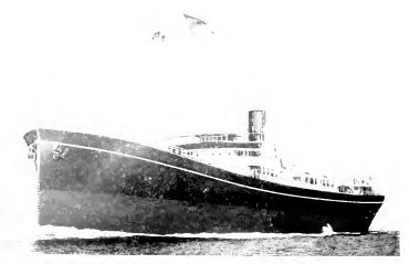
The Rohm Gray is an Express Freighter Propelled by a 3000 h.p. Turbine Geared Unit of the Two-plane Double-reduction Type. The boat entered the service in the early part of 1920
