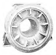
Fig. 2. Assembly of Armature Structure Showing Open Slot Laminations which Permit of the Use of Form-wound Coils
