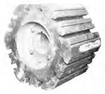
Fig. 6. Rotor Spider of a 6-pole, 3530-kv-a., 500-r.p.m. Waterwheel Driven Alternator
