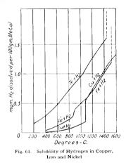
In the case of the metals, copper, iron, and nickel, the careful investigations of A. Sieverts and his associates<sup>11</sup> have shown that the amount of hydrogen dissolved at any given temperature varies with the pressure according to the relation
