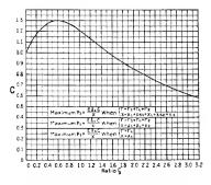
Fig. 8. Curve Showing Variation in Maximum P<sub>1</sub> for Constant Values of Reactance and Varying Values of Resistance When K = 1
