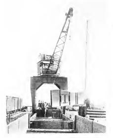
Fig. 1 Full Arch Gantry Revolving Jib Crane Handling Steel Directly from Cars to Lighter
