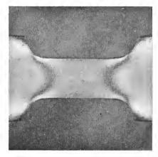
$(B) \quad \mbox{Tension member of approximately two units width connected to ends of four units width by quadrantal arcs of one unit radius.}$
