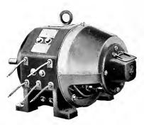
Fig. 27. 3-h.p., 1250-r.p.m., 550-volt Compound-wound Motor Designed for Mine Pump Operation
