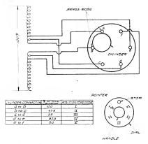
Fig. 3. Diagram of Connections for Ratio Adjuster
