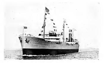
Fig. 2. S. S. Sucrosa of the Cuba Distilling Company, 5788 Gross Tons, Equipped with 2400-h.p. Marine Geared Turbine of the Two-plane Type
