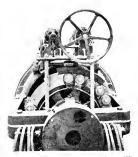
Fig. 16. Pilot Motor, Gear Train, Rope Wheel, and Drum Control Switches for Automatically Controlling a Brush-shifting Motor from Push Button Stations or Pressure Regulator
