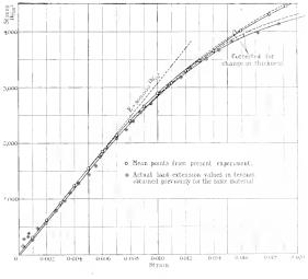
Fig. 15. Comparison of Stress-strain Curves
