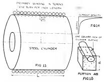
Figs. 13, 14, and 15. Schematic Diagrams for Deriving Mathematical Expressions for Current and Voltage
