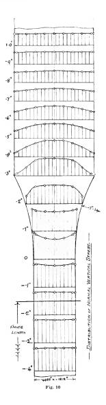
of the enlarged ends. It is therefore apparent that there is little to criticise in the form, since an increased contour stress seems inevitable for any form, but it would undoubtedly be safer to increase the minimum length of the parallel portion, and thereby avoid all risk of complex stress in the gauge length under any circumstances.
