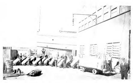
Sprague Electric Freight Truck Carrying 48 Cases of Canned Goods which as shown is Equivalent to 12 Hand Truck Loads
