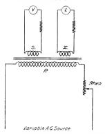
Fig. 3. Connection Diagram of a Device for Measuring Turns of Coils Within a Precision of 99 Per Cent
