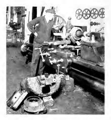
Fig. 3. Broken Cast Iron Motor Casing and Brake Housings Welded by General Electric Constant Energy Welding Machine Case Broken in Twelve Pieces
