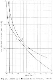
"Ungettered" Lamp A--Initial pressure, 1-33 bar (1 micron) B--Initial pressure, 6-67 bar (5 microns)
