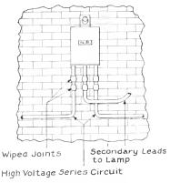
Fig. 21. Subway Installation in Series Transformer
