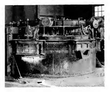
Fig. 11 Induction Type Furnace at Pittsfield Works, Waich Has Recently Completed 555 Heats on One Lining
