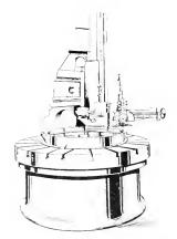
Fig. 5. Automatic Welding Head Supported on Boring Mill to Obtain Circular Weld
