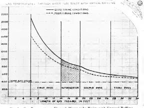
Fig. 4. Gas Temperatures Through Water-tube Boiler with Vertical Baffling
