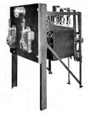
Fig. 66. Standard Panel for Control of 500-h.p. Three-phase Induction Motor
