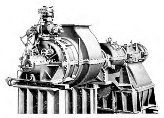
General Electric Marine Geared Turbine for Ship Propulsion. The turbine is of the Curtis high-speed type and has both "ahead" and "astern" elements. The gears are of the two-plane double-reduction type
