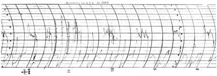
Fig. 4. Kilowatt Input to Shovel. Full scale equals 600 kilowatts. Interval between curved lines 15 seconds
