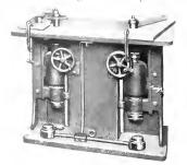
Fig. 5. Double Spindle Shaper, Each Cutter Driven by a High Speed Built-in Motor. Push hutton control panel concealed in base
