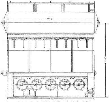
Fig. 2. Front Elevation of the Babcock & Wilcox Marine Boiler Shown in Fig. 1
