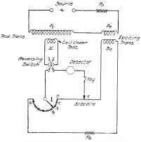
Fig. 4. Connection Diagram of a Turn-counting Device of Greater Precision Than That Shown in Fig. 3
