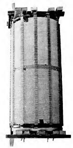
Fig 4 Completed Low-voltage Helical Coil in Clamps Ready for Varnish Treatment
