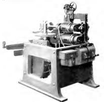
Fig. 3. Saw Tenoner with Directly Applied Motors for Driving the Three Saw Spindles. Manually controlled switches are mounted on the side of the machine
