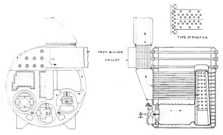
Fig. 1. Return-tube Marine Boiler, Showing Details of Construction Together with Oil Burners and Arrangement for Forced Draft with Pre-heated Air
