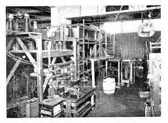
Fig. 1. Lightning Generator; high-tension transformer on floor at left behind table, kenotrons above, glass plate condensers at the side, main regulating sphere gap (vertical) in front of condensers, racks of regulating resistance rods immediately beneath, and test gap on barrel below
