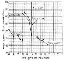
Fig. 15. Illustration of the Effect of the Thickness of the Glass of Globes Upon Light Transmission. The curves refer specifically to the type and size of globe shown in Fig. 3
