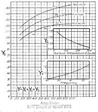
Fig. 4. Admittance Coefficient Y. Use Curve No. 1 when rotor spider has an irregular shape—large leakage flux. Use Curve No. 3 when rotor spider has no irregularities—small leakage flux
