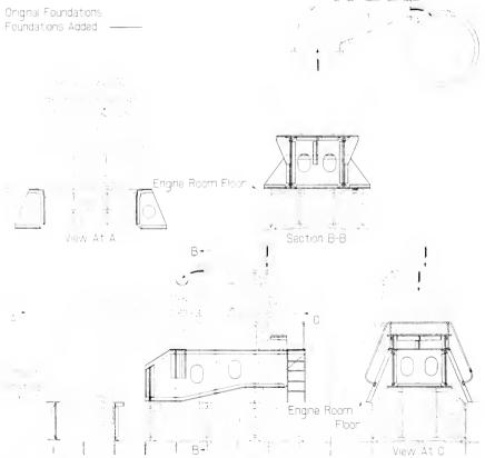
F 11 Diverse Showing Changes in Foundation Required when Substituting Two-plane Reduction Gear for Single-plane Gear
