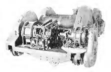
Fig. 11, Trolley Carriage with Alternating-current Crane Motors and Solenoid Load Brake Mounted on the Hoist Motor
