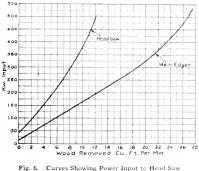
Fig. 6. Curves Showing Power Input to Head Saw and Main Edger
