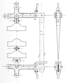
Fig. 74. Disconnected Switch, Showing Use of Hewlett Suspension Insulators
