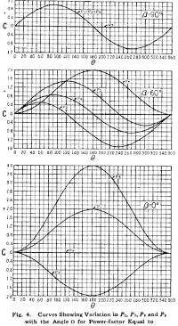
with the Angle  $\Theta$  for Power-factor Equal to Cos  $\beta$ , 0, 0.5 and 1.0
