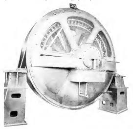
Fig. 1. 3000-h.p. Synchronous Motor of the Steamship Cuba
