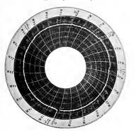
Fig. 3. Chart Indicating the Desirable Load of Large Electric Furnaces. It is a 24-hour load chart from a large calcium carbide furnace, the current being controlled within one per cent by a General Electric automatic electrode regulator
