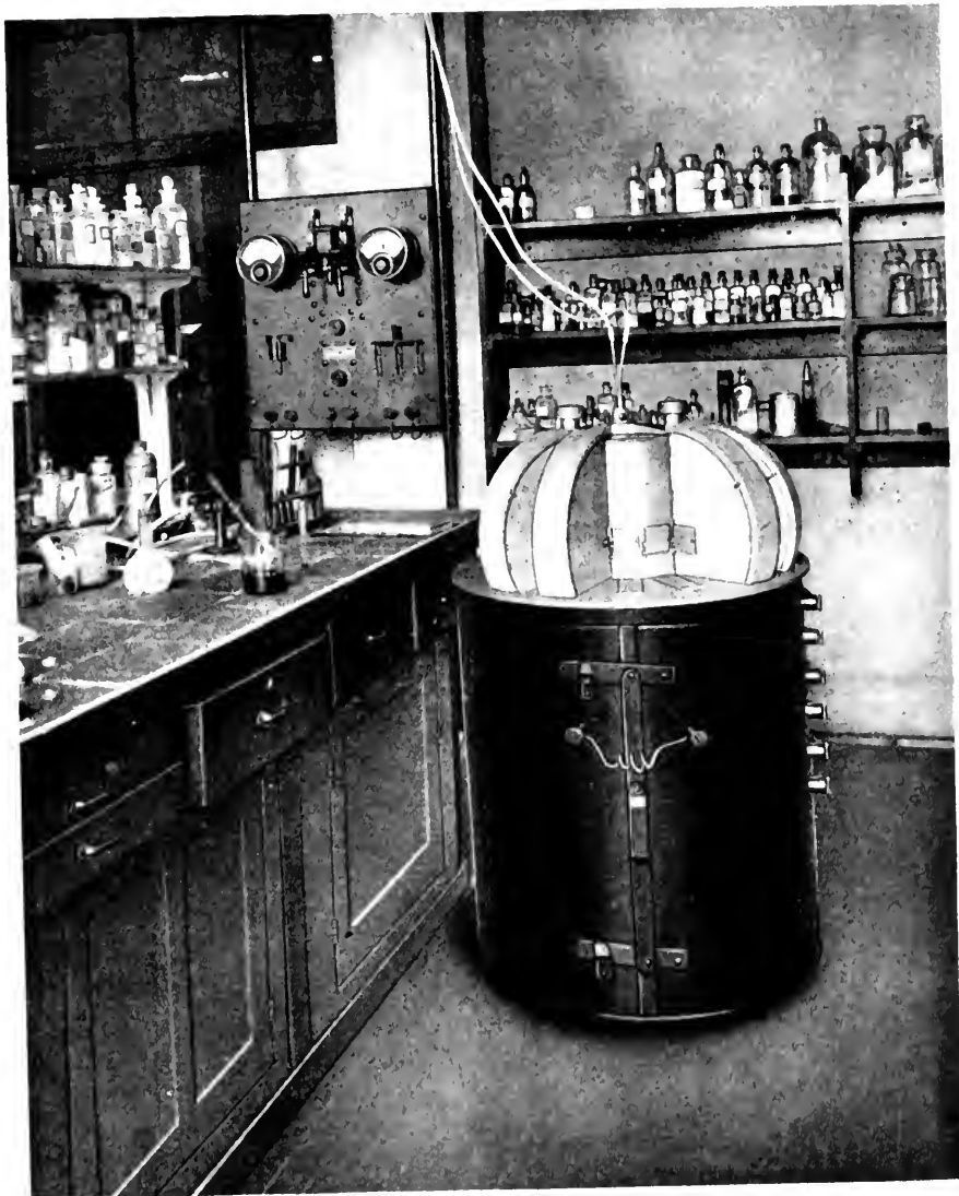
Crystal Analysis by X-ray Diffraction Apparatus, as described in this issue, has been used in scientific laboratories for some time. Its application to factory control work is more recent; but is extending. Our illustration shows an apparatus designed for this purpose.
