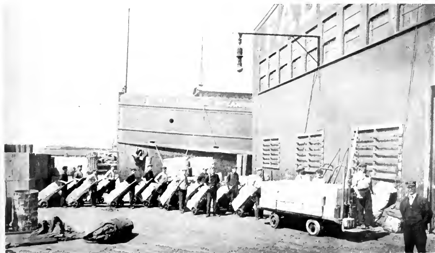
Electric Freight Truck Carrying 48 Cases of Canned Goods Which as Shown is Equivalent to 12 Hand Truck Loads
