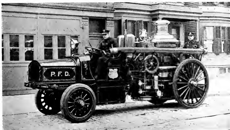
Fig. 6. Two wheel Steamer Tractor with Special Battery-mounting, Half on Each Side of the Front Driving Axle
