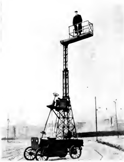
Fig. 5. An Electric Lamp Trimmer's Wagon with Center of Gravity so Low as to be Perfectly Stable When the Bridge is Raised and Offset. (Commercial Truck Company)
