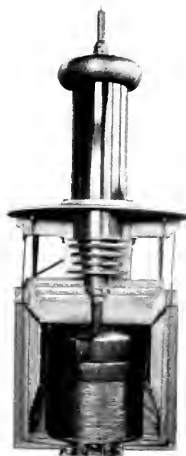
FIG. 4. Main Transformer Removed from its Tank; Front View, Showing the Tapered Major Insulation and the Extra-heavy Coil Insulation at the Top or Line End
