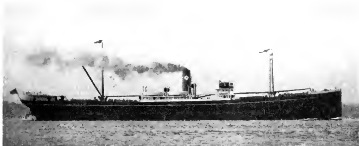
Fig. 3. Typical Cargo Vessel of Approximately 14,000 Tons Displacement Equipped with G-E Marine Geared Turbine. Nearly 300 have been placed in service
