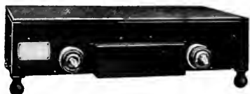
Fig. 11. 18 by 36-in., 6-kw. Electric Griddle. The heating unit is divided into a right and a left-hand section, each controlled by a separate three-heat switch and protected by individual cutouts mounted at the front of the device in a readily accessible box
