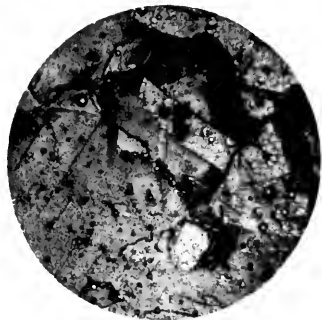
Fig. 4. Ordinary Copper Packed in Sea Sand in an Iron Pipe and Heated in Air to 800 Deg. C. for One Hour. 200 times magnification
