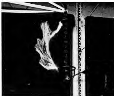
Fig. 3. Suspension Insulator String with Antenna or Shielding Ring of the Peek Type for Equalizing the Voltage
