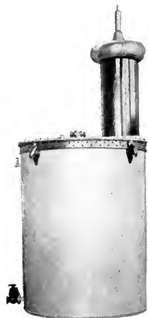
FIG. 3. Exterior View of the Main Transformer, 578,000 Volts. A similar unit stripped of cover, tank, and terminal is used as the line transformer
