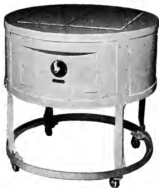
Fig. 13. 6-kw. Doughnut Stove. This device is intended to heat a 24-in. grease kettle and has a capacity of approximately 100 dozen doughnuts per hour
