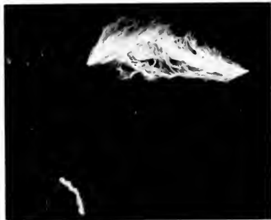
Fig. 12. The Upper Arc, Which Occurred at the Proper Place Between the Terminal Points, arc of Several Successive Discharges Across a 9-ft. Gap Between Sharp Points, and Started by a Million Volts from Line to Ground. The lower discharge took place from the cap of the main terminal to a fence in the background. This accidental arc was photographed nearly end-on and does not indicate its length of 13 feet. The two strong lines near the arc show respectively the curved outline of the cap and the straight surface of the terminal by reflection from the arc. The location of this latter arc is shown in Fig. 13 at the points marked A and a
