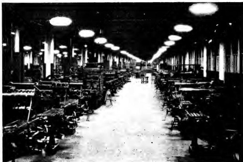
Figs. 1 and 2—The glaring local light shown in the top picture is a menace to safety and vision and is one of the evils which lighting coils are aiming to destroy. Contrast the lighting of this milling machine with the lighting of those shown in the bottom picture.
