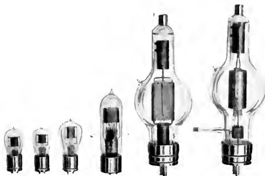
Fig. 1. Group of Radiotrons Used as Power Oscillators and Amplifiers in Radio Transmission and as Detectors, Oscillators, and Amplifiers in Radio Reception
