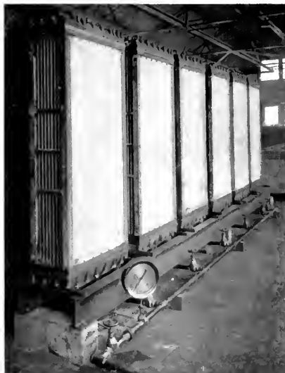
Fig. 3. Group of Surface Coolers on a Hydraulic Test Stand
