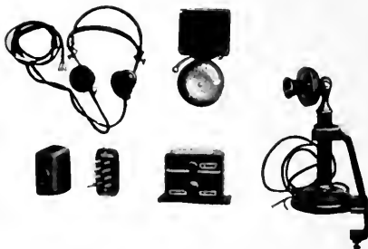
Fig. 11 Extension Station Equipment for 200 and 1000-watt Radio Telephone Transmitters
