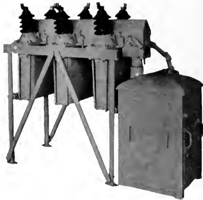
Fig. 53. 15,000-volt, 400-amp. Triple Pole Solenoid Operated Oil Circuit Breaker
