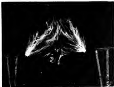
Fig. 18. Spark-over Between Needle Points at One Million Volts. Distance about nine feet
