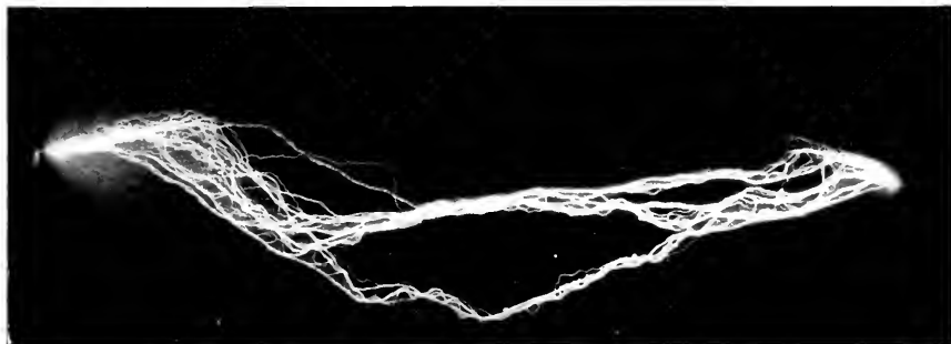
Fig. 17. Successive 1,500,000-volt Arcs over a 14-ft. Gap. The brush discharge before the spark took place shows particularly strong on the left terminal
