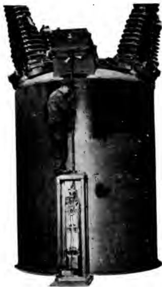
Fig. 56. 200,000-volt Oil Circuit Breaker Showing Arrangement of Triple Solenoid for Operating Mechanism
