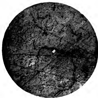
Fig. 3. Ordinary Copper Packed in Sea Sand in an Iron Pipe and Heated in Air to 800 Deg. C. for One Hour. 200 times magnification
