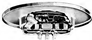
Fig. 3 Sectional View of Sheath-wire Hotplate
