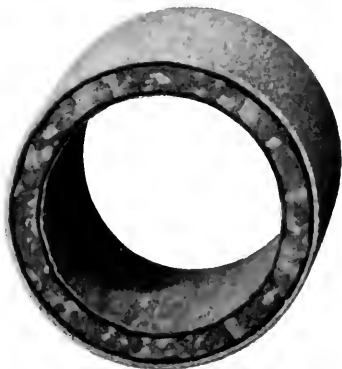
Fig. 2. Calorized Steel Showing Oxidization of Unprotected Section
