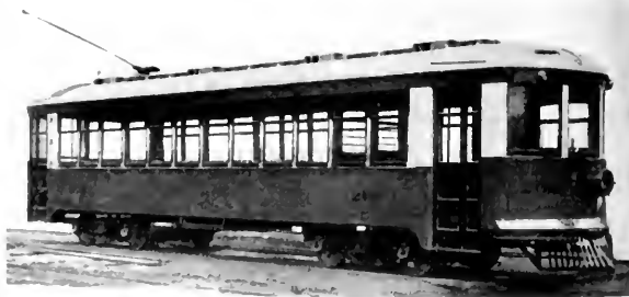
Fig. 2. Single End 14 ton, 48 passenger Car with Baggage Compartment in Operation on Union Traction Company, Nashville, Since January, 1920
