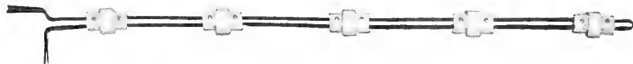
Fig. 27. Ribbon Resistor Forming Electric Heating Unit for Insertion in Tubes of a Fire Tube Steam Boiler
