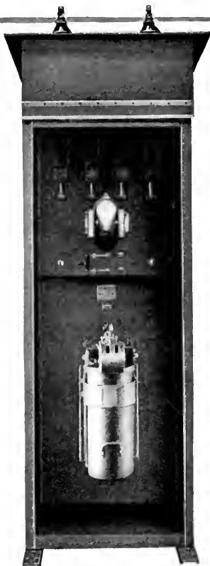
Automatic Reclosing Outdoor Substation (door removed), including oil circuit breaker, centrifugal operating mechanism, and necessary relays and instruments. Can be furnished for service on circuits from 2,300 to 13,200 volts.
