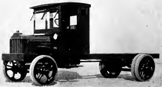
Fig. 2. A 5-ton Gasoline Truck with Front Axle and Steering Mechanism Parts Interchangeable with Those of an Electric Truck of the Same Capacity
