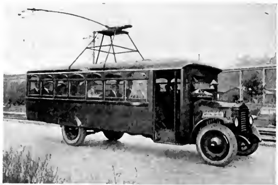
Fig. 10. Trackless Trolley Equipped with Railway Motors, Foot Control and Special Form of Collector
