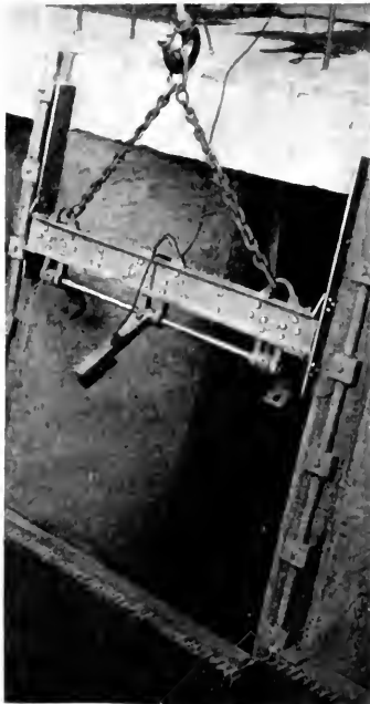
Fig. 5. This Screen Lifting Device eliminated the hazardous practice of grappling for the screen, pulling it to the water surface, and sending a man down to sling it to the crane hook
