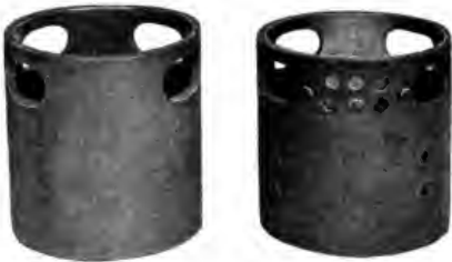
Fig. 4. Magnet Frame Constructed from Steel Plate
