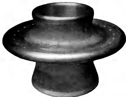
Fig. 10. Cast Aluminum Sleeve, 715-lb. Weight, for Supporting the High-voltage Terminals, Figs. 7 and 8
