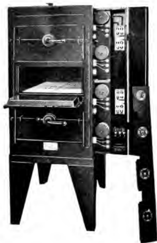
Fig. 2. 30-loaf Electric Bake Oven for Small Restaurants with Switch Panel Removed to Show Interior Switchbox Construction
