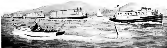
Fig. 6. Proposed Electrically Propelled Power Boat Supplying Current to Fleet of Four Barges
