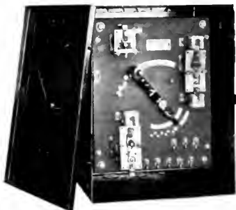
Fig. 5. Direct-current Remote-control Self-starting Speed Regulator for Blowers, Combined Armature and Field Control. Automatic self-starting type for remote operation by push buttons. Controller arm can be set for any desired predetermined speed
