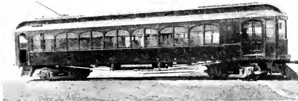
Fig. 8. Single End, 2-man, 52-passenger, 3-compartment, 36-ton Car of Kentucky Traction & Terminal Company, Replaced by 12.5-ton, 1-man Car, Shown in Fig. 6
