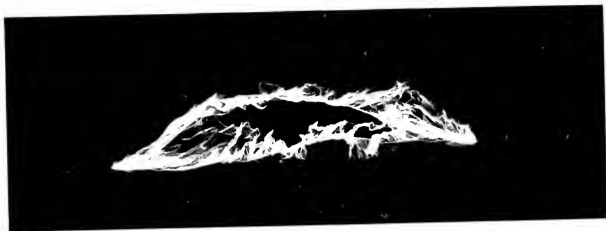
Fig. 15 Two Successive 1,200,000 volt Arcs Between Points Spaced 11 Ft. Apart
