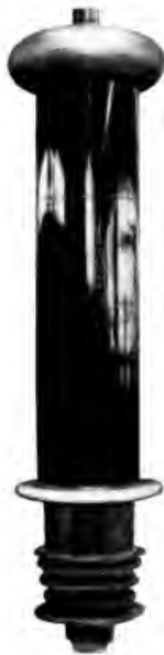
Fig. 7. Million-volt Terminal for the Line End of the Testing Set, Fig. 1
