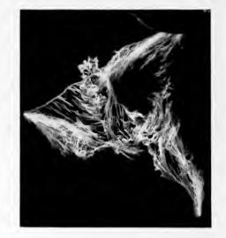
Fig. 36. Three-phase Arc Between Points 10 ft., 2 ½ in. Apart. Generator over-excited, giving arc of great volume
