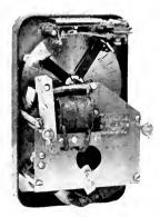
Fig. 19. Motor-operated Timer
