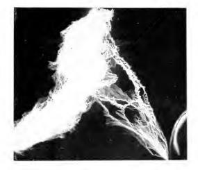
Fig. 25. Repetition of Single-phase Arcs with Y Arcs Tending to Predominate on Two Legs
