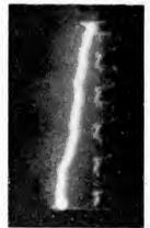
Fig. 9. Spark-over of Shielded Insulator String; single lightning stroke 1,200,000 volts, during heavy rain
