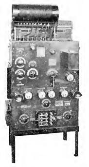
Fig. 54. Vacuum Tube Transmitter and Power Panel for use on Submarines
