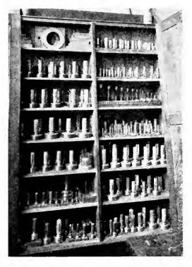
Fig. 12. Cabinet of Reference Thread Gauges
