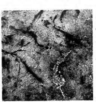
Another Close-grained Cast Iron with less graphite than No. 5 and also less phosphorous. Magnified 100 dia. Fig. 14.
