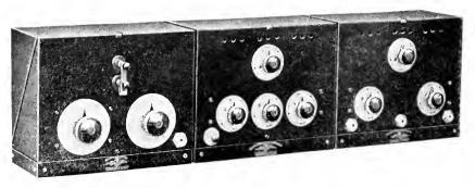
Fig. 47. Radio Receiver, Frequency Amplifier, and Detector Amplifier
