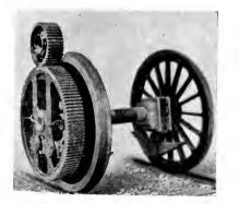
Fig. 16. Swiss Federal Railways. Outside geared drive showing location of gear and pinion with respect to the driving wheels
