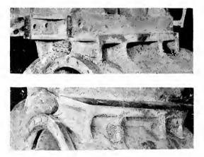
Fig. 7. Cylinder Repaired with Bare Electrodes Using 175 Amp. Quarter-inch studs were used without V-ing out the work
