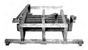
Fig. 10. Resistance Unit Removed from Its Position in the Tank as shown in Fig. 9
