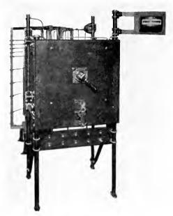
Fig. 8. Antenna Tuning Unit
