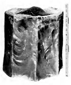
Fig. 1. Solid Ingot of Opaque Fused Quartz, Weight 115 Lb.
