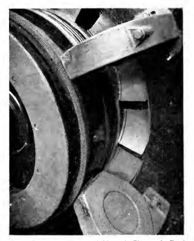
Fig. 4. Fan on Armature and Magnetic Blowout in Brushholder for Prevention of Flash-over on 4500-kw., 1500-volt B.T-H. Synchronous Converter
