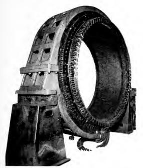
Fig. 7. Stator of the 20,000-kv-a., 257-r.p.m., 60-cycle, 11,000volt Horizontal Generator, City of San Francisco Hetch Hetchy Development
