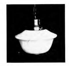
Fig. 75. A typical recent type of luminaire with globe so shaped as to direct as much light as practicable downward and upward rather than horizontally
