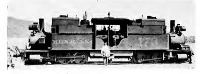
Fig. 6. Electric Locomotives will Replace this Double-ended Type of Steam Locomotive on the Mexican Railway between Mexico City and Vera Cruz
