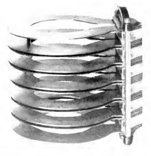
Fig. 45. Complete Low-voltage Winding of High-current Transforme
