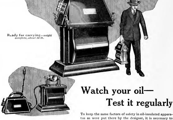
Ready for Service—The set may be supplied from lighting circuits of 110 volts, 50 to 140 cycles.
