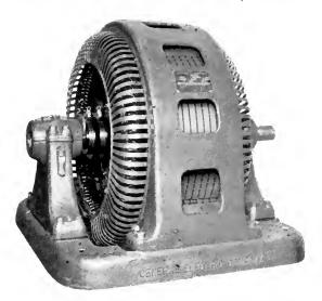
Fig. 2. Medium Capacity Synchronous Condenser, 8 poles, 1500 kv-a., 900 r.p.m., 4000-2300 volts
