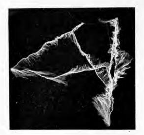
Fig. 35. Three-phase Arc Between Points 10 ft., 2½ in. Apart. Generator under-excited, giving arc of little volume
