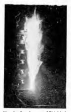
Fig. 7. Spark-over of Shielded Insulator String; dry, 60 cycles
