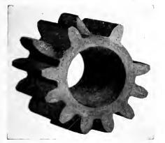
Fig. 11. Fatigue Failures of Teeth Produced by Experiment (without Radial Pressure in Bore)
