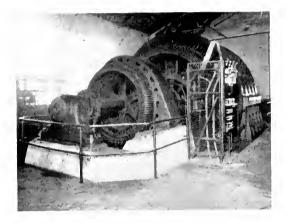
Fig. 3. Testing Generator, 26,700-kv-a., 300 r.p.m., 25 Cycles 13,200/7620/6600/3810 Volts
