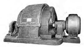
Fig. 3. Large Capacity Synchronous Condenser (12 poles, 25,000 kv-a, 600 r.p.m., 11,000 volts) with Connected Exciter and Induction Motor for Starting and Line Charging Purposes
