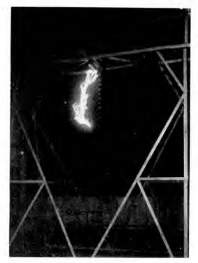
Fig. 2. Section of Full-size 220-kv. Tower Erected in the Laboratory to Study the Effect of the Tower on the Behavior of the Insulator Shield
