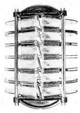
Fig. 43. Complete Low-voltage Winding of High-current Transformer
