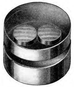
Fig. 5. Interference Bands on Two Flat Gauge Blocks That Are Being Compared for Length and Parallelism
