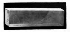
Fig. 10. Rectangular Bar of Clear Fused Quartz 4 × 1<sup>3</sup>/<sub>2</sub> × <sup>2</sup>/<sub>4</sub> in. made in Thomson Research Laboratory, General Electric Company, Lynn Works
