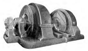
Fig. 10. A 12,000-kw. 500-r.p.m. 25/50-cycle Frequency Converter with Direct Connected Exciters and Stator Shifting Device
