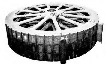
Fig. 22. Rotor Spider of 40,000-kv-a Generator for Shawinigan Engineering Company, Ltd., Canada
