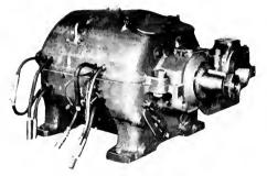
Fig. 25. A Typical Enclosed Mill-type Motor
