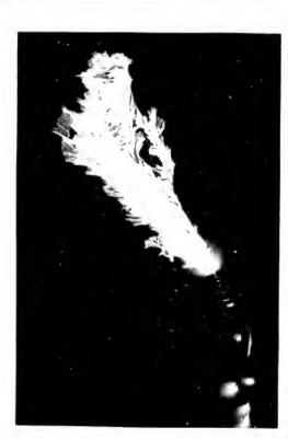
Fig. 17. Nine-foot, Million-volt Arc Photographed through a Glass Lens
