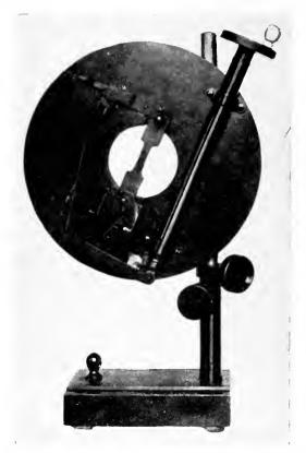
Fig. 6. Frame for Comparison Member Designed by E. G. Coker and A. L. Kimball, Jr.
