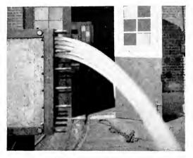
Fig. 4. Portion of One Water Box Removed to illustrate the uniformity of flow through the various tubes. This test was made to be sure there was no congestion in the water boxes
