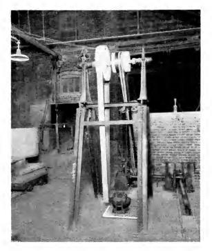
Fig. 1. Motor-driven Mechanism for Slowly Pushing Glass Melting Pots Through a Preheating Kiln
