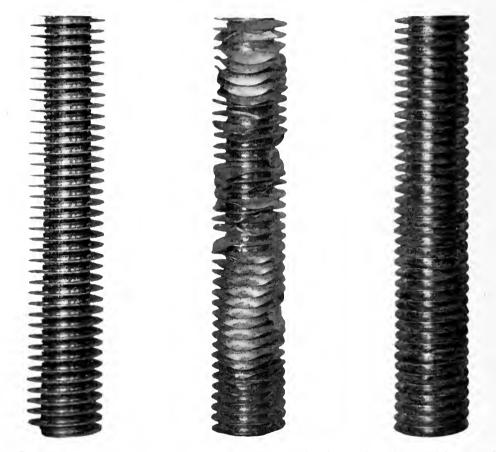
Fig. 2. To show how substantially the Fins are Attached to the Tubes, the fins of the perfect tube on the left were mutilated as shown in the center and were then trued up as shown at the right. No injured or broken joints appeared
