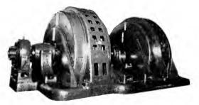
Fig. 1. A 10,000-kw. 450-r.p.m. Synchronous Type Frequency Converter Consisting of a 12,000-kv-a. 30-cycle Machine Direct Connected to a 16,000-kv-a. 60-cycle Machine. A 60-kw. direct-connected exciter is provided for each machine
