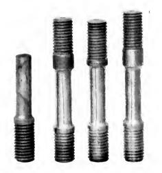
Fig. 12. Four Welded Specimens, which broke in the threads on the first two tests, turned to one-half inch diameter for the third test
