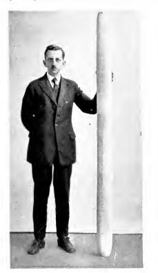
Fig. 12. Ingot of Opaque Fused Quartz weighing approximately 100 pounds. Six feet long and six inches in diameter
