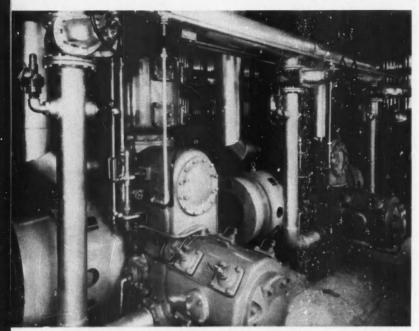
ROUND-FRAME synchronous motors are mounted directly on the frame of the air compressor; thus no special motor foundation is required during installation
