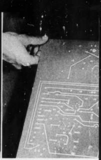
PRINTED CIRCUITS, using laminated plastics faced on one or both sides with
