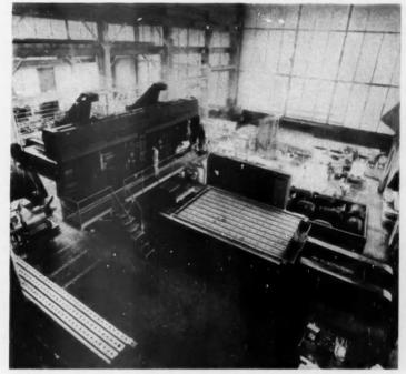
WING SECTIONS for jet planes are machined from large aluminum plates on this new "skin miller." Electric drive and control were furnished by General Electric
