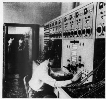
NETWORK ANALYZERS are now interconnected for solving power-system problems
