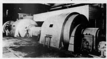
WIND TUNNELS require tremendous drives—from this 81,000-hp unit to the world's largest that will be rated 250,000 hp; 300,000 hp for one hour
