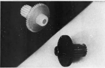
NYLON GEARS reduce cost, save critical and hard-to-get metals
