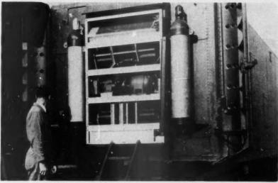
TRANSPORTABLE air conditioners for mobile laboratories and field medical units
