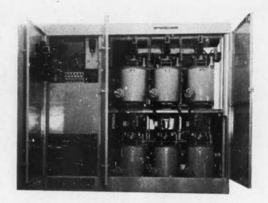
PUMPLESS IGNITRON built by General Electric to supply power pulses of 3000 amp at 2500 volts for the California Institute of Technology's particle accelerator
