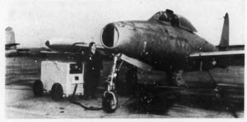
GROUND POWER PLANT provides reliable power; has capacity for heavy loads
