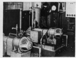
MAKE QUALITY CONTROL AUTOMATIC. Perhaps you're finding it difficult to accurately control a chemical proportion operation. Fibreboard Products, Inc. solved this problem by putting a G-E Thy-mo-trol\* Drive on a chemical pump which injects a chemical conditioner into process water as it is needed. The trick is to keep the flow of chemical accurately proportionate to the demand—no trick at all for Thy-mo-trol. Ask for Bulletin GEA-5337 on Thy-mo-trol drive.
