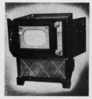
COLOR RECEIVER has flexible circuits for study of various transmission standards
