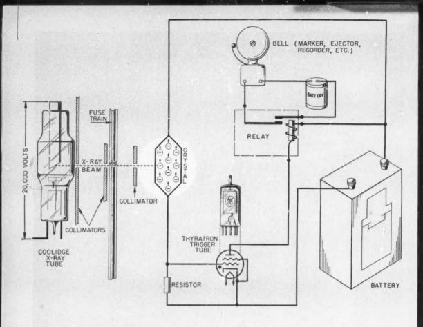
HIGH-SPEED automatic x-ray inspection of blast-fuse powder train uses new cadmium-sulfide crystal as an amplifier
