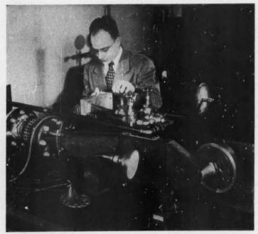
TURBINE BUCKETS are tested by closely simulating operating conditions
