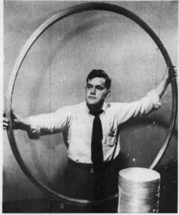
BINDING BAND is fabricated from glass fiber impregnated with polyester resin
