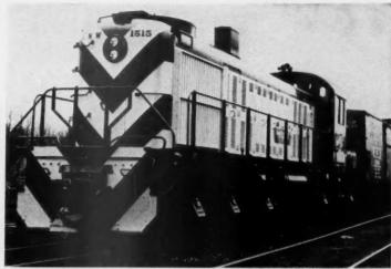
SIX-MOTOR Alco-GE road switcher for heavy-duty drag-and-transfer service
