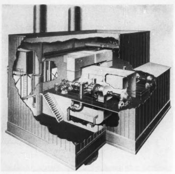
BOOSTER STATIONS on many natural gas pipelines will use General Electric gas turbines to move this high-grade fuel from the Southwest to industrial areas
