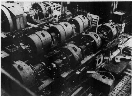
TRIPLE-ARMATURE twin drive—first of its type—on test. Complete five-stand mill will roll tinplate at 7000 feet per minute
