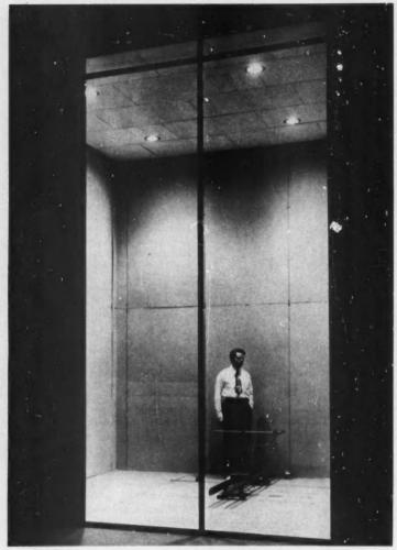
MEASUREMENTS LABORATORY with ceiling at maximum height of 16 feet and walls moved in to make room of smallest size. A complete range of room finishes is available
