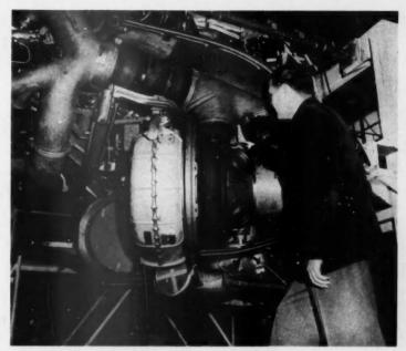
TURBOSUPERCHARGERS, such as this one on a test stand, accumulated more than one million hours of commercial air line service on Boeing Stratocruisers
