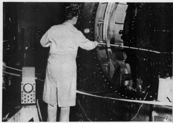
"SNIFFER" checks coils of large generator for corona. Cathode-ray oscilloscope (left) shows amplified signal from sensing element (right) if corona is detected
