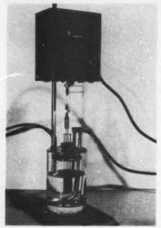
GEL TIME of polymerizable substances is determined with this new meter
