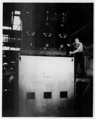
TANKING a sealed dry-type transformer rated 750 kva. Units like this are easy to handle and install; they are especially suited to industrial plants and commercial buildings
