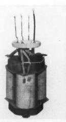
INTERNAL STRUCTURE of 15-kva 2400-volt oil-immersed wound-delta-yoke transformer characterized by compactness and symmetrical flux distribution
