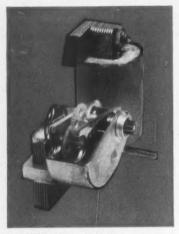
SYNCHRONOUS MOTOR and gear train, sealed within a case with oil for lubrication, are basic mechanism for timers and clocks used in home and industry
