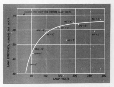
Fig. 8. LAMP OPERATING VOLTAGE vs lamp efficiency, in lumens per watt at 100 hours for standard white. For multiple-current lamps, values of %-inch diameters are 120 milliamperes and, 1-inch diameters, 200 milliamperes, for current density and brightness approximately equal to 1½-inch diameters at 425 milliamperes
