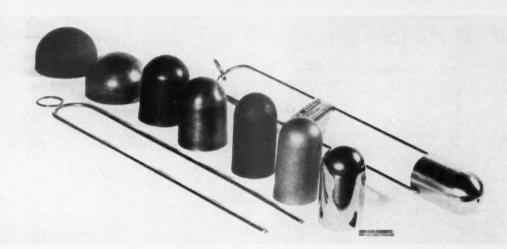
VISCOSIMETER CUPS are tumbled to remove scale after three stages of drawing and anneal and are finished by tumble burnishing; stainless steel bail and ring are also finished and burnished by tumbling
