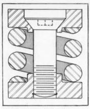
INDIVIDUAL SPRING in cross section, showing method of compression. Springs like this support the stationary member of the thrust bearing
