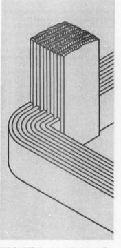
DESIGN DETAIL—A simplified sketch illustrating the arrangement of layers in the junction of core materials in yoke to the vertical punchings in the core legs
