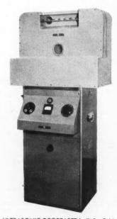
ULTRASONIC DEGREASER built for Schick Inc. with conveyor equipment and tank for cleaning solution surmounting the generator
