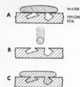
Fig. 5. MECHANICAL ADHESION between ice and Teflon foil. (A) A water droplet rests and freezes on the Teflon surface without penetrating the surface irregularities; (B) a droplet strikes the surface at high speed; and (C) is forced into the irregularities, where it freezes
