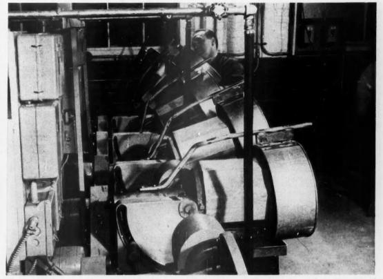
SMALL BARRELS designed for flexibility in tumbling activity permit variation in mechanical conditions because they can be positioned to obtain most efficient deburring and polishing actions
