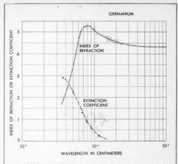
Fig. 6. OPTICAL PROPERTIES of germanium films, Region of greatest photoelectric sensitivity is between high absorption and low absorption (1.0 to 2.0 microns)
