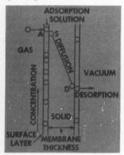
The gas hits the surface and is absorbed at A as a surface layer. With high gas pressures this may be more than monomolecular. Then the gas dissolves in the body of the solid at S. Because there is a vacuum on the other side, the dissolved material diffuses down the concentration gradient to D on the low-
