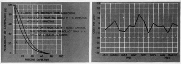
FIG. 3. OPERATING CHARACTERISTICS OF SAMPLING PLANS
