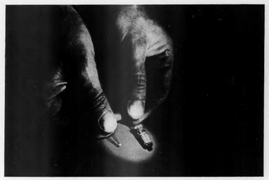
AMPLIFICATION PROPERTIES AND SMALL POWER REQUIREMENTS OF TRANSISTORS MAKE THEM A NATURAL FOR USE IN MANY ELECTRONIC DEVICES
