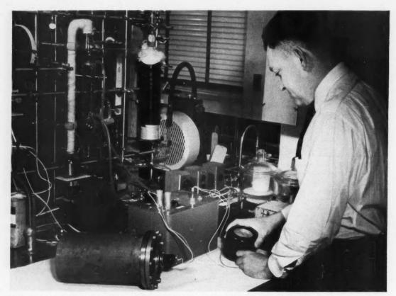
AUTHOR WITH ION CHAMBER OF THE TYPE THAT PROMISES SUPERIOR RESULTS FOR RADIOCARBON MEASUREMENTS. IT'S A MEANS OF ...
