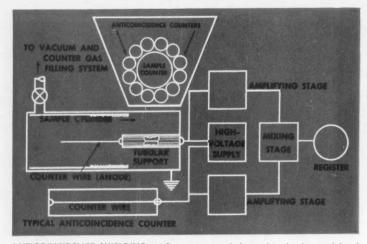
ANTICOINCIDENCE SHIELDING on Geiger counter helps reduce background level. To count background the sample cylinder is slid in the direction of the arrow so that the bare portion of the sample cylinder surrounds the counter wire
