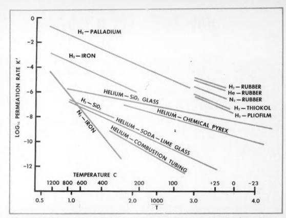
RATE OF PERMEATION of gas through solids. Units for permeation constant K' are cubic centimeter of gas (at normal temperature and pressure)per second per square centimeter of area per millimeter thickness per one atmosphere partial pressure difference
