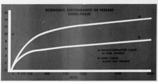
FIG. 1. SMALL INCREASE IN PERFORMANCE CAPABILITY P OF CABLE SIZES 1000 MCM AND UP DOES NOT JUSTIFY ADDITIONAL COST
