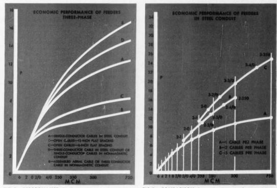
FIG. 2. PERFORMANCE of self-supporting aerial cable is particularly noteworthy. Curve A is same as shown in Fig. 1 above
