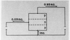
FIG. 4. JUNCTION TRANSISTOR UTILIZES SMALL BASE CURRENT
