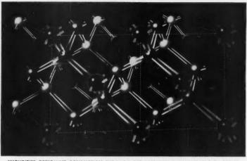
IMPURITIES DETERMINE CONDUCTION THROUGH GERMANIUM'S DIAMOND CUBIC LATTICE
