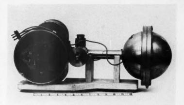
**IONIZATION CHAMBER**, of the type used for cosmic-ray study, was used by researchers for measuring low-level radiation. Spherical chamber is at right, recording camera is at left. This equipment was a forerunner of the type shown on page 20
