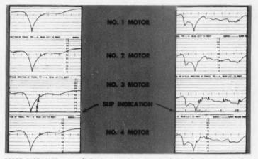
SPEED-DISTANCE curves (left) show simultaneous wheel slip of all motored axles. Curves at right show sustained wheel slip on slippery rails
