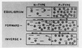
FIG. 1. P-N JUNCTION IN GERMANIUM CRYSTAL IS A RECTIFIER
