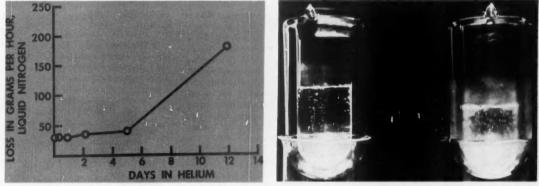
RATE OF LOSS OF LIQUID NITROGEN FROM DEWAR VACUUM FLASK
