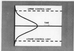
FIG. 1. BELL-SHAPED DISTRIBUTION OF 100 MEASUREMENTS
