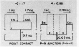
FIG. 2. TRANSISTOR COMPRISES TWO ADJACENT P-N JUNCTIONS
