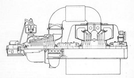
1800 rpm and carries remainder of 160,000-kw load. Advan- use of smaller size generators, and lower initial cost
