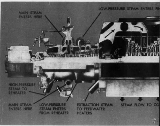
FIRST MODERN REHEAT UNIT BUILT IN THE POSTWAR PERIOD IS A TANDEM-COMPOUND UNIT WITH A DOUBLE-FLOW LOW-PRESSURE ELEMEN
