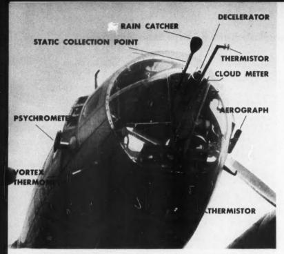
FLIGHT INSTRUMENTS mounted in the nose of a Project Cirrus B-17 include: static collection point to measure variations in the electrical potential of the atmosphere, a rain catcher to give average value of the precipitation in the air for approximately each 1000 feet of flight, and a decelerator to slow down the air and assist in sorting out rain, snow, dust, or cloud particles from the atmosphere as the plane passes through.
