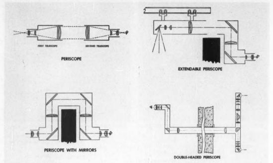
made *unsymmetrical*. If, for example, you use a periscope objective with four times the eyepiece's focal length, the instrument magnifies four times.
