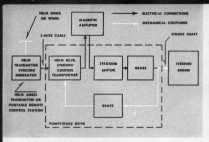
FIVE-WIRE CABLE that transmits helm order information is the only connection between the control station and steering engine located in the stern of the ship
