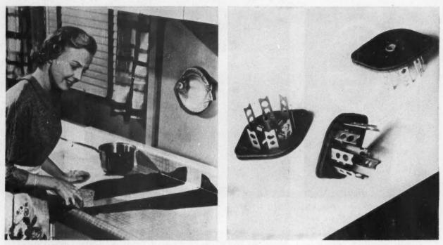
HIGH-PRESSURE LAMINATED PLASTICS MATERIALS ARE EQUALLY AT HOME IN KITCHEN OR AS HIGH-FREQUENCY CIRCUIT INSULATION
