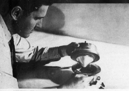
MERCURY JET SWITCH monitors 48 thermocouples at a rate of 480 per second. It is able to expand to scan additional couples at the same rate
