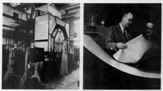
PAPER MACHINE (ABOVE) MAKES MICA MAT IN CONTINUOUS LENGTHS FOR INSULATION IN VARIOUS TYPES OF ELECTRICAL APPARATUS
