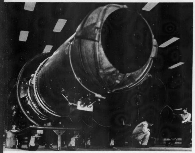
... THESE GENERAL ELECTRIC TURBOJET ENGINES WITH AFTERBURNERS WHERE ADDITIONAL FUEL IS BURNED FOR THRUST AUGMENTATION
