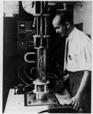
GERMANIUM DIODE with water-cooling unit. Current through germanium wafer exceeds that recommended for a copper con-
