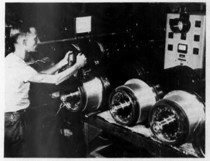
WINDING INSULATION TESTER IS USED ON TRANSPORTATION MOTOR PRODUCTION LINE
