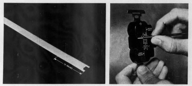
ELECTRIC RADIANT HEATING PANELS (ABOVE) ARE FINDING NEW USES, WHILE A PRESSURE-LOCK TERMINAL SPEEDS CONNECTIONS
