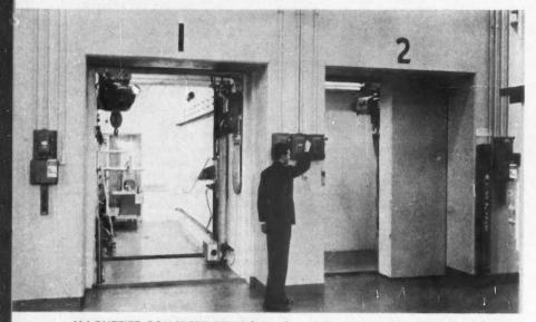
MAGNETITE CONCRETE CELLS (above) provide protection during testing of radioactive materials in the KAPL Laboratory. Control face of a cell (below) for handling radioactive materials contains electrical, mechanical, and hydraulic controls
