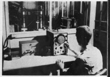
combines simplicity and high inherent stability for making corona studies of insulation under a series of voltage stresses
