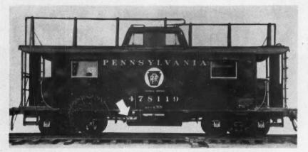
AXLE-DRIVEN ALTERNATOR (ARROW) FURNISHES POWER FOR CABOOSE EQUIPMENT
