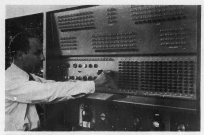
SEVEN THOUSAND germanium diodes are used in this digital computer. It has the largest "memory" yet incorporated in any computing device. Control center is shown
