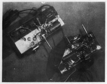
DIP-SOLDERED RADIO CHASSIS ON LEFT COMPARED WITH HAND-SOLDERED COUNTERPART
