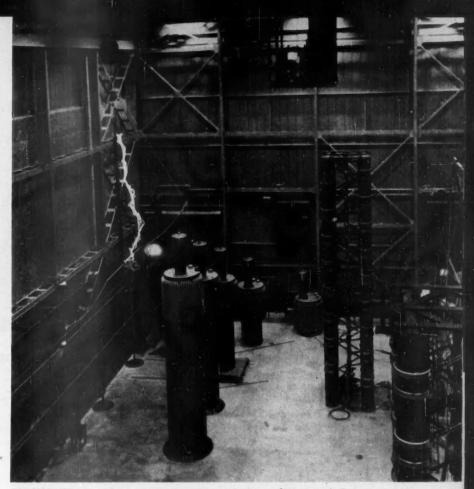
FLASHOVER on a 30-unit string of suspension insulators (*left center*). The new equipment at the high-voltage laboratory obtains data at spacings up to 20 feet
