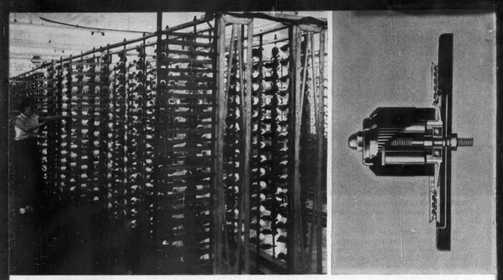
WARPING CREEL of the magazine type is equipped with hysteresis brakes that use permanent magnets to control torque
