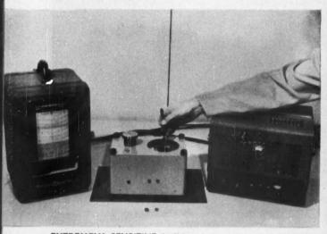
EXTREMELY SENSITIVE ball-bearing torque tester indicates presence of faults in tiny bearings that other techniques do not
