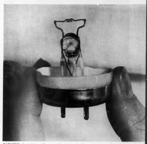
**CATHODE** of rapid-start fluorescent lamp requires less energy to preheat. More life for its size is given than for any cathode that was previously used
