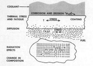
**JACKETING OF URANIUM** in a nuclear reactor is necessary to prevent corrosion by the coolant. Thermal stresses and interdiffusion are other important problems.
