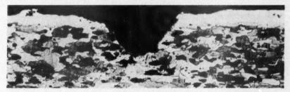
FIG. 9. This is the cross section of an alclad 17S-T4 (-T) sheet (0.040 inch thick) showing electrolytic protection of the core which was exposed by a deep scratch. No corrosion of the core occurred during six years' exposure to the atmosphere at New Kensington, Pa. Note sacrificial attack of coating adjacent to the scratch. (This cross section is enlarged 100 times and the sample was etched with HF-HCL-HNO<sub>a</sub>.)
