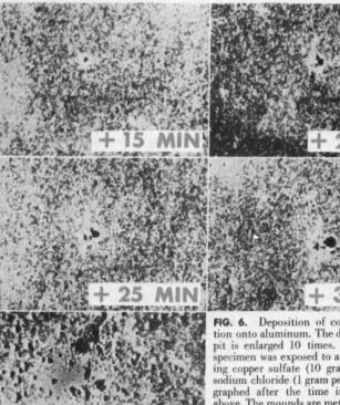
FIG. 6. Deposition of copper out of solution onto aluminum. The development of the pit is enlarged 10 times. An aluminum 2S specimen was exposed to a solution containing copper sulfate (10 grams per liter) and sodium chloride (1 gram per liter) and photographed after the time intervals indicated above. The mounds are metallic copper, while the dark spot near the center of each picture is the corrosion pit. This is further covered under the discussion of *CASE II* on page 16.
