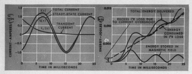
FIGS. 4 AND 5. INSTANTANEOUS CURRENT AND ENERGY COMPONENTS IN A SINGLE-PHASE RL CIRCUIT WITH 0.5 POWER FACTOR AT 60 CYCLES.
