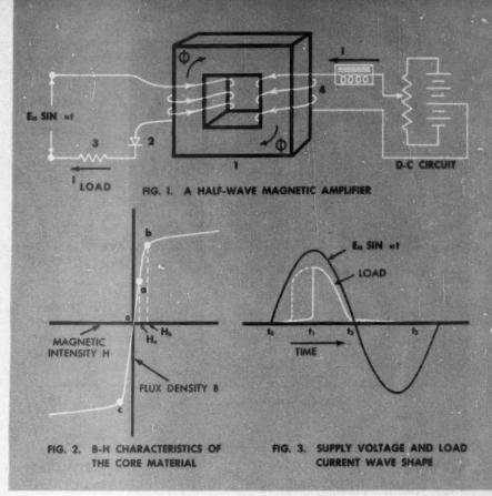
of a high inductance makes the amplifier's speed of response slow—the use of a high resistance reduces the amplifier's gain.
