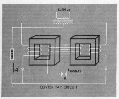
PRACTICAL MAGNETIC AMPLIFIER HAS TWO HALF-WAVE CIRCUITS, ONE SIGNAL.
