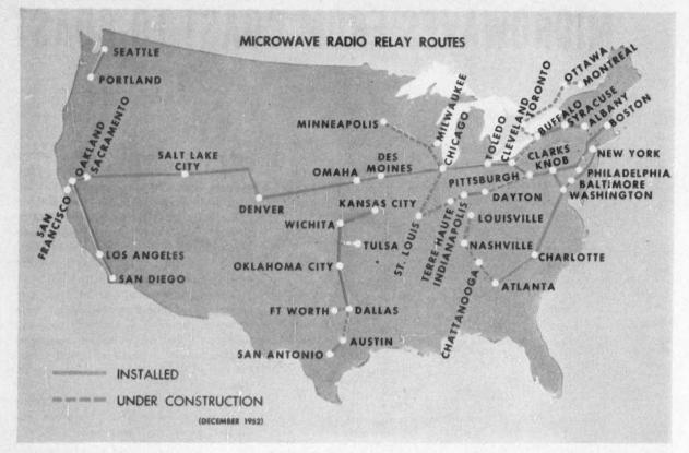
under construction or in the planning stages. The routes in operation provide 36,000 miles of broad band radio channels that are utilized to furnish 17,000 miles of television circuits and about one million miles of two-way telephone trunks.
