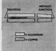
FIG. 8. Film of electrolyte between aluminum and copper in metallic contact. Note that the metallic contact can be at a considerable distance from the site of corrosion. This situation differs from others because no copper need be deposited on the aluminum. *CASE III* on page 16 describes this.
