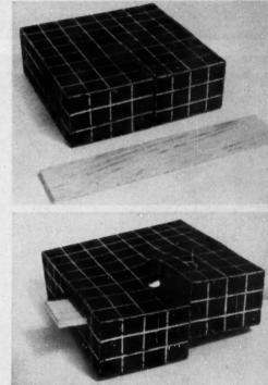
**SCREW DISLOCATION** demonstrated with a rubber model of a crystal (*top*). When dislocation is present (*bottom*), it offsets the crystal one atomic spacing, thereby converting the crystal's separate atomic planes into a spiral ramp or screw.
