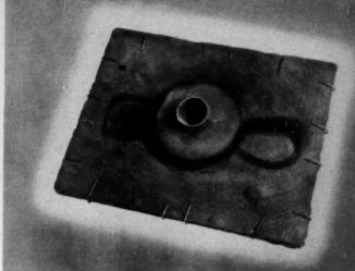
6 The ejected shell's upper and lower halves are next assembled to form the mold. Halves can be bolted together with speed nuts, held by spring clamps, set in mechanical jigs, or stapled. Adhesives in the cold state—or the resin itself in the hot state—can be used to join them. Here the propeller mold is fastened together with ordinary wire staples. On the next page you'll see how ...
