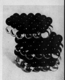
**SINGLE CRYSTALS** before and after testing. Reason why most materials are weaker than they should be is now traced to defects within the individual crystal.
