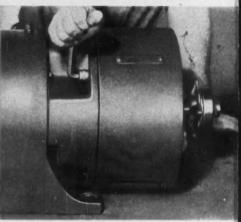
**UNBOLT STATOR FRAME BOLTS.** Adapter located between motor frame and gear housing gives easy access to stator frame bolts. Note: no special tools are needed.
