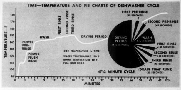
HEAT LOSS OF 150 F WATER SUPPLY TO DISHES AND TUB IS GRADUALLY COMPENSATED FOR BY A BUILT-IN HEATING UNIT.
