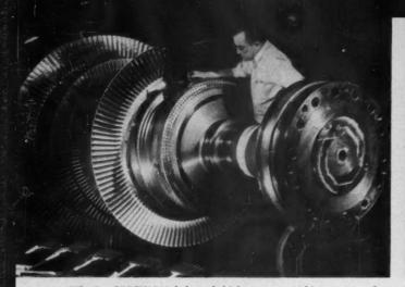
FIG. 8. PRECISION balanced high-pressure turbine rotor—after more machining the rotor will be test run in the turbine casing.
