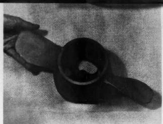
8 The finished product is removed from the pouring flask and cleaned. Practical effect of the propeller's smooth finish is to reduce the number of subsequent machining operations. For mass production, the last two operations—pouring metal, removing and cleaning cast product—are performed automatically. By the shell-molding process, almost any metal can be cast to close tolerances.
