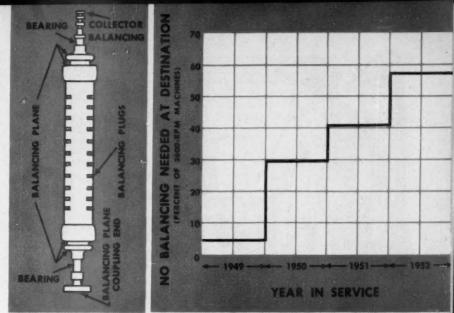
FIG. 12. VARIOUS positions FIG. 13. PRACTICAL EFFECT of precision balancing at accessible on generator rotor factory. During 1952, 58 percent of all turbine-generators for balance weight corrections. shipped needed no further balancing at destination.
