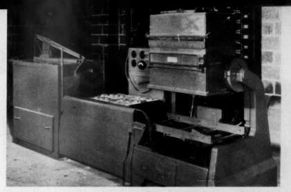
SINGLE-PATTERN MACHINE of the type used to turn out shells for preceding pictures. Left to right are oven, ejection station, and investment box. Equipment takes little space.
