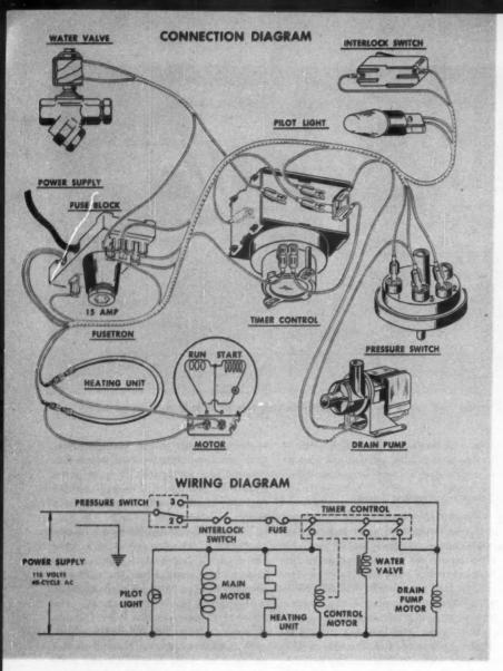
**FLOODING** of dishwasher at any time is prevented by water-actuated pressure switch. Note in wiring diagram that switch is connected ahead of control circuit's fuse.
