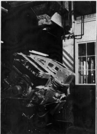
3 The hot pattern wheels along on its carriage to the investment box and clamps in place onto the bottom. Formation of the shell mold begins when the curved louver that supports the sandresin mix—supplied from the chute above—swings upward, dumping and spreading mix onto the hot pattern. Now begins a heat transfer process that determines how thick the shell will be, for...
