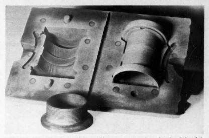
**SHELL-CORE PROCESS** eliminated four machining operations from this threaded nickelsilver plumbing fixture. Here, molten metal is poured with the mold in upright position.
