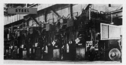
AMPLIDYNE CONTROL—In the steel industry the amplidyne controls motors and generators representing hundreds of thousands of horsepower. One tandem coldreduction mill—with a total of over 22,000 horsepower—utilizes 34 amplidynes to carry out the mill operator's commands. Only 10 seconds are needed to accelerate the steel strip from a dead stop to 80 mph. Mill speeds have increased to this figure from less than 9 mph 20 years ago.
