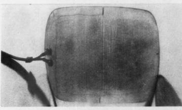
THERMOPLASTIC LENS IS ELECTRICALLY HEATED TO DEFROST AIRCREW GOGGLES.
