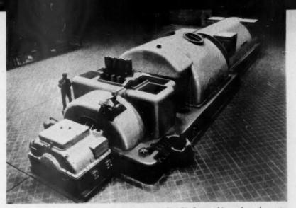
**MODERN** steam turbine-generator set rated 80,000 kw. Similar machines of much greater capacity and efficiency will shoulder the major portion of future power expansion.
