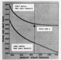
IMPROVED STATION EFFICIENCY is obtained through increasing temperature and pressure, as boldly done for Philo Unit No. 6. Studies indicate that for any further significant increases, considerably higher initial and reheat temperatures will be required to take advantage of pressures higher than 4500 psig. new and forward-reaching technological ideas that will contribute to an expected over-all plant thermal efficiency of more than 40%.
