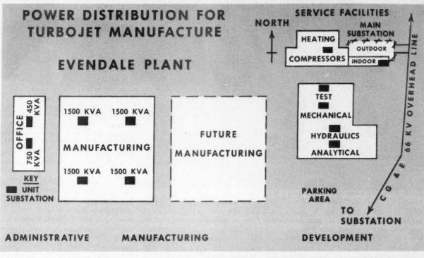
ARRANGEMENT OF FACILITIES FOR GENERAL ELECTRIC'S NEW JET ENGINE CENTER AT EVENDALE, OHIO, USED AS THE MODEL IN A ...
