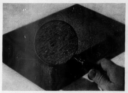
AIR POCKETS enclosed by solid resin films make up the expanded phenolic foam. About two-thirds of these air pockets are independent cells—the others are interconnected.
