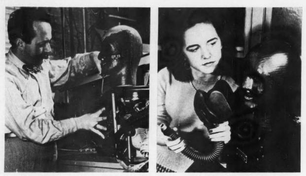
HEAD THAT BREATHES IS WIRED TO SIMULATE HUMAN SKIN TEMPERATURES; COMPLETE WITH ITS FINAL LATEX COATING (RIGHT).
