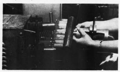
**FABRICATION** of junction transistors weighing 0.05 ounces nears final stage as exhaust tubes are pinched off and vent welded. New manufacturing methods cut their cost in half.
