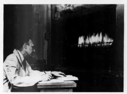
CONTROL CABLE WITH SILICONE INSULATION UNDERGOES A 24-HOUR TEST AT 1400 F.
