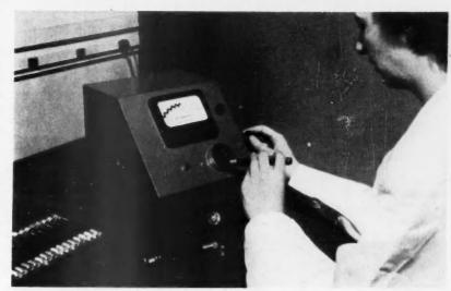
ELECTROMETER READS RADIATION DOSAGE OF POCKET-TYPE IONIZATION CHAMBER.
