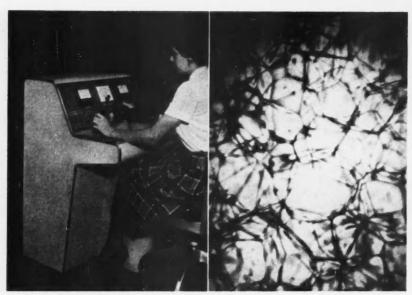
**X-RAY MICROSCOPE** (*left*) photographs details of specimens normally opaque to light. X-ray micrograph shows grain structure of an aluminum-tin alloy magnified 100 times.
