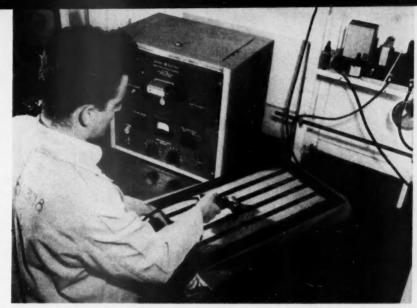
**ELECTRICAL FAULT TESTER** reduces manufacturing losses by providing improved control of the quality of capacitor paper during production. It is also a valuable laboratory tool.
