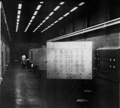
RADIOMETALLURGY LABORATORY contains three multicurie cells for study of materials with intermediate radioactivity plus a fourth cell for highly radioactive substances.
