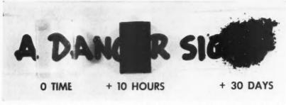
EXPERIMENT SHOWS DAMAGE TO LITHIUM FLUORIDE RESULTING FROM RADIATION EXPOSURE.
