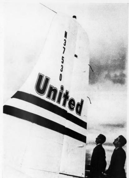
HIGH-INTENSITY BEACON mounted on the vertical fin of an airliner increases air safety. A fixture rotates the beam horizontally making it visible from all points of the compass.
