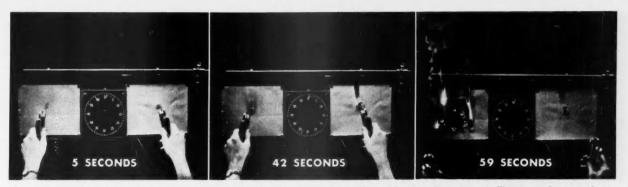
**HOT FLAMES** of identical alcohol torches are applied to conventional silicone rubber and special flame-retardant silicone rubber. Samples tinguishes self while conventional rubber continues burning (*right*).
