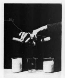
**SILICONE FLUID** pours at -100 F (*right*) while standard petroleum fluid freezes over.
