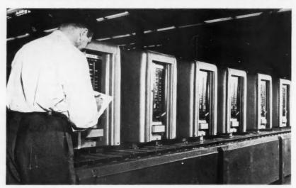
LONG-LIFE A-C TRANSFORMER WELDERS ARE EASILY OPERATED AND HIGHLY DEPENDABLE.
