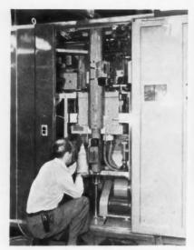
**CERAMIC-COATED TETRODE** is used with a 50-kw amplifier for high-channel VHF.
