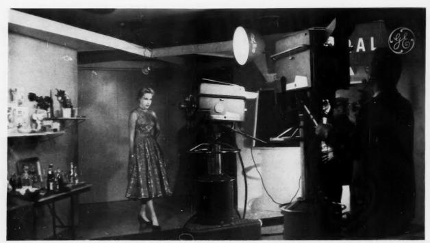
FIELD-SEQUENTIAL COLOR-TV CAMERA USED WITH A CHROMACODER IS LIGHT AND EASILY HANDLED AND TRANSMITS A COMPATIBLE SIGNAL.
