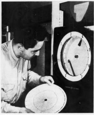
**CENTERLESS POINTER** of process-instrumentation recorder increases readability, retains high accuracy, and simplifies chart changing.
