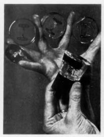
RECEIVING TUBES filled with clear plastics are sliced for microscopic examination.
