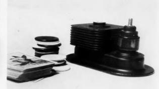
**MINIATURE** germanium power rectifiers range in operation to 400-amp output and have efficiencies approaching 100 percent.
