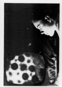
**FIELD-EMISSION MICROSCOPE** aids crystalchange and adsorption-phenomena study.
