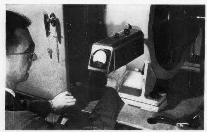
PORTABLE VIBRATION METER MEASURES UP TO 300-MIL DISPLACEMENTS AT 250 CPS.
