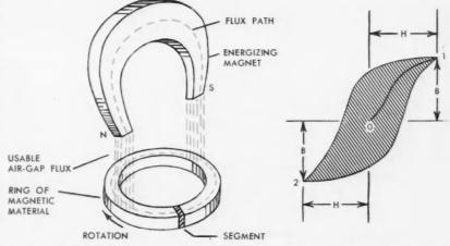
**PRINCIPLE UNDERLYING** a hysteresis torque device is continuous tracing and retracing of the magnetic material's hysteresis loop. Repulsive force is independent of speed.
