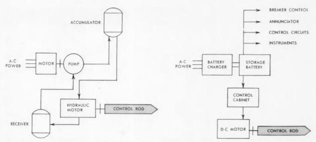
**HORIZONTAL PENETRATION** of a nuclear reactor can be accomplished by one of two systems, both utilizing the force of gravity:
