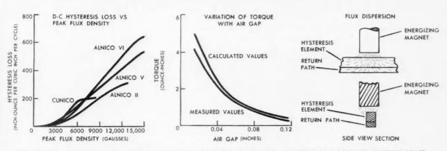
FLUX DENSITY, LENGTH OF AIR GAP, AND FLUX DISPERSION ARE FACTORS THAT DETERMINE TORQUE OF A ROTATING HYSTERESIS DEVICE.
