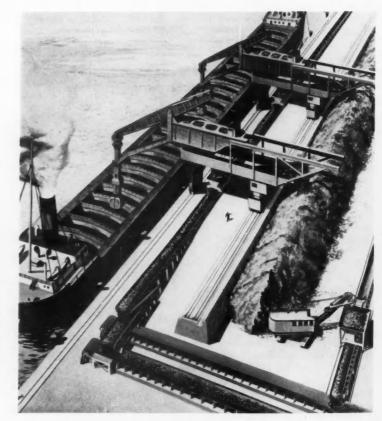
**EARLY CONCEPTION** of Riverlake: Hulett-type unloaders at new dock facilities on Lake Erie at Cleveland would unload ore vessels at high speed (*left*); mainline conveyor resembling a huge steel tube would simultaneously transfer coal and ore from one flight to the next (*center*); coal unloaders at river terminal would unload the barges.
