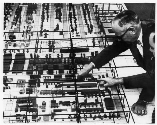
EQUIPMENT MODELS DISPLAYED IN LAYOUT OF A NEW MANUFACTURING PLANT AT BLOOMINGTON, ILL., ARE POSITIONED BY AUTHOR.
