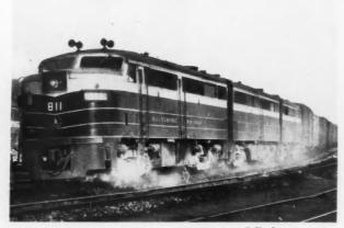
EACH CAB of New Haven Railroad's fleet of 4000-hp passenger THREE-UNIT 4800-HP DIESEL ELECTRIC, using G-E electric equipment, typifies today's freight and passenger locomotives.
