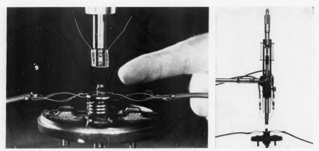
PRESSURE OF THE WIRE-LOOP PROBE ON A CONTACT BUTTON IS INCREASED IN CONTROLLED INCREMENTS WITH A MICROMETER HEAD (RIGHT).
