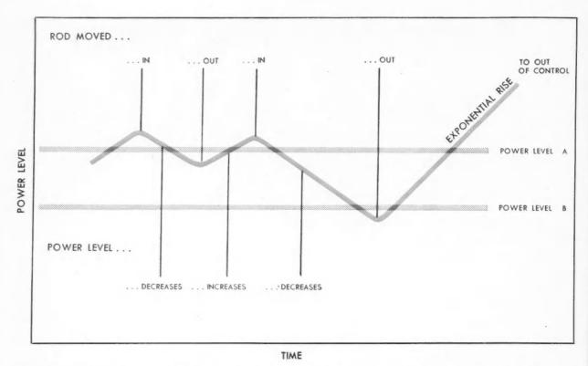
NUCLEAR REACTORS can be controlled by inserting rod-like sults in more neutrons and increased reactor power; insertion of the rod causes fewer neutrons and, consequently, decreased power.
