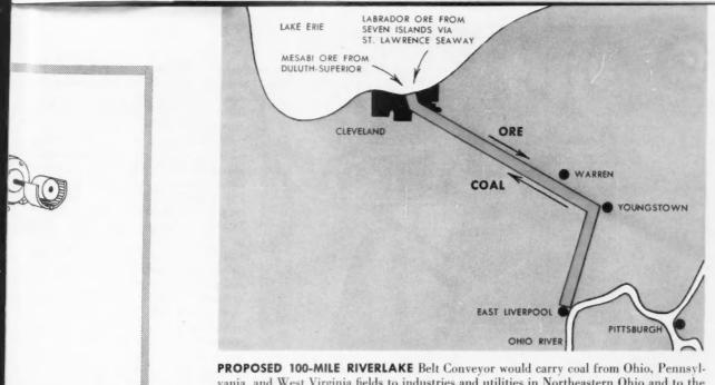
**PROPOSED 100-MILE RIVERLAKE** Belt Conveyor would carry coal from Ohio, Pennsylvania, and West Virginia fields to industries and utilities in Northeastern Ohio and to the lake terminal for shipment to other industrial areas. It would also transport ore from lake vessels to the river terminal for shipment via barges to steel plants in the three states.
