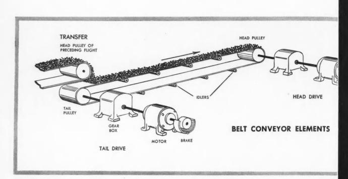
**BELT**—primary element in a belt conveyor—has rubber covering to protect the cotton duck, nylon, or steelcable core from abrasion and weather. Idlers, pulleys, power drives, and supporting structure form the supplementary parts. Combined with others, one belt becomes a flight in a long-distance conveyor like the Riverlake proposal.
