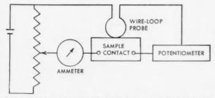
ELECTRIC CIRCUIT MEASURES CONTACT RESISTANCE OF SURFACE FILM.
