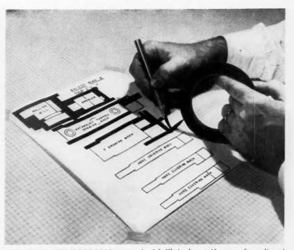
**ONE-FOURTH-INCH BLACK TAPE** or opaquing ink fills in the outside areas of complicated outlines so that the template can be easily cut out when reproduced.
