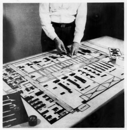
**DOUBLE-COATED SELF-ADHERING TAPE** holds the outline, or template, to the transparent floor layout. All lettering not in the template is similarly handled.
