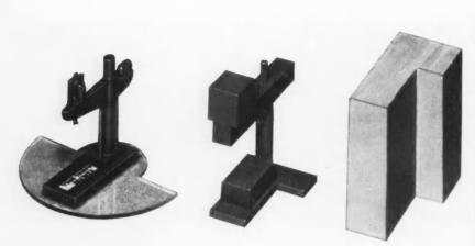
**VARYING DEGREES OF DETAIL** of a radial drill model show that a good three-dimensional model (*center*) must be recognizable yet easily fabricated and simply detailed.
