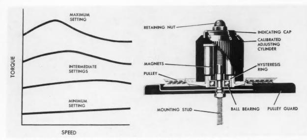
SPEED-TORQUE CURVES INDICATE EDDY-CURRENT EFFECT (LEFT); COMPONENTS OF YARN-TENSION BRAKE ARE ARRANGED AS IN CUTAWAY.
