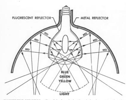
FLUORESCENT REFLECTOR utilizes light from both sides of phosphor coating that also reflects light from the arc, and it provides five percent more output than nonreflector lamps.
