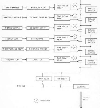
A CONTROL-ROD CIRCUIT consists of a number of sentinels that monitor certain conditions and properties, reporting to a series circuit that controls a set of trip relays.
