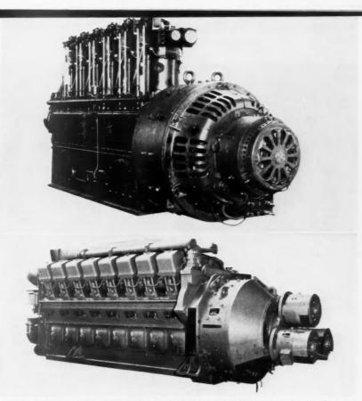
**ENGINE AND GENERATOR DESIGN** of today's 16-cylinder V-type 2250-hp diesel engine (*lower*) contrasts sharply with early 6-cylinder 300-hp engine, showing 30 years of progress.
