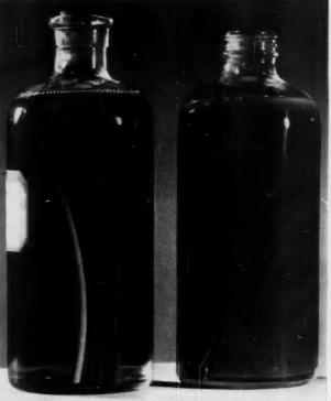
PLASTICS REMAINS FLEXIBLE IN OIL; RUBBER DISINTEGRATES.
