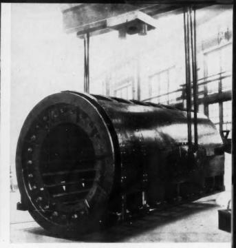
**ADVANCED WELDING TECHNIQUES** permitted the fabrication of large generator stator frames (left), replacing cumbersome struc-
