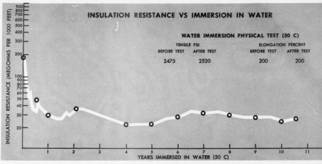
INSULATION RESISTANCE OF PLASTICS WIRE REMAINS STABLE AND HAS AN ADEQUATE MARGIN OF SAFETY AFTER HIGHLY ACCELERATED TEST.
