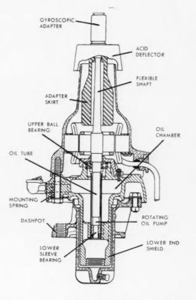
by oil pumped up the inside of the oil tube surrounding the shaft—the pumping action obtained by a rotating shoulder on the shaft.
