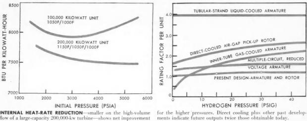
INTERNAL HEAT-RATE REDUCTION-smaller on the high-volume flow of a large-capacity 200,000-kw turbine-shows net improvement
