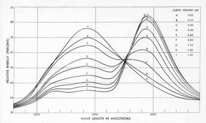
FOR STANDARDIZED LIGHT, PRECISE AMOUNTS OF MANGANESE ARE ADDED TO CALCIUM-PHOSPHATE PHOSPHOR, REGULATING LUMEN OUTPUT.
