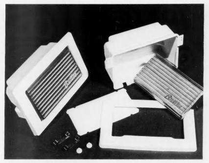
**REFRIGERATOR BUTTER CONDITIONER**, molded from styrene material, contains two pinions, housing, and bezel cemented together to make one unit; baffle plate snaps into place.
