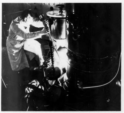
**STANDING ATOP HEAT,** operator checks molten metal in the new 1000-pound vacuummelting furnace located just beneath him where temperatures range from 2800 to 3200 F.
