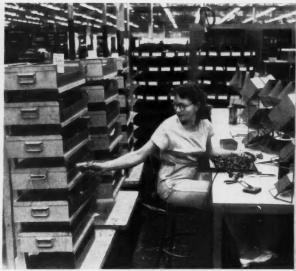
4 At each work station, the operator not only gets the right parts at the right time but also has all parts for the order only an arm's length away. There is no chasing around the plant for missing parts.
