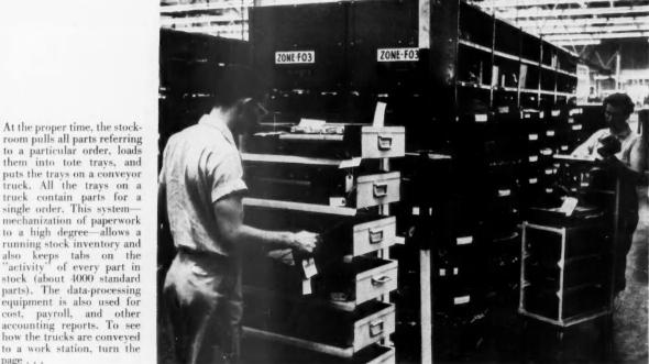
them into tote travs, and puts the trays on a conveyor truck. All the trays on a truck contain parts for a single order. This systemmechanization of paperwork to a high degree-allows a running stock inventory and also keeps tabs on the "activity" of every part in stock (about 4000 standard parts). The data-processing equipment is also used for cost, payroll, and other accounting reports. To see how the trucks are conveyed to a work station, turn the page . . .
