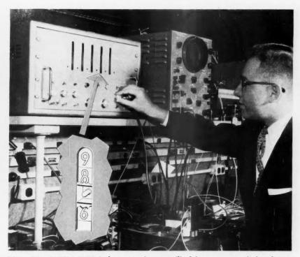
TINY NEON GLOW LAMPS in large quantity are utilized in events-per-unit-time instruments and other counters of various types. Simplified design in inset shows lamp mounting.
