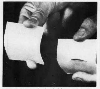
**IMMERSED** under stress in a household detergent solution, irradiated polyethylene (left) shows outstanding stress-cracking resistance.
