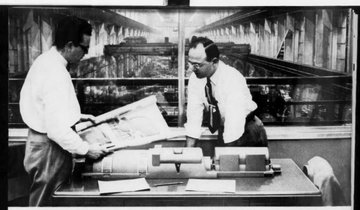
**LARGEST TURBINE STEAM FLOW** to date, 2,700,000 pounds per hour, will be one of many advances in the General Electric turbine-generator units for the Linden station. The
