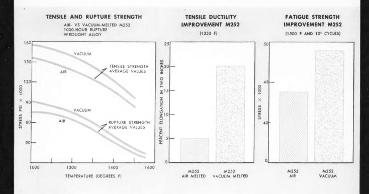
VACUUM MELTING SO ENHANCES PROPERTIES OF M-252 ALLOY THAT IT IS WELL SUITED TO A VARIETY OF HIGH-TEMPERATURE APPLICATIONS.
