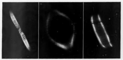
**RADIO-PANEL LAMP** synchronizes filament and lead-in wire resonant frequency (right) vibration formerly moved filament in one direction (left), lead-in wires in another (center).
