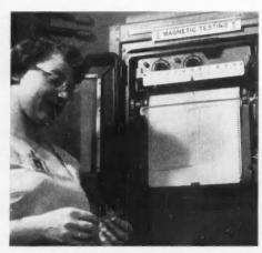
**AUTOMATIC RECORDER** speeds search for new and improved magnetic materials. Direct current is switched on (right) from two germanium rectifiers with a capacity of 12,000 amp at 15 volts.  $\Omega$
