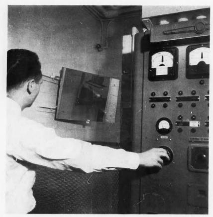
ONE-MILLION-VOLT ELECTRON BEAM IRRADIATES MOVING POLYETHYLENE FILM TO PRODUCE ...
