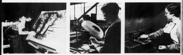
SKILLED HANDS ASSEMBLE WIRING HARNESSES AND MICROMINIATURE RELAYS; DIP-SOLDERING IS USED ON SOME CONTROL COMPONENTS.
