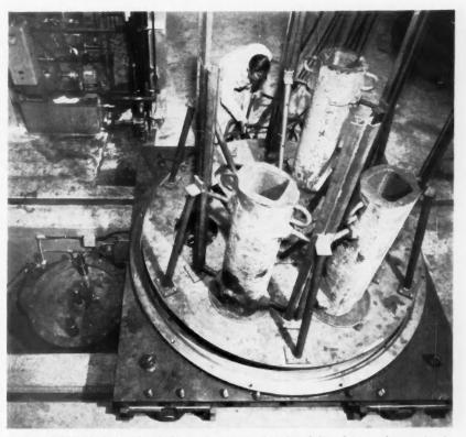
**MOLD CHAMBER** designed to hold up to six ingots is indexed directly over the opening in the turntable so that the lift (lower left) can push the molds up into pouring position.
