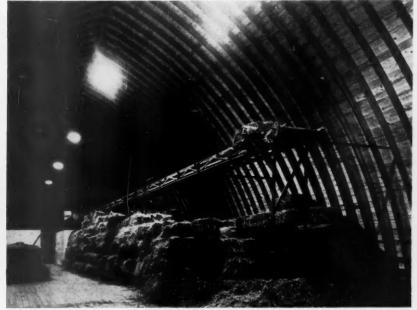
peanuts, and corn can be harvested damp and dried electrically in this equipment.
