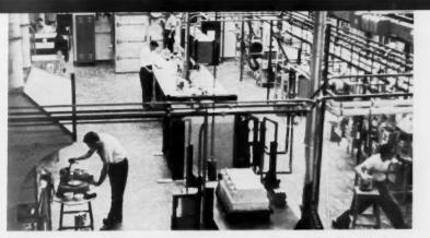
**EQUIPMENT** to meet all foreseeable future requirements is at the disposal of ceramists in the Metals and Ceramics Building. In this area, ceramic materials are melted and heat-treated; they are formulated, mixed, and pressed in adjacent rooms.
