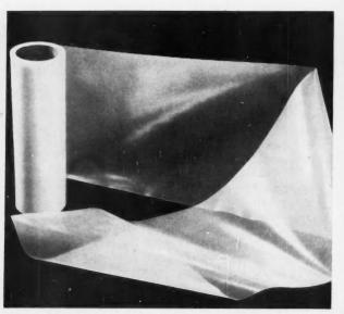
**ROLL** of 12-inch-wide irradiated polyethylene film—an ideal largevolume application of irradiation—will be slit into insulating tapes.
