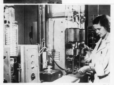
**CARBON CONTENT** of a metal is quickly analyzed in chemical laboratory. With this information, metallurgist can accurately control melting process.
