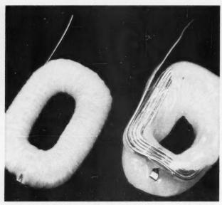
**NONMELTING** at 150 C, irradiated polyethylene permits insulation of motor-starting coils. Conventional polyethylene melts away.
