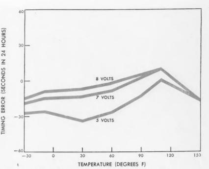
**TEMPERATURE-COMPENSATING** characteristics of the Motochron's hairspring assure accurate timekeeping over a wide temperature range, matching the motor's torque characteristics.
