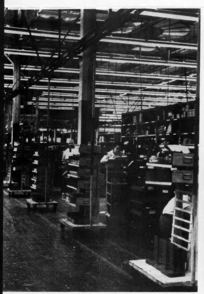
**3** Three conveyor systems carry parts from stockrooms to various product-assembly areas throughout the plant. The trucks are disengaged easily from the conveyor at the appropriate work station. No traffic problems and a clean plant layout are two results.
