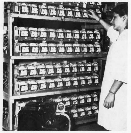
**EACH MOTOCHRON CLOCK** undergoes a timekeeping test. The impulses of the clock's escapement are picked up by a microphone and then amplified and recorded for observation.
