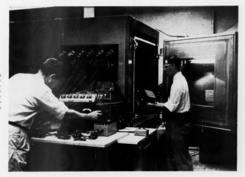
AIRCRAFT CONTROLS, such as voltage regulators, hermetically sealed relays, and generator-protective panels, are subjected to the same conditions they'll encounter on today's aircraft in one of the Product Development Laboratory's altitude-temperature chambers.
