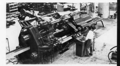
**POLISHED STEEL RAM** of this hydraulic extrusion press—one of the fastest in existence—rapidly deforms superalloys at speeds up to eight inches per second.
