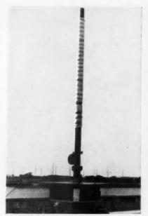
HELICAL ANTENNAS, interlaced for experiment, give good radiation patterns.
