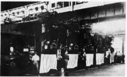
AUTOMATIC GAGE-CONTROL SYSTEM PERMITS IMPROVED ACCURACY IN ROLLING OF TIN PLATE.
