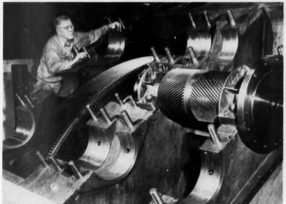
USS "SARATOGA," newest 60,000-ton aircraft carrier, develops with four cross-compound steam turbines and four double-reduction gears more shaft horsepower than any naval vessel.
