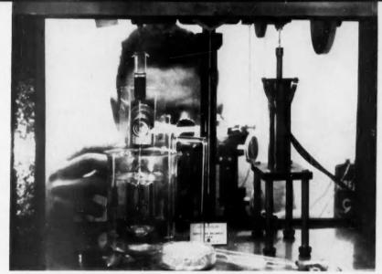
PERFECT COPPER CRYSTALS, without the usual irregularities in atomic structure, have sometimes revealed strengths almost 1000 times more than those of normal crystals.
