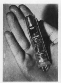
TRANSISTOR micropower audio-frequency amplifier can operate for three years.
