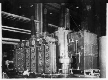
TWO FOUR-WINDING 185,000-KVA AUTOTRANSFORMERS WEIGHING 260 TONS SET SIZE RECORD
