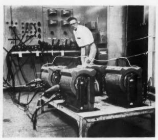
CAST COIL TRANSFORMERS OFFER SAVINGS IN SIZE AND WEIGHT.
