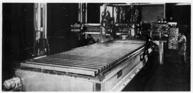
TRACER CONTROL GUIDES A CONTOUR PROFILE MACHINE THAT ACCURATELY AND ECONOMICALLY MAKES DUPLICATE SPARS FOR B52 BOMBERS.
