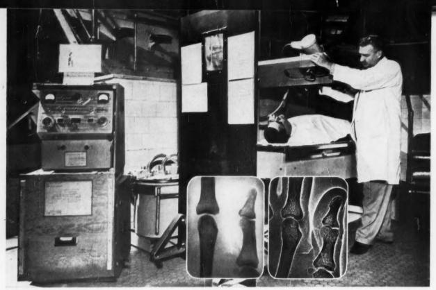
MOBILE XERORADIOGRAPHIC EQUIPMENT, using its own packing case as a support, can be set up in any building for emergency
