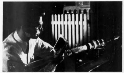
ZONE-MELTING PROCESS for production of high-purity silicon consists of successive recrystallizations of silicon as an ingot is slowly drawn through a gas-filled quartz tube.
