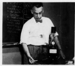
PORTABLE NUCLEI METER COUNTS MINUTE PARTICLES IN AIR SAMPLE.
