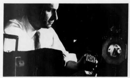
**DIRECT AMPLIFICATION** of light that is independent of electronic tubes occurs only when electroluminescence is "triggered" by light striking an experimental phosphor screen.
