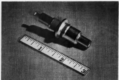
METAL-AND-CERAMIC high-frequency tube of the lighthouse line can deliver two kilowatts of peak power at 3500 megacycles and can be pulse-operated up to 4000 megacycles.
