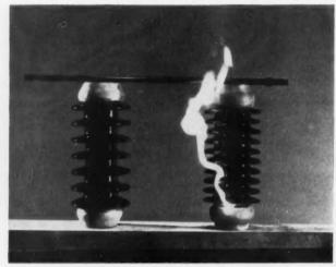
POST INSULATOR WITHSTANDS HIGH VOLTAGE IN DRY FLASHOVER TEST
