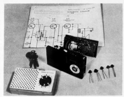
POCKET-SIZED PORTABLE RADIO, utilizing transistors instead of vacuum tubes, has unusual sensitivity and power output. A special circuit arrangement extends battery life.
