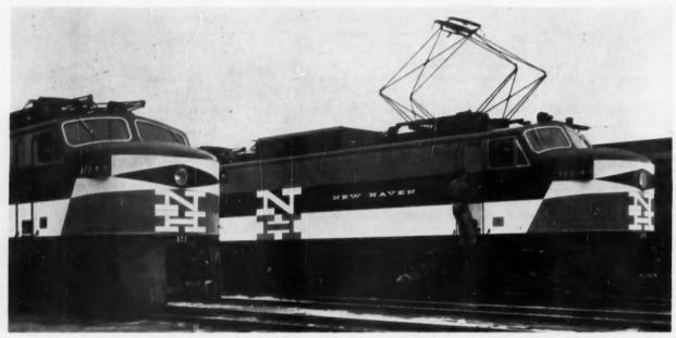
TEN STREAMLINED RECTIFIER PASSENGER LOCOMOTIVES, RATED 4000 HP, WERE DELIVERED TO THE NEW HAVEN RAILROAD IN MARCH.
