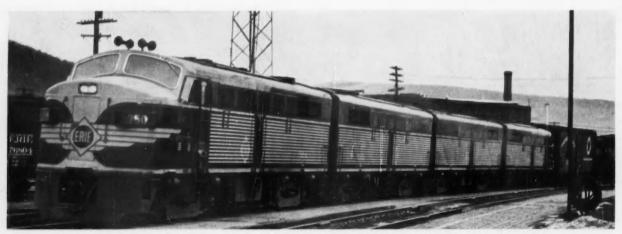
A ROLLING LABORATORY, THIS FOUR-UNIT DIESEL-ELECTRIC LOCOMOTIVE EVALUATES COMPONENTS FOR USE IN THE EXPORT TRADE.
