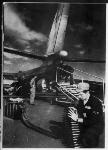
**ARMAMENT**, designed and built by General Electric, is radar controlled and gives the B47 a heavyweight punch to the rear.
