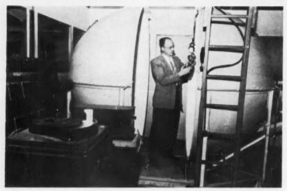
STANDARD LAMP FROM BUREAU OF STANDARDS CALIBRATES LUMINAIRE TEST LAMP.
