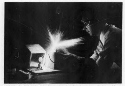
ZIRCONIUM METAL POWDER—heat-sensitive ingredient in a primer—ignites readily, resists oxidation in an oxygen atmosphere at normal temperatures, and can be handled safely.
