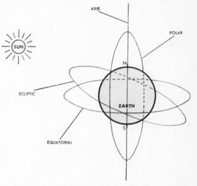
**ORBITS** of future earth satellites each possess distinct advantages. For example, on the equatorial orbit a 22,300-mile-high satellite would be stationary relative to the earth.
