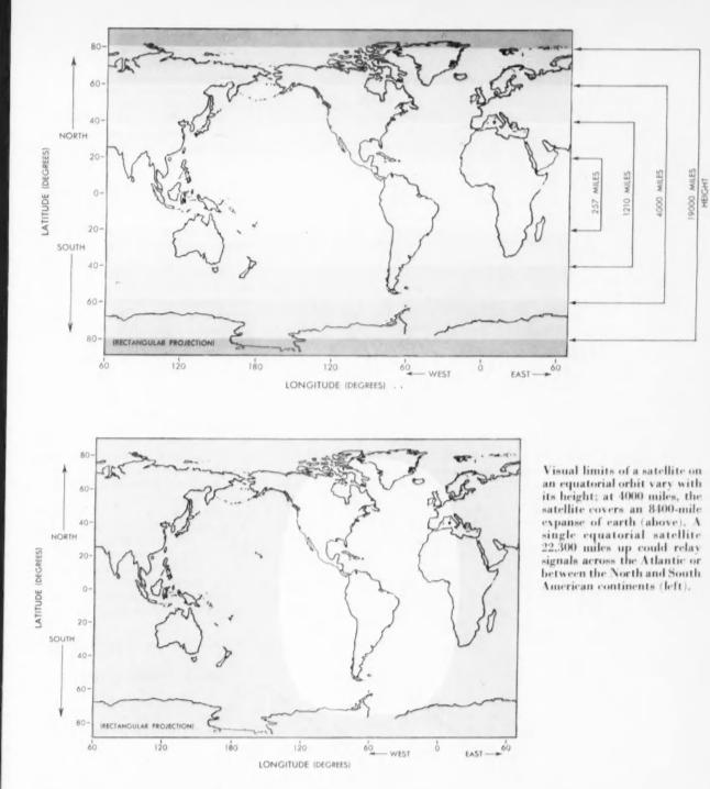
equatorial orbit vary with height (illustration, top). Arrows along the side bound the visible area north and south of the equator. At 4000 miles up, for example, the band extends from 60 degrees north to 60 degrees south latitude—a distance of 8400 miles.
