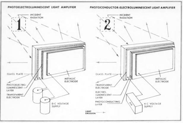
**INCIDENT RADIATION** initiates and controls light emission. Amplifier (right) utilizes two well-known solid-state elements. electrodes is almost completely different forms of energy. All these coat- then permitted to flow into the ch
