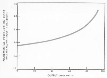
INCREMENTAL PRODUCTION COST increases with each additional megawatt of output.
