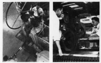
MODERN EQUIPMENT: hand-controlled rolling mill (left) and 1250-ton extrusion press.
