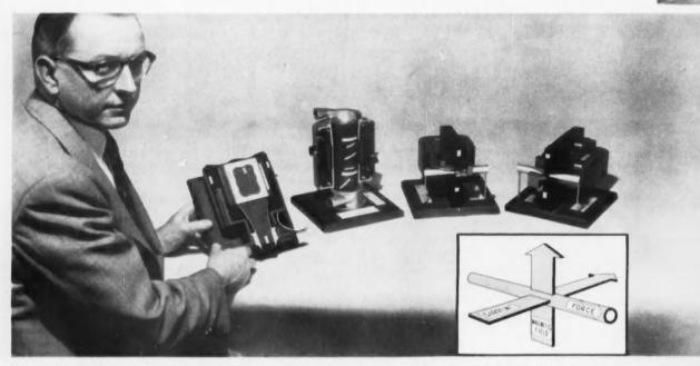
FOUR GENERAL ELECTRIC EM PUMP MODELS are shown by J. F. Cage, Manager—Component and Coolant Systems Engineering Operation, Atomic Power Equipment Department, (I. to r.): linear induction, helical flow, d-c, and a-c types. Diagram shows pumps' operating principle: Force is exerted on currentcarrying liquid in magnetic field.
