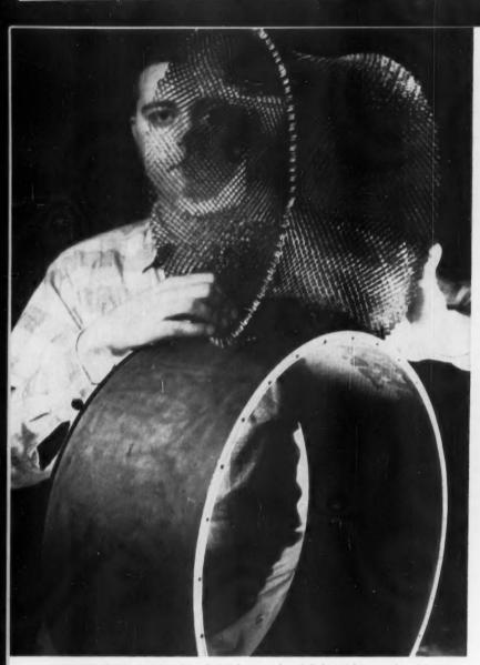
**HONEYCOMB SANDWICH** of stainless steel and lightweight core has 80 percent more strength than solid structural members. Used developmentally for casings, tailpipes, and nozzles, it also withstands high bending loads and temperatures.
