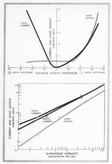
LIGHT OUTPUT AND CURRENT depend on voltage across the phosphor with constant ultraviolet irradiation (top) and on ultraviolet intensity with constant voltage (lower).
