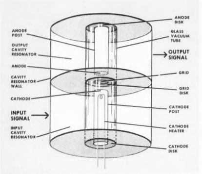
BASIC LIGHTHOUSE TUBE and forerunner of the microminiature ceramic tube was used in World War II radar. Its revolutionary concepts led to the development of the new tube.
