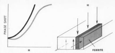
**NONRECIPROCAL EFFECTS** can also be obtained in rectangular waveguide without rotations of polarized high-frequency waves. By simple modification the ferrite isolator does the modulating job without any attendant frequency modulation.
