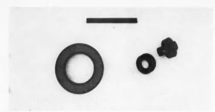
FERRITE SHAPES for electronics include simple rod, toroid, and cup cores. In television . . .
