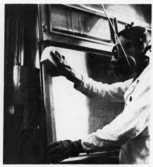
**ANALYSIS CONCLUDED,** hood is cleaned up and sponge disposed of along with other radioactive wastes. Technician wears face respirator to guard against inhaling any contaminated particles.
