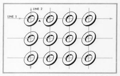
. . . with toroidal cores storing the acquired information in a binary manner. But by . . .
