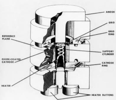
Size of a pencil eraser, the new tube offers high-gain low-noise ability to Structure Size of a pencil eraser, the new time one; and special applications.
