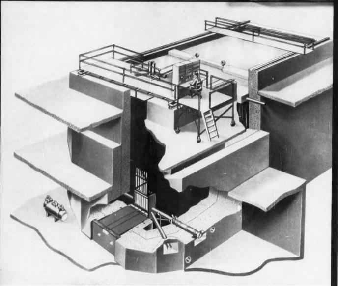
SWIMMING POOL REACTOR, one of three G-E research reactors available under the 7-point program, is designed to produce large quan-
