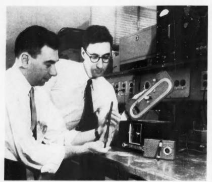
Antenna Rod Space-saving ferrite rod held by author Katz (left) sharply cuts size of today's portable radios. By contrast, author Mullen displays former loop antenna, once an essential component.
