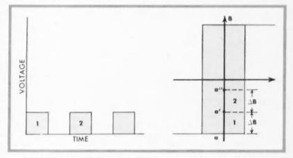
. . . applying voltage pulses, square-loop ferrites count digitally and store the count.
