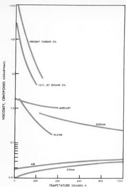
**VISCOSITY** of air and steam, unlike other lubricants, increases with temperature. Such gaseous lubricants may be feasible, but many problems remain to be solved.
