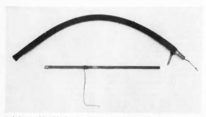
... high permeability delay lines provide more time delay per unit length than other means.
