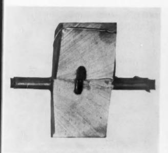
TRACKING INSULATION (RIGHT), NO CARBONIZED PATH FORMS.
