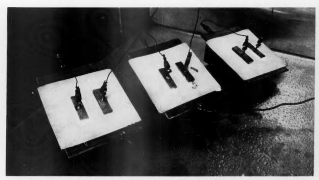
INSIDE FOG CHAMBER, NONTRACKING INSULATION COVERED WITH SYNTHETIC DUST COUNTERS THE FORMATION OF FREE CARBON.
