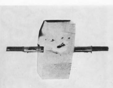
HIGH VOLTAGE APPLIED TO THE ELECTRODES CAST IN BUTYL RUBBER (CENTER) CHARS A CONDUCTING PATH BETWEEN THEM. BUT WITH NON-
