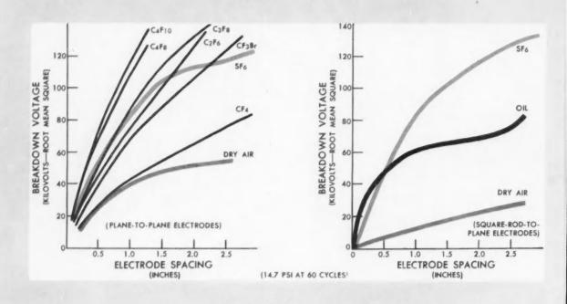
GASEOUS FLUOROCOMPOUNDS have progressed to the point where they now have a fairly high dielectric strength at moderate pressure. SULFUR-HEXAFLUORIDE SF6 GAS has a dielectric strength that competes favorably with petroleum-based oil under special conditions.
