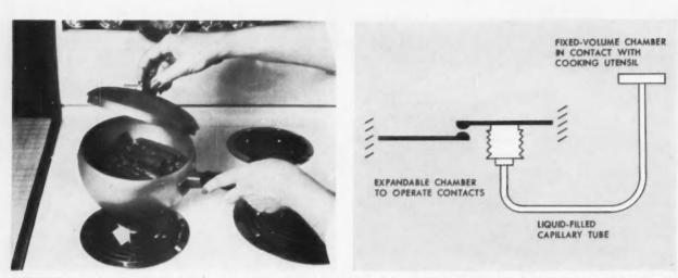
TEMPERATURE SENSITIVE DEVICE (ARROW) OPERATES ON THE PRINCIPLE THAT LIQUID VOLUME VARIES WITH TEMPERATURE CHANGE.
