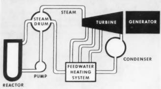
**STEAM FLOWS FROM REACTOR** to drum. Saturated steam passes to turbine; water goes to feedwater heaters and returns to steam drum. Forced circulation pump provides automatic control of response to load changes.
