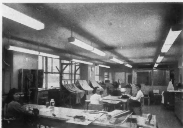
Occupational Therapy Good lighting lessens the strain and fatigue of the physically handicapped (left). Well-shielded commercial-type fixtures for shop training reduce glare and help prevent accidents.
