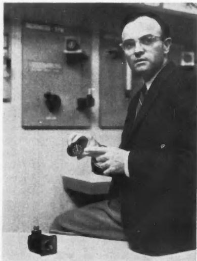
TACHOMETER for jet aircraft displayed by author Fraizer receives electric impulses from engine-mounted generator (table).
