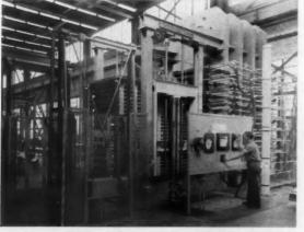
One of fifteen giant laminate presses in the Coshocton plant with capacity to meet industry requirements.
