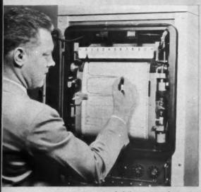
**DIRECT RECORDING** of diffraction analysis supplements film and direct-reading techniques.
