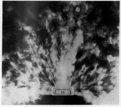
**SMOKE TEST** reveals how warm air hugs the wall closely and prevents cold air from spilling down to create drafts; floor level air drawn to register blends with the warm air.
