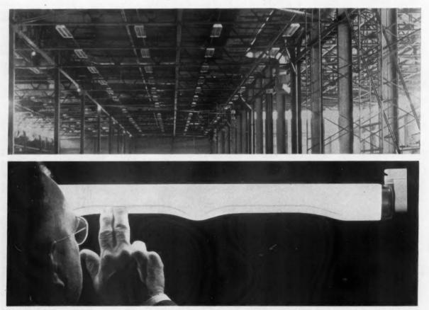
**THE GROOVES** are the reason you get twice as much light. They bring the phosphors on the inside wall of the tube closer to the ultraviolet radiation thus reducing internal light losses. You get
