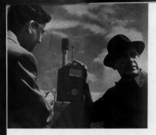
Comprising haze that overhangs industrial complex (left) are airborne particles that Van Luik and Rich (above) measure with a portable condensation nuclei meter. Engineers (right) determine erosion rate of motor-starter contacts in test chamber.
