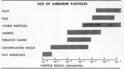
approximately 5000 particles per cubic centimeter of air. In a small industrial town, it would rise to about 50,000 per cubic centimeter. And over a superhighway or major industrial complex, the count might go as high as 500,000.
