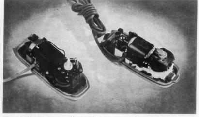
**NEW MOTOR DESIGNS**—a small universal-series unit perched on top of a die-cast aluminum chassis—resulted in both reduced dimensions and value improvements.
