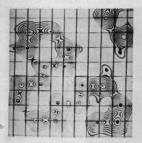
**MATHEMATICAL ANALYSIS** of diffraction results yields electron density map. Number and spacing of contour lines show kinds of atoms present. Three-dimensional crystal model (left) is based on map.
