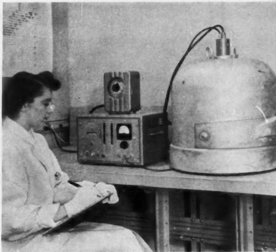
4. Placed in scintillation counter, slug's radioactivity—proportional to plastics' abrasiveness—is recorded
