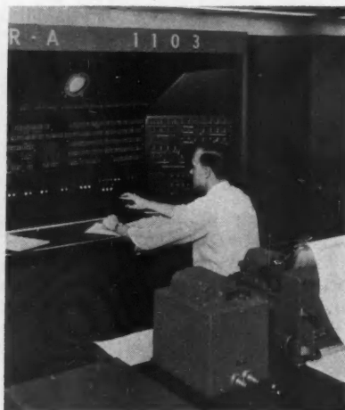
Lewis Flight Propulsion Laboratory Observers view the tests via television in supersonic-tunnel facility's main control room. Data signals from the tunnel are fed to an encoder (below) and, in turn, to a push-button-controlled computer.
