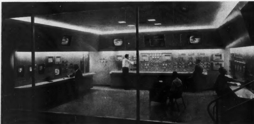
Lewis Flight Propulsion Laboratory Observers view the tests via television in supersonic-tunnel facility's main control room. Data signals from the tunnel are fed to an encoder (below) and, in turn, to a push-button-controlled computer.
