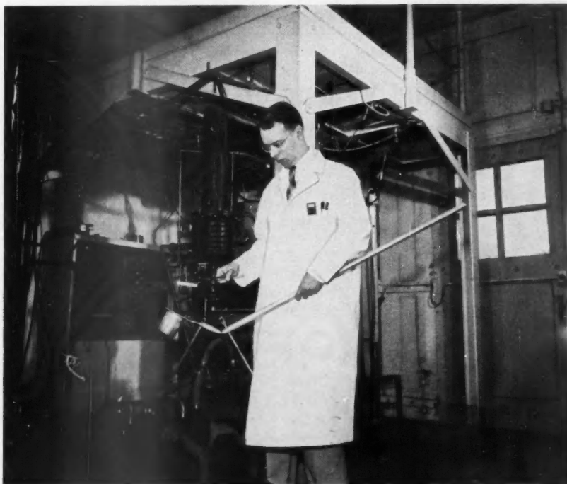
LUBRICATING-OIL SAMPLE is removed from linear accelerator by author. Bombardment by accelerator's neutrons render the oil's trace-impurities radioactive for identification.
