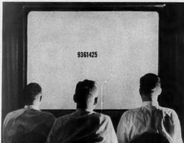
TACHISTOSCOPE —Numbers and words flashed on the screen for 1/100 second make staccato demands on nerve and muscle. Operator presses an ordinary camera cable release to operate the shutter.
