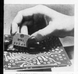
**ENCAPSULATED** resistor-capacitor network adapts to placement. resists humidity.
