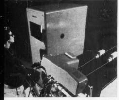
**COLOR STEREO TV** permits an operator to observe screen and direct manipulator.
