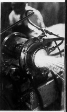
FIRST-STAGE ROCKET ENGINE powered Project Vanguard missile to an altitude of 109 miles and a top speed of 4250 mph, from Air Force Missile Test Center, Cape Canaveral, Fla.
