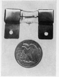
**QUARTZ LAMP** for jet aircraft has 100 percent light output until near end of its life.
