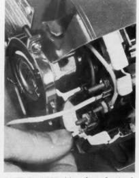
**QUICK-CONNECT** wiring tabs on fractionalhorsepower motors are economical to apply.
