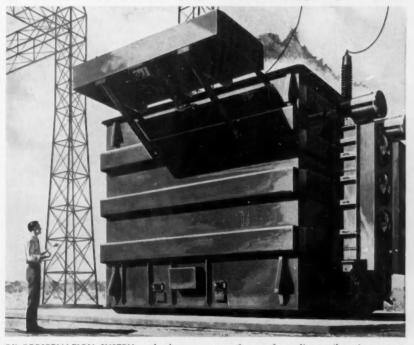
OIL-PRESERVATION SYSTEM seals the power transformer from direct oil-to-air contact.
