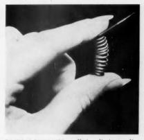
**THERMOCOUPLE'S** small size eliminates disturbances in systems under measurement.
