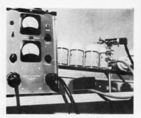
**FIXED-HEAD HALOGEN DETECTOR** facilitates automatic high-production leak testing at low cost.
