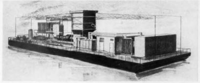
GAS-TURBINE POWER PLANT on barge operates from a central power plant on shore.
