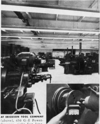
Grooves, eight feet long, mounted 10 feet high, with 10 feet between rows, maintain a lighting level of 160 footcandles economically. This means
