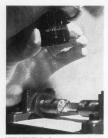
**NEW DETECTOR** of temperature resistance utilizes tungsten wire as sensing element, withstands nuclear radiation from reactor.
