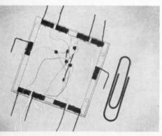
TINY CRYOTRONS may replace vacuum tubes and transistors in certain applications.
