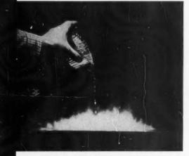
**VOLATILE LIQUID** is poured on vibrating plate during vibration-pattern studies.
