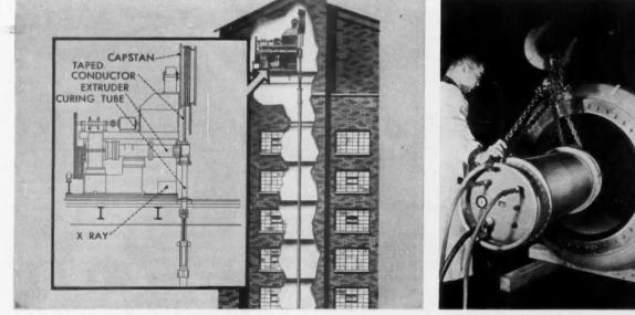
**VERTICAL DOWNWARD EXTRUSION** of high-voltage butyl-insulated cables overcomes danger of eccentricity present in horizontal manufacturing methods.
