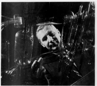
**THERMIONIC CONVERTERS**, designed in many experimental versions, have already achieved the direct conversion of more than 8 percent of the applied heat energy into electric power.
