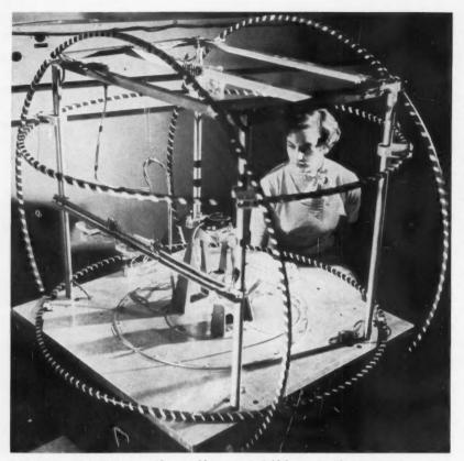
**INTRICATE EQUIPMENT** provides a stable magnetic field for testing the compass transmitter of new lightweight low-priced compass system intended for business aircraft.
