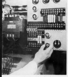
**SPEED VARIATORS** for d-c drives incorporate a newly designed static regulator.
