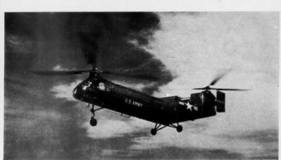
**T58 TURBOSHAFT ENGINE** powered the Vertol H21D (shown) and a modified Sikorsky S58—the first twin-engine helicopters in U.S. to be propelled by aircraft gas turbines.
