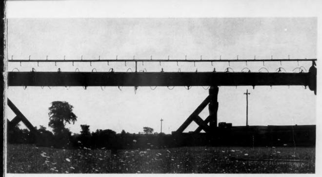
to produce a horizontal field pattern for TV broadcasting undergoes pattern tests prior to shipment to WJMR-TV in New Orleans.
