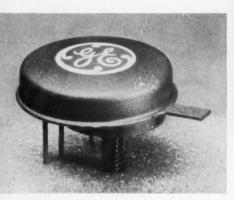
HIGH-POWER silicon transistor has a grounded emitter cutoff frequency of 400 kc.
