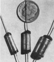
CAPACITORS, uncased and low in cost, have microfarad ratings of 0.001 to 0.1.
