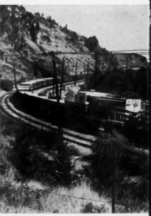
HIGHER FREIGHT-TRAIN SPEEDS in the mountainous terrain of the West will be met by 30 new 8500-hp gas-turbine electric locomotives being constructed for the Union Pacific.
