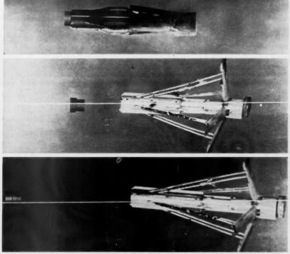
**BOOSTER UNIT** (top) for testing missile nose cone—fired from a 5-inch gun—rips through air, right to left, at Mach 2, then releases nose-cone model as air drag slows its flight.
