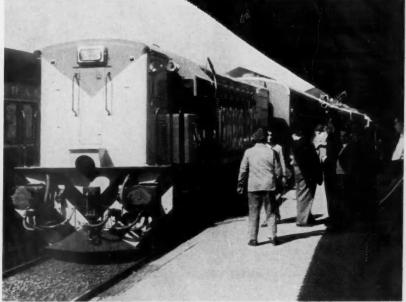
**PRODUCTION BEGAN** in 1957 on 3 sizes of the new standard export line of diesel-electric locomotives. The Chilean State Railways received the first shipment.
