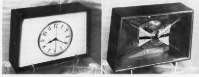
**PERMANENT-MAGNET MOTOR** obtains power from 4 ferrite rods. Flux is picked up from a 60-cycle coil concealed about a foot away. Thus this clock has no visible power supply.
