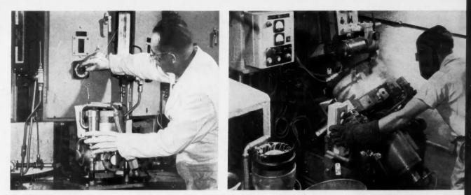
HERMETIC SEALING of compressors for new air-conditioners is carefully checked to provide air-tight operation throughout the life of the units.
