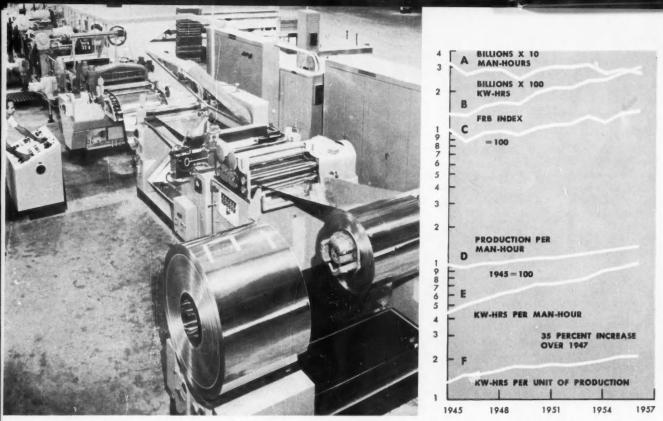
**NEW EQUIPMENT** automatically processes tin plate from coils, improving quality control and reducing manufacturing costs—an exrise in production per man-hour and use of electric power.
