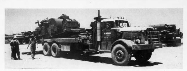
DIESEL-ELECTRIC POWERED oil-well drilling-rig drives have the advantage of excellent portability, speeding preparation cycle.
