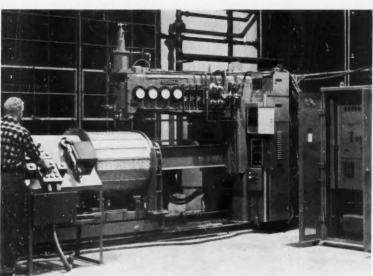
WORLD'S FIRST automatically programmed resistance-welding machine realizes new
