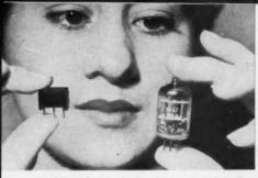
**MIDGET** double-diode selenium rectifier offers sizable savings to TV set manufacturers.
