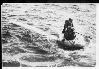
The test torpedo surfaces when spent and must be retrieved for the information recorded during its run.
