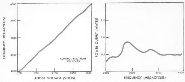
FREQUENCY set by the d-e anode voltage varies almost instantly. POWER up to 10 watts is possible through narrower tuning ranges.
