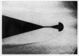
HELIUM FLOW forms shock-wave pattern around a ½-inch hemispherical model in tunnel at Mach 28.
