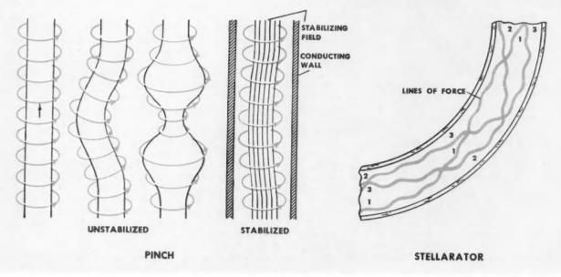
Confining Gas Plasma at stellar temperatures has been attempted with current-carrying gases that rely on the stabilized made with the recently announced stellarator and mirror devices, which use current in ex-
