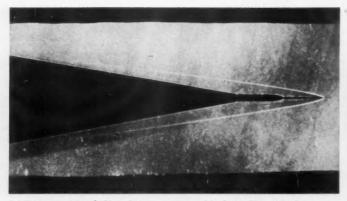
**RAZOR BLADE** is held in helium stream at Mach 22. The white line represents shock wave; the dark inside line marks the boundary layer.
