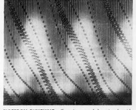
**ELECTRON BUNCHING** effect is caused by signal grid. Reflection of light from smooth surface produces shadow pattern. Slope of curve tells acceleration of "electron."
