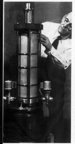
**MECHANICAL SWITCH** developed by Dr. W. F. Westendorp is used in large-scale plasma experiments; it can accurately control power in the order of 1000 megawatts.
