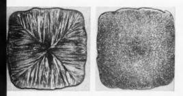
By inoculating a casting with special additives, scientists in the Research Laboratory have produced stainless steel with greatly refined grain structure (above, right) compared with characteristic columnar grain. This technique, although still experimental, resulted from a better basic understanding of how metals freeze from the melt. With E. Van Patten (center) are metallurgists James L. Walker (left) and A. J. Kiesler.
