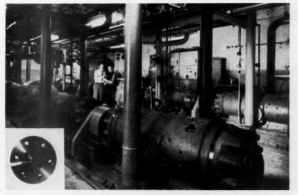
**VACUUM PUMPS** for helium tunnel fill an entire room and maintain a vacuum in the test section of the tunnel. Helium flows through a 1/10-inch orifice (inset).
