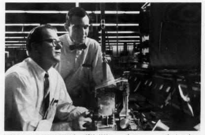
WIDE-BAND SPECTRUM TESTS from 2500-4000 megacycles are run on production voltagetunable magnetrons by G. J. Griffin, Jr. (standing) and Frank Yatsko.
