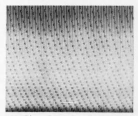
**MODEL** "electrons," constantly accelerating, roll down from cathode to anode. The visible electron tracks represent 90 exposures over a period of  $1\frac{1}{2}$  seconds.
