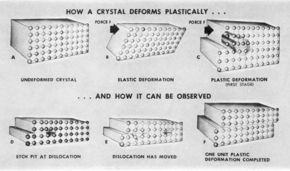
**DISLOCATION MOTION** inside a crystal permits plastic deformation. Acid easily attacks the crystal where the dislocation line intersects line as it moves through the crystal, under force.
