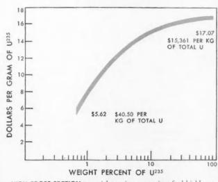
HIGH-CROSS-SECTION material requires a uranium fuel highly enriched with U-235; cost per gram varies with enrichment.
