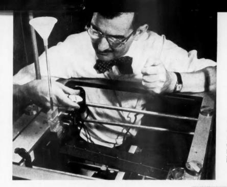
With a mechanical analog of an electron tube—the latest of a variety of mechanical models that make electrons appear larger— Dr. Andrews studies the electron's journey from cathode to anode.
