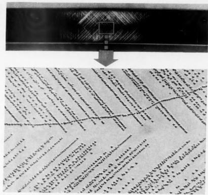
**PLASTICALLY BENT CRYSTAL** is etched in acid: one area (color inset) magnified 600 X (below) discloses long lines of etch pits that occur only in plastically deformed portion.
