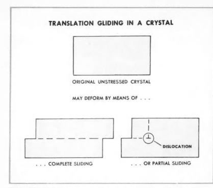
**TRANSLATION GLIDING** permits crystal deformation without destroying the crystal pattern. Partial sliding overcomes crystal resistance by moving a dislocation through the crystal.
