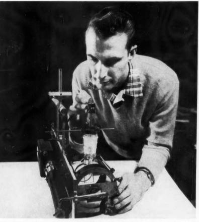
**MOV!E CAMERA**, light source, and glass cylinder attached to an aluminum supporting plate are used in a project to find out how fire burns in the absence of gravity.
