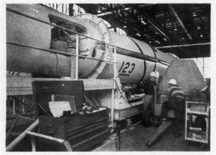
**Re-entry Vehicle** With electronic equipment to relay information back to earth during flight, re-entry vehicle (in orange handling dolly) will be installed on intermediate-range *Thor* missile.
