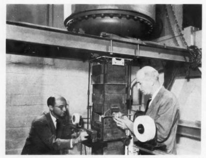
**RESEARCH SCIENTISTS** prepare experiment on polyethylene film irradiation. Lead bricks block stray beams from the million-volt electron radiation generator, situated overhead.
