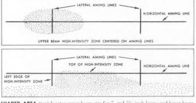
**SHADED AREA** (top) locates upper-beam aim for 7- and  $5^{3}_{4}$ -inch lamps and lower-beam aim (lower) for Type 2 ( $5^{3}_{4}$ -inch) lamps and Suburban headlights, both with left lamp.
