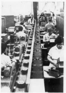
To minimize the manual handling of components, manufacturing engineers have applied mechanization to the assembly of watthour meters whereever feasible.
