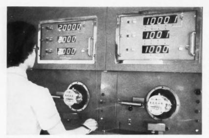
"**TOTE BOARD**" automatically rates test meter (right) against standard meter—indicating (from top) light load, 0.01 percent fast; lagging load, 0.1 percent fast; full load, perfect.
