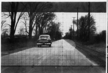
CRITICAL CORNER (shaded area) needs greatest intensity, to light objects far enough ahead for safe visibility. Superimposed grid defines elements for optimum beam design.
