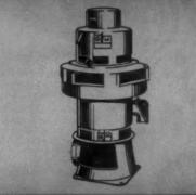
NEW VERTICAL WEATHER PROTECTED MOTOR—150 to 1000 hp—has withstood hurricane-force winds and water blasts. Windings remained completely dry.
