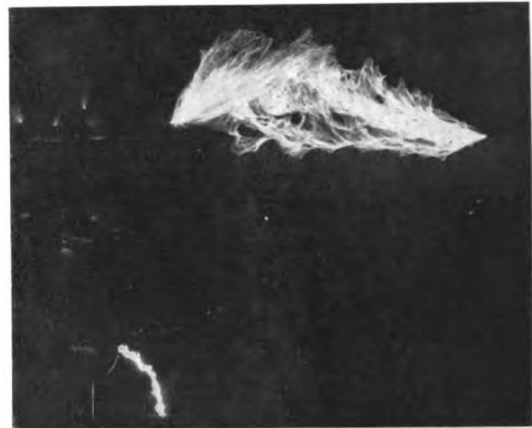
Fig. 12. The Upper Arcs, Which Occurred at the Proper Place Between the Terminal Points, are of Several Successive Discharges Across a 9-ft. Gap Between Sharp Points, and Started by a Million Volts from Line to Ground. The lower discharge took place from the cap of the main terminal to a fence in the background. This accidental arc was photographed nearly end-on and does not indicate its length of 13 feet. The two strong lines near the arc show respectively the curved outline of the cap and the straight surface of the terminal by reflection from the arc. The location of this latter arc is shown in Fig. 13 at the points marked A and a
