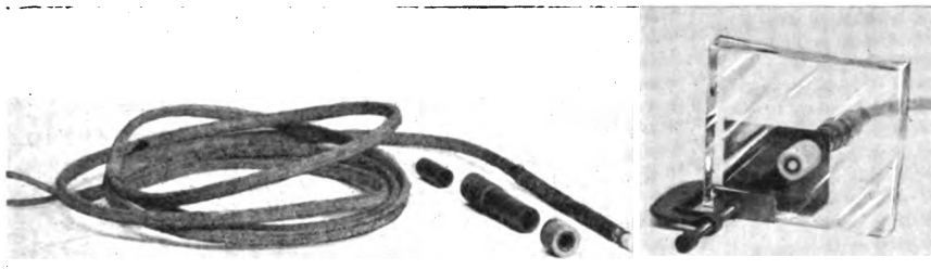
Fig. 2. Parts of the Protected Thermocouple and an Assembled Thermocouple Clamped on a Glass Plate
