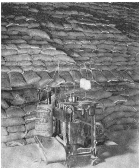
Fig. 5. Portable Motor-driven Bag Sewing Machine at Work in a Sugar Warehouse
