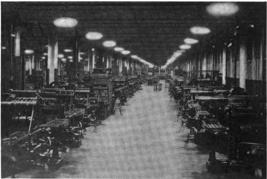
Figs. 1 and 2. The glaring local light shown in the top picture is a menace to safety and vision and is one of the evils which lighting codes are aiming to destroy. Contrast the lighting of this milling machine with the lighting of those shown in the bottom picture
