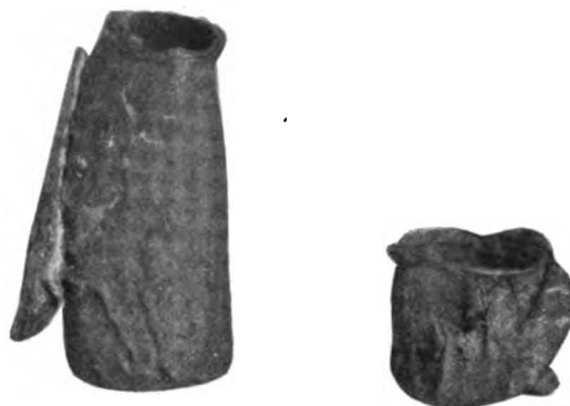
Fig. 3. Calorized Copper Tubing Heated to Its Melting Point
