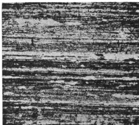
Fig. 3. Recrystallization of Severely Rolled Aluminium at 250 deg. C. Magnification 100 dia. Reduced by \frac{1}{4} . (From Recrystallization of Aluminium Sheet on Heating, by Carpenter and Elam. Jour. Inst. Metals, Vol. 25, p. 272, Plate XVIII, 1921)
