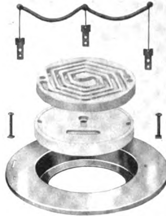
Fig. 2. Parts of Hotplate shown in Fig. 1
