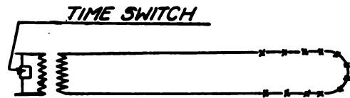
Fig. 18. Station Type Constant-current Transformer Equipment and Its Application
