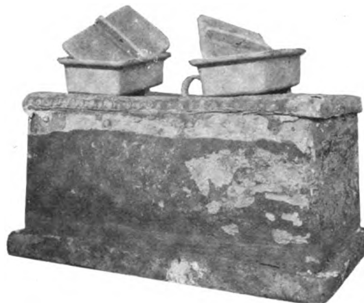
Fig. 5. Two Small Calite Annealing Boxes After 1500 Heat-Hours. Large box shows characteristic scaling of steel
