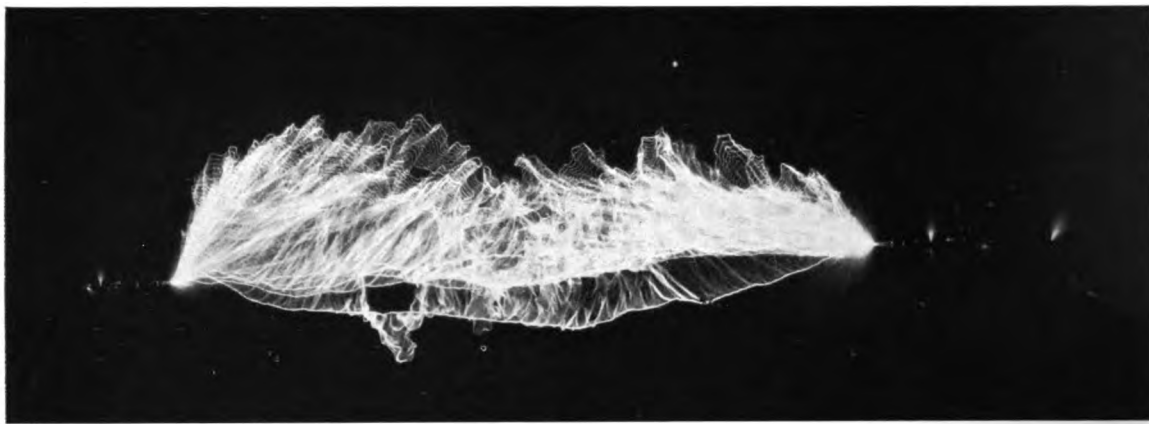
Fig. 14. Several Successive 1,200,000-volt Arcs Between Points Spaced 11 Ft. Apart
