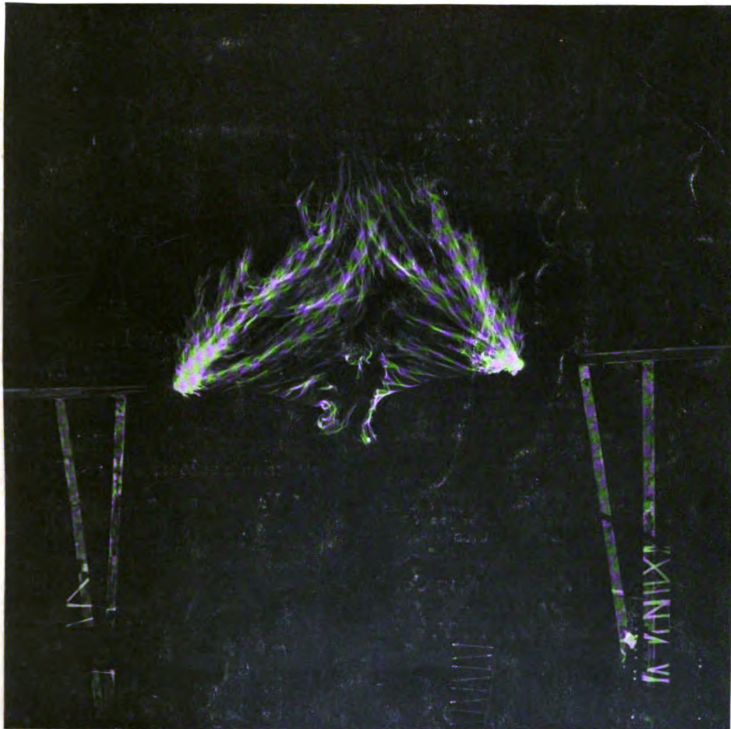
SPARK-OVER AT ONE MILLION VOLTS BETWEEN NEEDLE POINTS ABOUT NINE FEET APART (See article, page 111)
