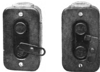
Fig. 6. Push-button Station for Starting and Stopping. The motors are equipped with remote control. A latch can be carried over the stop button and this latch held in place with a padlock. When this lock is in place the feed circuit is open and the equipment cannot be operated from this or any other station
