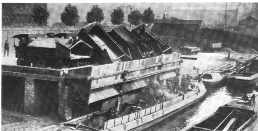
Fig. 2. Orwell Electrics Belonging to the Willesden Urban District Council Dumping House Refuse into Barges
