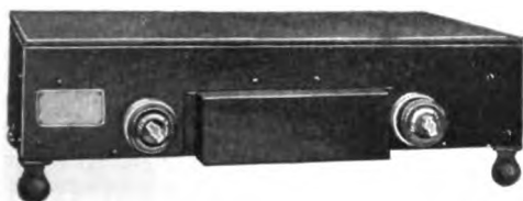
Fig. 11. 18 by 36-in., 6-kw. Electric Griddle. The heating unit is divided into a right and a left-hand section, each controlled by a separate three-heat switch and protected by individual cutouts mounted at the front of the device in a readily accessible box
