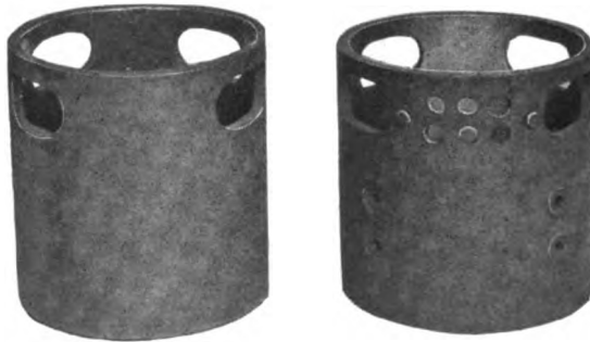
Fig. 4. Magnet Frame Constructed from Steel Plate
