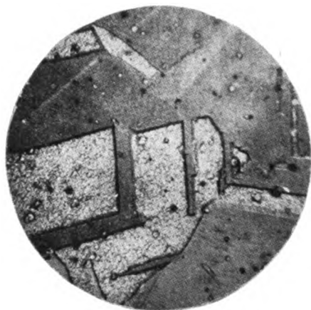
Fig. 1. Photomicrograph of Ordinary Copper. 75 times magnification
