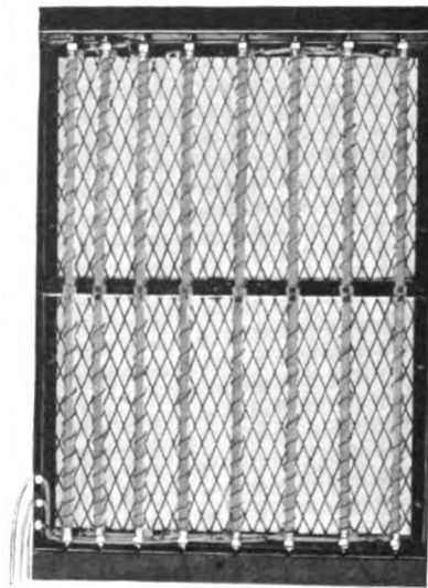
Fig. 3. Heating Unit of the Type of Bake Oven in Fig. 4, Showing the Large Amount of Heating Wire Used and the Method of Distributing the Heat Over the Entire Area
