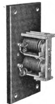
Fig. 45. Voltage Drop Relay
