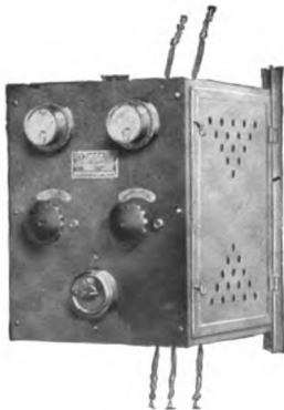
Twenty battery Tungar—capacity one to ten 6-volt batteries at 12 amperes or less, or one to twenty 6-volt batteries at 6 amperes, or less.
