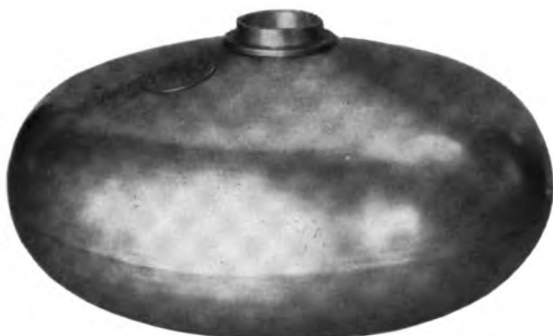
Fig. 9. Spun Brass Cap, 50-in. Dia., Used at the Top of the High-voltage Terminals, Figs. 7 and 8, to Prevent Corona Formation
