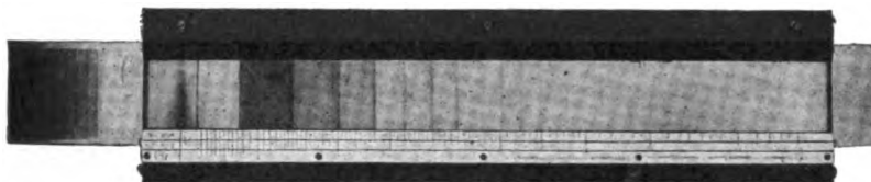
Fig. 7. Diffraction Pattern of NaCl on Scale, Ready for Measurement
