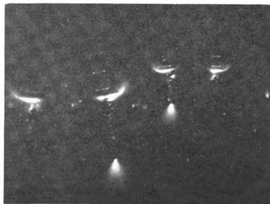
Fig. 21. Automatic Shielding by Corona (See Fig. 23)
