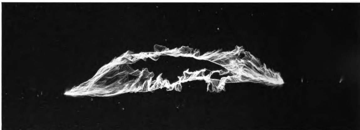
Fig. 15. Two Successive 1,200,000-volt Arcs Between Points Spaced 11 Ft. Apart
