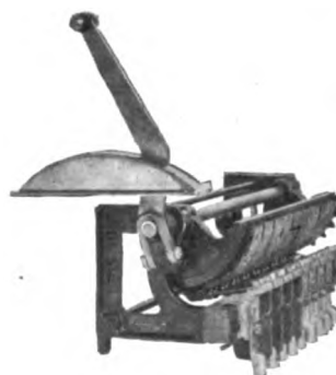
Fig. 8. Assembly of Standard Direct-operated Controller
