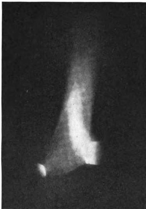
Fig. 1. High-intensity Arc at 72 Amp., 61 Volts, 18-mm. Length. Negative axis at 14 deg. 30 min.
