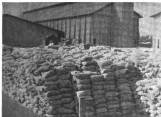
Fig. 4. The Effectiveness of the Cottrell Precipitator is Graphically Illustrated by This Photograph of a Five Days' Catch of Dust at the Plant Shown in Fig. 3
