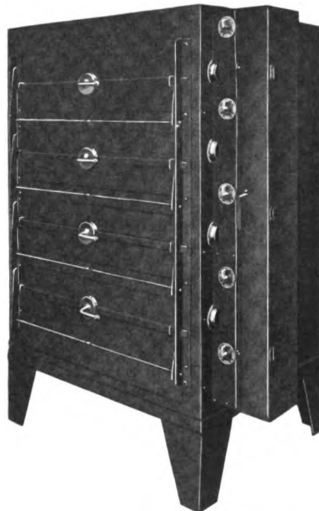
Fig. 4. Four-compartment 11-kw. Electric Bake Oven Having Four Tile Decks with Heating Unit Below Each Deck and One in the Top of the Upper Compartment. Each unit is controlled by a separate three-heat switch and is protected by an individual cutout
