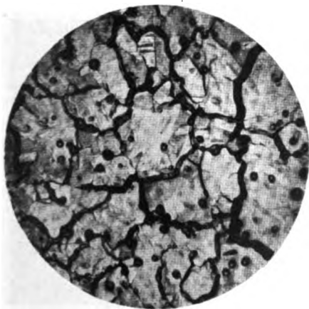
Fig. 2. Ordinary Copper Annealed in Hydrogen for Two Hours at 850 Deg. C. 200 times magnification
