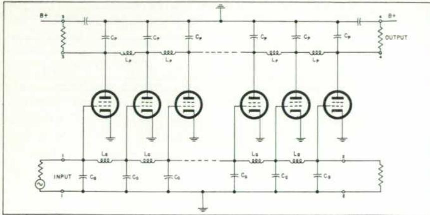
Figure 2. Basic Circuit of Distributed Amplifier
