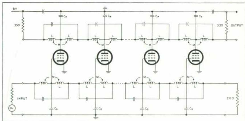
Figure 3. Basic Amplifier Circuit Using Bridged-T Lines
