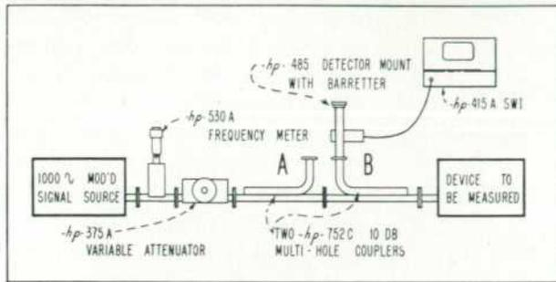
Fig. 3. Equipment arrangement for measuring reflection coefficient.
