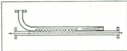
Fig. 2. Cross-sectional drawing of *-bp-* multi-hole coupler.
