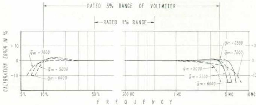
Fig. 2. Effect on vohmeter reading of variation in  $G_m$  in all tubes of Model 400H amplifier. Center  $G_m$  value for tubes used is 6200 micromhos.
