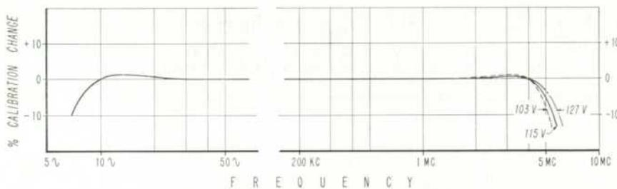
Fig. 3. Effect on vohmeter reading of  $\pm 10\%$  line voltage variation.
