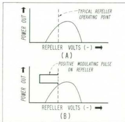
Fig. 4. (a) Typical power output vs. repeller voltage characteristic of klystron used in *-bp-* microwave generators. (b) Positive modulating pulse applied to repeller circuit pulses klystron out of oscillation.
