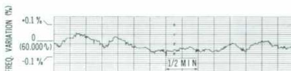
Fig. 2. (a) Curve of accuracy of power line frequency made by operating strip recorder from analog output of the new *hp* 560A Digital Recorder which operated from *hp* 524B counter (measuring 10-period averages). (b) at right shows section of printed tape corresponding to part of plotted curve ( $\frac{1}{3}$  actual size).
