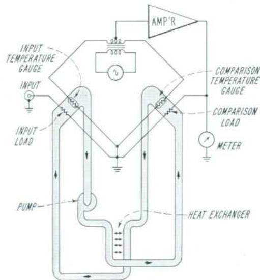
Fig. 2. Basic circuit and oil stream arrangement of Power Meter. Parallel-flow heat exchanger is located physically close to load resistors to bring oil streams entering the two load-gauge regions to same temperature. Arrangement also includes heat radiators (not shown) down-stream from gauge resistors to dissipate heat transferred from load resistors.
