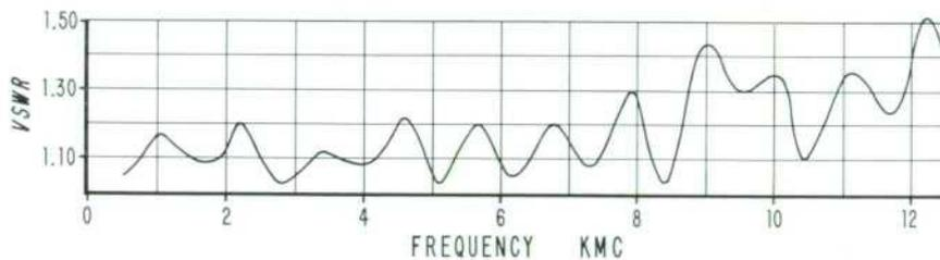
Fig. 5. Typical VSWR characteristic of Power Meter.
