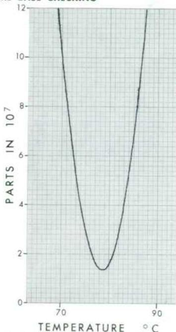
Typical crystal temperature characteristic automatically plotted with equipment shown on page 5.
