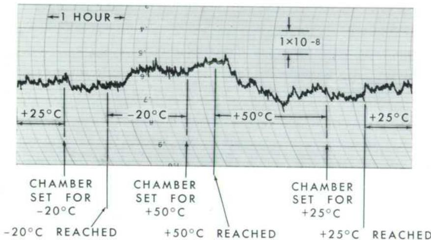
Fig. 10. Record of time-base oscillator stability as complete frequency counter was temperature-cycled in chamber which reached  $-20^{\circ}$  and  $+50^{\circ}$  C.
