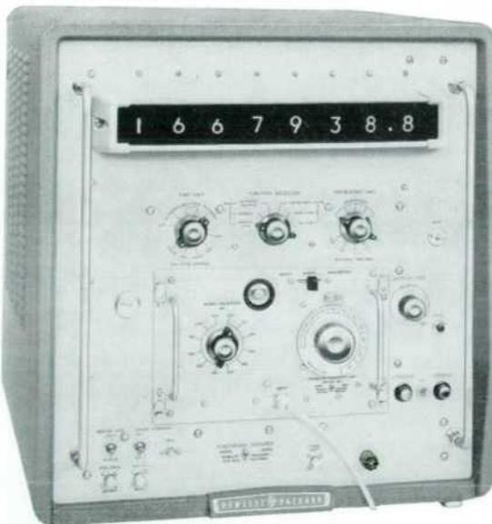
The *-hp-* 10-megacycle counter with the advanced time base described in the accompanying article has the model number 524D. In addition to its new time base this instrument also has a full 8-decade readout as shown on front page. In other respects, the instrument is the same as the well-known Model 524B.
