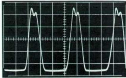
Fig. 3. Same plate current as in Fig. 2 but with capacitive component bucked out using technique indicated in Fig. 4 and described in text.
