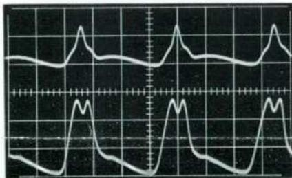
Fig. 2. Oscilloscope showing screen current (upper trace) and plate current (lower trace) of same tube as in Fig. 1 measured using two 456A current probes with dual-channel oscilloscope. Upper trace has twice the sensitivity of lower trace.
