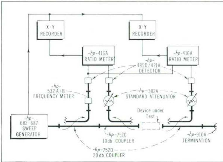
Fig. 7. Equipment set-up for simultaneously measuring reflection and attenuation of component under test.
