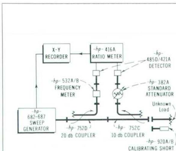
Fig. 1. Improved microwave equipment set-up for making swept-frequency measurements of reflection coefficient. Use of precision attenuator in reflection arm enables a calibrated grid to be established for desired range of reflection coefficient. Use of attenuator in this way gives higher calibration accuracy than calibrating by using a known reflection to terminate main line.
