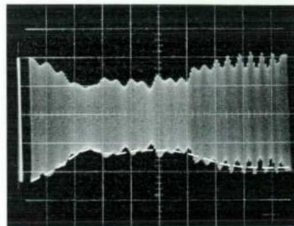
Fig. 13. A typical calibration obtained with set-up of Fig. 12 for a load reflection coefficient of 0.1. Fast ripples are from multiple system reflections and should be averaged out on both upper and lower edges of trace. For clarity typical averaging is shown only along lower edge of trace by white dashed line.
