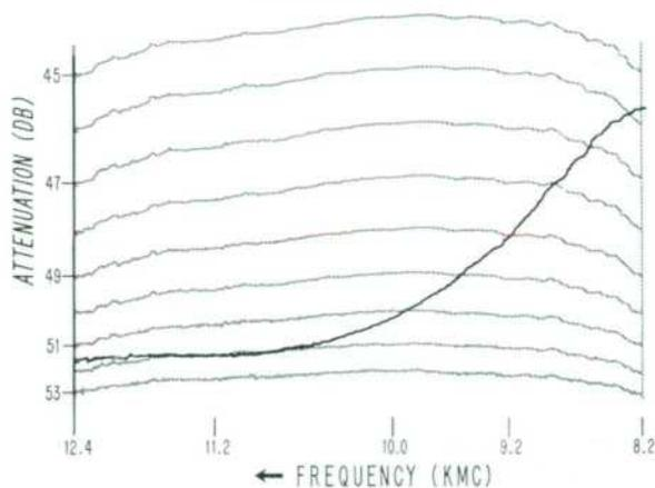
Fig. 6. Measurement of attenuation made using set-up of Fig. 5. Measurement made of non-*hp*-attenuator measured in Fig. 2 with dial now set for 50 db. As in Fig. 2, measurement can be recorded on transparent paper so that one calibration grid can serve for many measurements.
