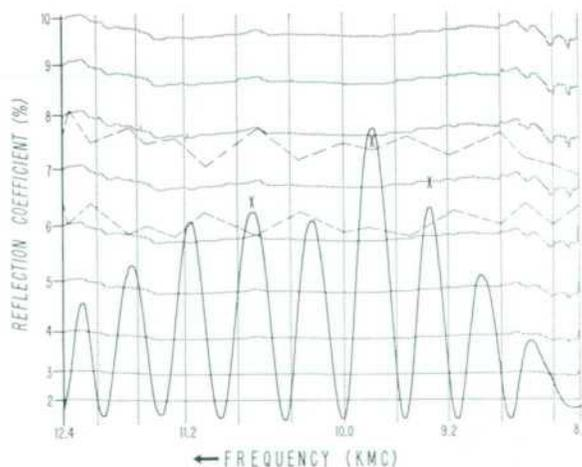
Fig. 2. Typical swept-frequency reflection-coefficient measurement made using set-up of Fig. 1. Measurement can be recorded on transparent paper so that calibration grid, once made, can serve as an underlay for many measurements. Dashed lines between 6 and 8% show error limits of measuring system for a true 7% reflection coefficient, the go-no go value in this case. X's show true value of three largest reflections as measured by single-frequency set-up of Fig. 4.
