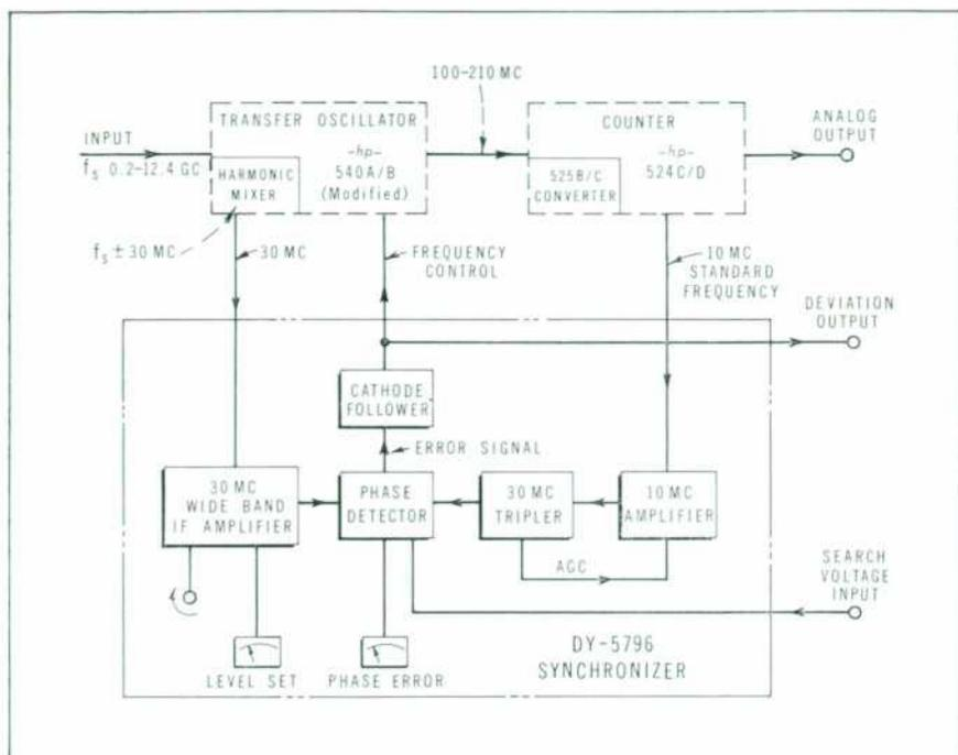
Fig. 6. Detailed block diagram of Dymec 5796 Synchronizer.
