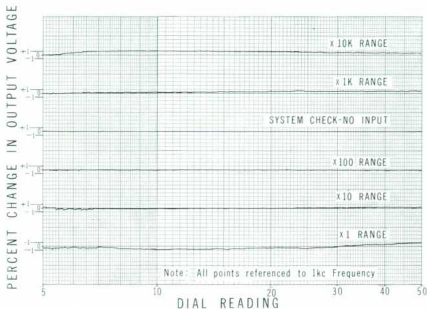
Fig. 5. Effectiveness of amplitude control circuit as shown by typical frequency response characteristic of Model 204B. Each minor vertical division has value of 1% so overall response is within about  $\pm 1\%$ .
