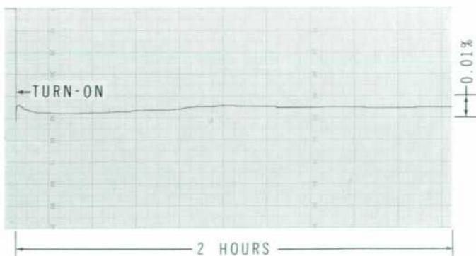
Fig. 2. Typical frequency-stability characteristic of Model 204B Oscillator. Frequency drift was only about 1 part in 20,000 in complete test including turn-on drift. Instrument begins to operate almost immediately after turn-on.
