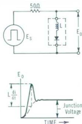
Fig. 6(b). Explanatory drawing for Fig. 6(a).
