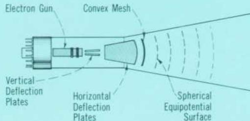
Curved mesh in new CRT terminates post-accelerating voltage lines of force; resulting equipotential surfaces are spherical.
