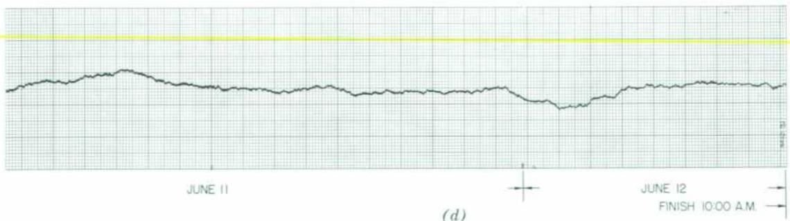
measure the stability of the two driving standards. No effort was made to synchronize the standards. While short-term fluctuations of a
