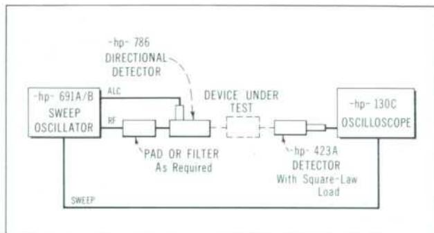
Fig. 8. Measurement set-up for supplying power in swept frequency measurements. Model 786D Directional Detector senses RF voltage level and supplies corresponding dc voltage to ALC input of sweep generator. Even with a load SWR of 2, power variations at main arm output of detector are less than  $\pm 0.5$  db.
