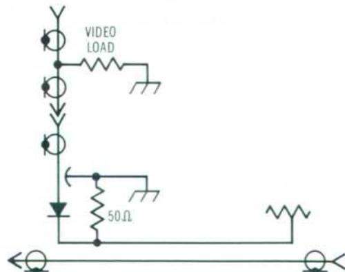
Fig. 7. Model 786D Directional Detector and equivalent schematic. Diode detector is in sealed capsule easily replaced without special tools.
