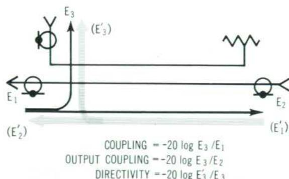
Fig. 4. Definitions of coupling, output coupling, and directivity.  $E_1$  is input voltage,  $E_2$  is voltage out of main arm, and  $E_3$  is voltage out of auxiliary arm.  $E'_1$  and  $E'_2$  are voltages out of input and auxiliary arms respectively with voltage  $E_1$  applied in reverse direction to main arm output. In all specifications, matched loads are considered to be connected to outputs.
