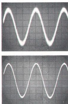
Fig. 4. Bandwidth filter improves resolution of low-level, low-frequency waveforms. Photo of 500-Hz sine wave at top was made on  $50\text{-}\mu\text{V/cm}$  range with full bandwidth (300 kHz at  $50 \mu\text{V/cm}$ ). Lower photo is of same waveform with bandwidth cut off at 5 kHz.
