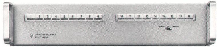
Fig. 6. Companion Programmer stores 18 programs for control of oscilloscope. Each program, selected by one pushbutton or one external contact closure, sets six oscilloscope functions. Programmers may be cascaded to provide greater number of programs.
