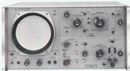
Fig. 1. New *-hp-* Model 1407A Differential Amplifier Plug-in (in lower plug-in compartment) works with either Model 140A General Purpose Oscilloscope or Model 141A Variable Persistence Oscilloscope. DC stabilization of plug-in amplifier eliminates drift problems, enabling use of dc coupling with deflection factors as low as 50  $\mu\text{V}/\text{cm}$ . Plug-in has upper frequency limit of 400 kHz.
