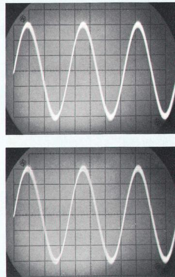
Fig. 2. Oscillograms, made with Differential Amplifier plug-in operating while dc-coupled on most sensitive range (50  $\mu\text{V}/\text{cm}$ ), demonstrate absence of drift over extended periods. Time elapsed between first and second oscillograms was 65 hours but there is no discernible drift in dc level of CRT trace.
