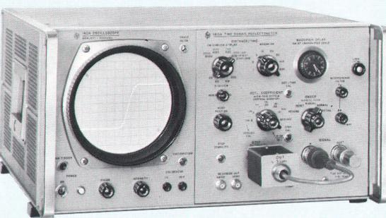
Fig. 2. Rise time converter is placed between *STEP OUTPUT* and *SIGNAL IN* connectors of *-hp-* TDR system, which consists of Model 1415A TDR Plug-in for Model 140A Oscilloscope.
