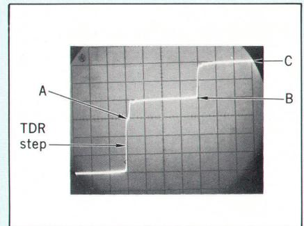
Fig. 3. Oscillogram of TDR display for test setup of Fig. 2, with cable open-circuited ( $Z_L = \infty$ ). Initial reflection at 'A' is due to impedance mismatch between 50-ohm TDR system and 100 ohms of adapter plus cable. Level 'B' is new reference level for 75-ohm measurements (reflection coefficient  $\rho = 0$ ). Level 'C' is open-circuit level ( $\rho = 1$ ).
