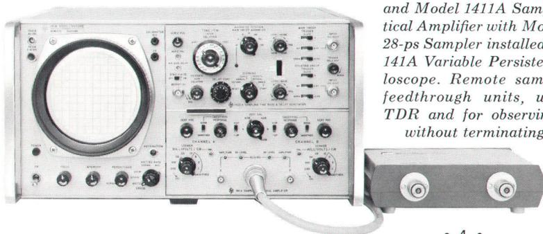
Fig. 5. Model 1425A Sampling Time Base and Delay Generator and Model 1411A Sampling Vertical Amplifier with Model 1430A 28-ps Sampler installed in Model 141A Variable Persistence Oscilloscope. Remote samplers are feedthrough units, useful for TDR and for observing signals without terminating them.
