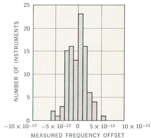
Fig. 4. (above). *Intrinsic reproducibility of portable cesium-beam standard is shown by results of comparisons of 100 independently aligned portable standards with *-hp-* house standards. All units produced same frequency within  $\pm 6$  parts in  $10^{12}$ .*
