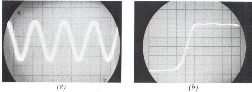
Fig. 1. Oscillograms of signals at frequencies never before viewed with oscilloscopes. (a). 18-gigahertz ( $18 \times 10^9$  cps) sine wave. (b). Step with 20-picosecond ( $20 \times 10^{-12}$ s) rise time. Rise time of step response is about 30 ps, indicating that oscilloscope bandwidth is considerably greater than 12.4 GHz. Oscillograms were made using new sampling plug-ins discussed in text. (a) Vertical: 100 mV/cm, Horizontal: 20 ps/cm. (b) Vertical: 50 mV/cm, Horizontal: 20 ps/cm.
