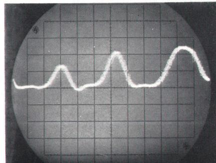
Fig. 2. Oscillogram taken with 40-ps TDR system showing reflections from short length of line with three discontinuities. TDR system can resolve discontinuities spaced as closely as  $\frac{1}{4}$  in. apart.
