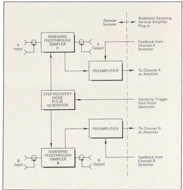
than 1.8 at 12.4 GHz, but has 5% to 10% more overshoot in the pulse response. The third sampler is a 4-GHz, 90-ps unit for applications where the widest bandwidths are not needed and lower cost is attractive. A five-foot cable (10-foot cable optional) connects the plug-in and the sampler so that measurements can be made at remote locations. Input signals are not terminated by the feedthrough samplers, so time domain reflectometry and signal monitoring are straightforward.
