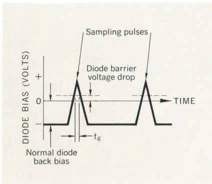
Fig. 3. Gate time  $t_g$  is time for which impedance of diodes is low in circuit of Fig. 2. Gate time is inversely proportional to bandwidth of sampling circuit. Note that gate time can be less than rise time of sampling pulse. In wideband sampling device,  $t_g$  is less than 28 ps, equivalent to bandwidth of more than 12.4 GHz.
