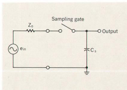
Fig. 1. Idealized sampling circuit. System to be sampled is represented by voltage  $e_{in}$  and impedance  $Z_0$ . Sample is taken by closing gate for short period, allowing sampling capacitor  $C_s$  to charge to fraction of  $e_{in}$ . Sample is stored on  $C_s$  when gate is opened.
