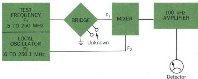
Fig. 7. Basic circuit of the *-hp-* Model 250A RX Meter is essentially a refined Schering bridge with an oscillator, detector, amplifier, null detector and power supply. When the bridge circuit is balanced in both amplitude and phase, no 100 kHz signal is produced.
