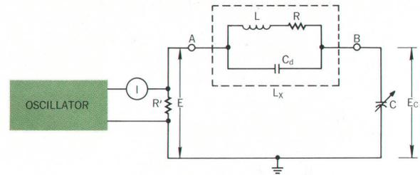
Fig. 11. In the Q meter, a known current  $I$  is passed through resistance  $R'$  which introduces the voltage  $E$  in series with the unknown  $L_x$ . The circuit under test is tuned to resonance with the oscillator frequency, and the voltage  $E_c$  is read. Then  $Q = \frac{E_c}{E}$ . In a series resonant circuit, the voltage appearing across either reactance is equal to the voltage induced in the circuit multiplied by the circuit Q.
