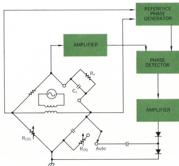
Fig. 9. The value of the  $R_{DQ}$  resistor is controlled automatically by a phase detector which responds to the phase relationship between the bridge output and a reference phase. This feedback method adjusts one bridge element automatically.
