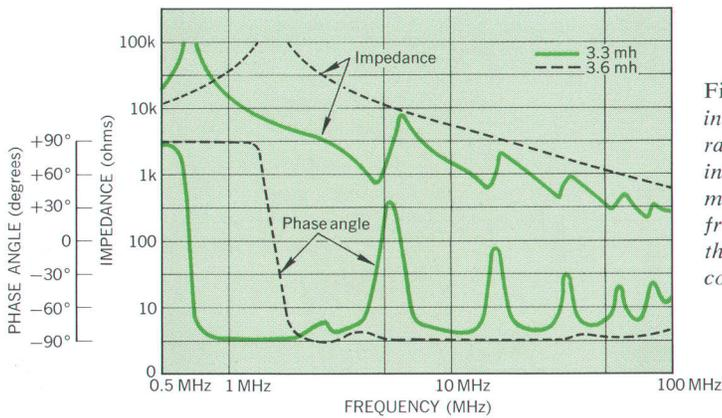
Fig. 1. Two chokes of nearly equal inductance behave differently over a range of frequencies due to differences in construction. Only impedance measurements over a wide range of frequencies will determine accurately the characteristics of circuit components.
