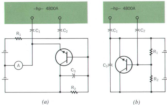
Fig. 11. Using an appropriate biasing scheme (a) it is possible to measure  $h_{ib}$  (small signal input impedance) of a transistor. By reconnecting the circuit (b) the instrument will measure  $h_{ie}$ .  $C_1$  and  $C_2$  are dc blocking capacitors, and  $R_1$  and  $R_2$  are bias resistors.
