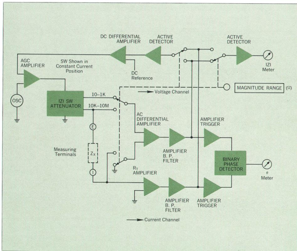
Fig. 2. In the *-hp-* Model 4800A, the unknown impedance is in the feedback loop of the trans-resistance ( $R_T$ ) amplifier. The  $R_T$  amplifier is designed to be very broadband, critically damped with extremely critical phase-gain relationships so that unknowns with wide variations in phase angle and amplitude may be placed in the feedback loop without causing oscillation or instability in the amplifier.
