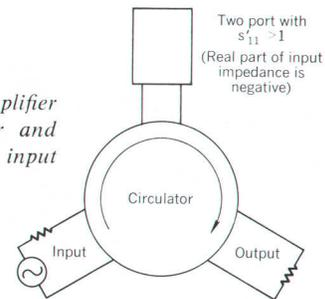
Fig. 11. Reflection amplifier consists of circulator and transistor with negative input resistance.
