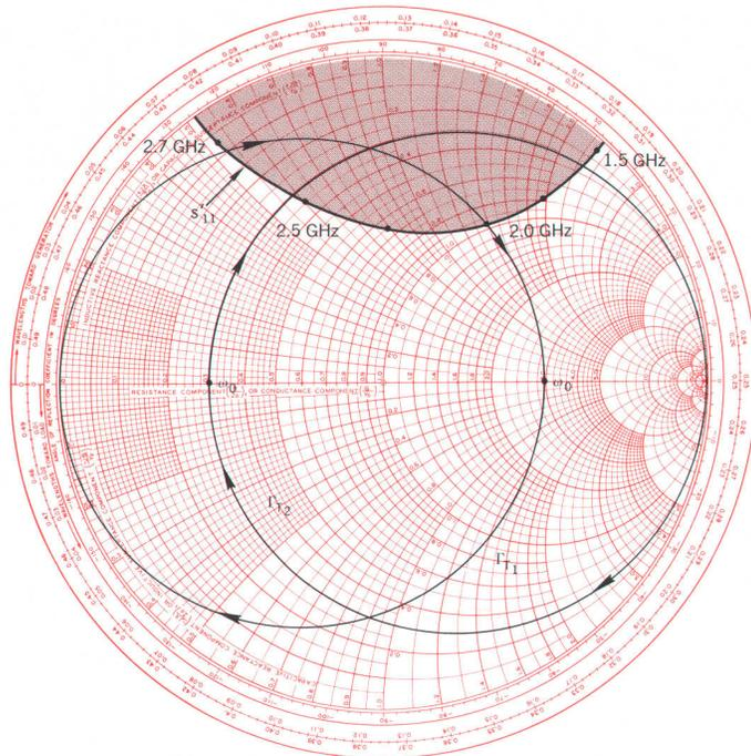
Fig. 13. Smith Chart for transistor oscillator design example.
