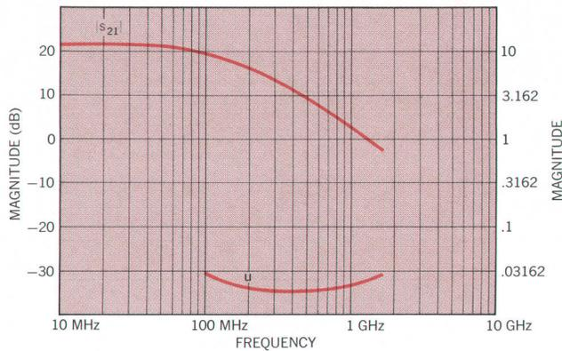
Fig. 5. Top curve:  $|s_{21}|$  from Fig. 4 replotted on logarithmic frequency scale. Data below 100 MHz measured with  $-hp-8405A$  Vector Voltmeter. Bottom curve: unilateral figure of merit, calculated from  $s$  parameters (see text).
