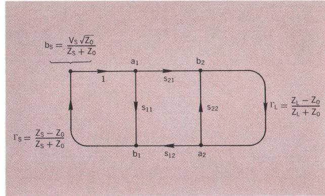
Fig. 3. Flow graph of network of Fig. 2.
