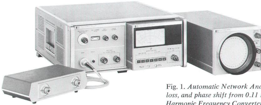
Fig. 1. Automatic Network Analyzer for measuring complex impedances, gain, loss, and phase shift from 0.11 to 12.4 GHz consists of (l. to r.), Model 8411A Harmonic Frequency Converter, Model 8410A Main Frame, and a plug-in display module (either Model 8413A Phase-Gain Indicator or Model 8414A Polar Display). Network Analyzer makes swept or single-frequency measurements. See Fig. 8 for other system components.
