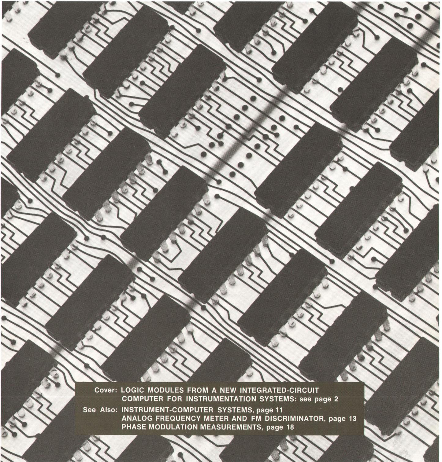
Cover: LOGIC MODULES FROM A NEW INTEGRATED-CIRCUIT
