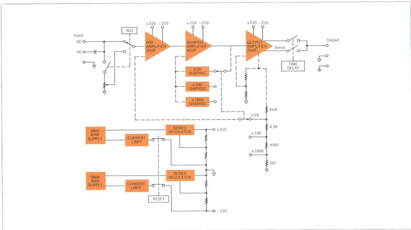
Fig. 2. Fixed gains in the *-hp-* Model 463A are selected by changing amplifier feedback characteristics by means of a precision feedback attenuator. The attenuator is made up of wire-wound resistors designed for good high-frequency characteristics, low temperature coefficient and good long-term stability.
