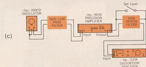
fier. To measure the output distortion, the output signal is fed first into a 1 kHz notch filter. By utilizing this notch filter to reject the fundamental signal, we can increase the sensitivity of the Distortion Analyzer because of the level of the output signal of the amplifier. This method allows measurement of distortion 85 dB down below the fundamental.
