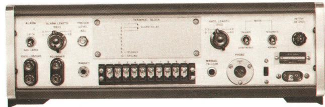
*Logic and automatic alarm circuits are built into new ac-powered Model 4950A Ultrasonic Translator for automated ultrasonic production testing. Instrument responds either to ultrasonic signal or to its integral, and closes a relay whenever signal or integral exceeds level set with input attenuator.*
