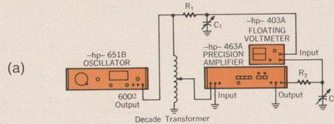
used has terminal linearity specified at  $\pm 1/2$  ppm at 1 kHz. By adjusting this decade transformer for a null reading on the null indicator (-hp- 403A) in conjunction with the phase shift compensators of R1, C1 or R2, C2, the gain of the amplifier can be read accurately from the ratio indicated on the decade transformer.
